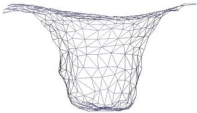
FIG 16F. PLAN VIEW SHOWING 3D MESHES OF PERFORATIONS WITH (A) CIRCULAR AND (B) ROUNDED POLYGON SHAPE. 'INSIDE-OUT' VIEW OF MESHES OF (C) FUNNEL AND (D) 'INVERTED-MUSHROOM' PROFILES. CROSS-SECTIONED WIREFRAME MODEL OF (E) FUNNEL AND (F) 'INVERTED-MUSHROOM' PROFILES. IMAGES BY ANDREW FITCHES
