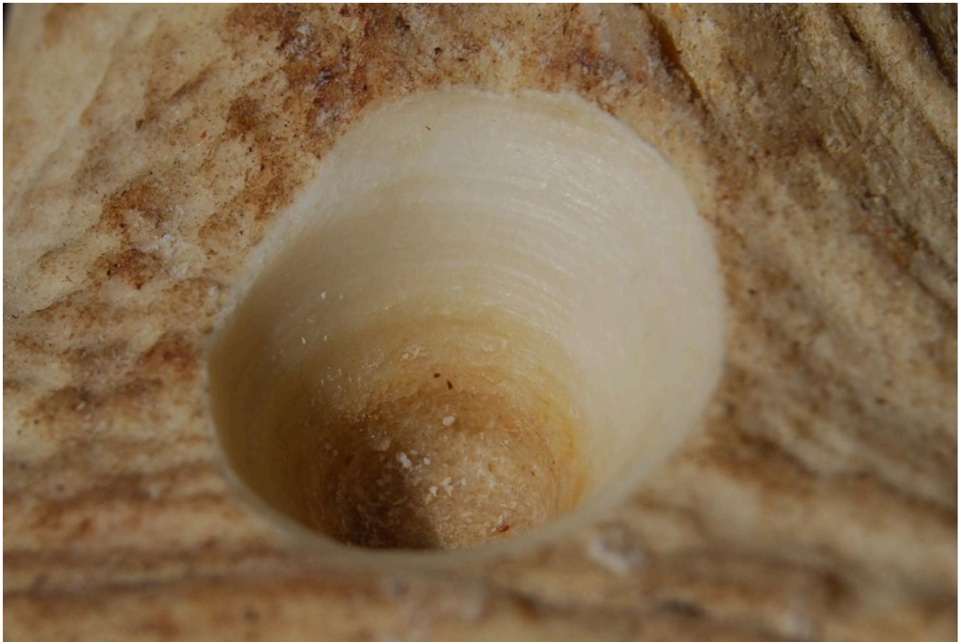
FIG 10A. STRIATIONS PRODUCED BY BOW DRILLING ON (A) SOAKED ANTLER AND (B) DRY ANTLER, AND (C) REPRESENTED IN A SCHEMATIC DRAWING. PHOTO BY ANDREW FITCHES
