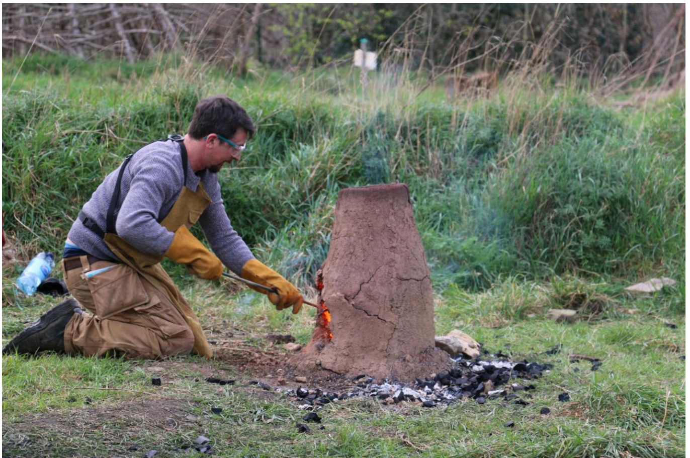
FIG 7A. RETRIEVING THE BLOOM AT THE END OF THE SMELT. FIRST THE "FALSE DOOR" IS BROKEN THROUGH (PHOTOS – UCD, CEAMC)
