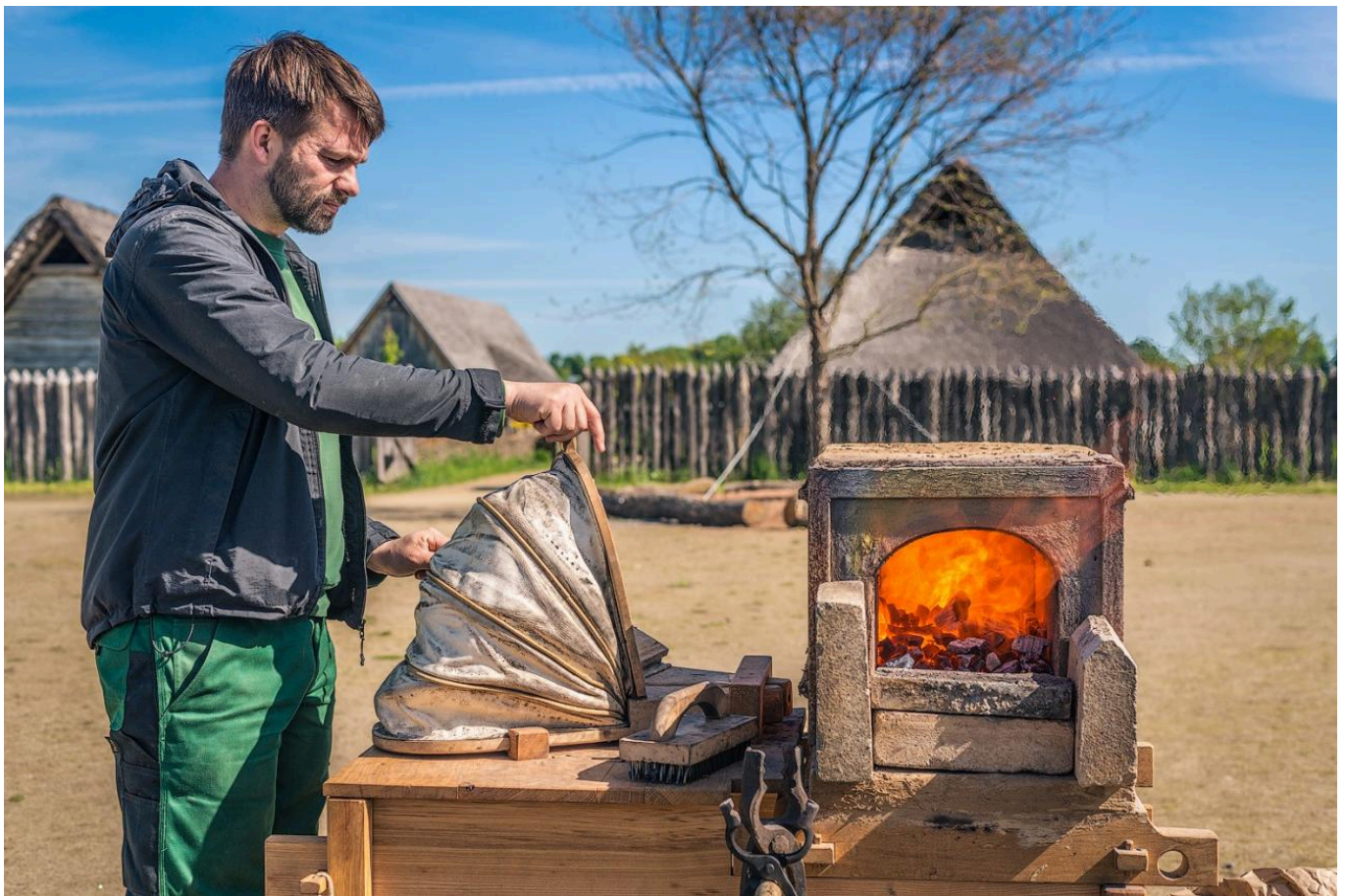
FIG 11A. FORGES USED FOR THE REFINING AND WELDING PROCESS AT THE OPEN-AIR LABORATORY DURING THE EXPERIMENT: PORTABLE FORE FOR TWO BELLOWS (FAILED). PHOTO BY M. THUMM
