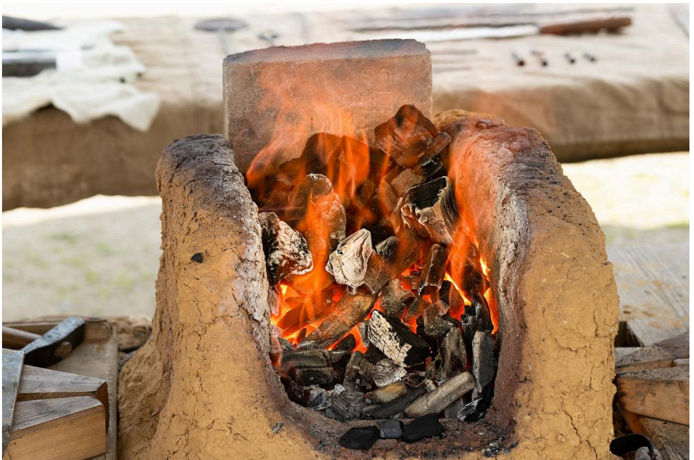
FIG 11D. FORGES USED FOR THE REFINING AND WELDING PROCESS AT THE OPEN-AIR LABORATORY DURING THE EXPERIMENT: DETAIL OF THE MODIFIED FORGE. PHOTO BY M. THUMM
