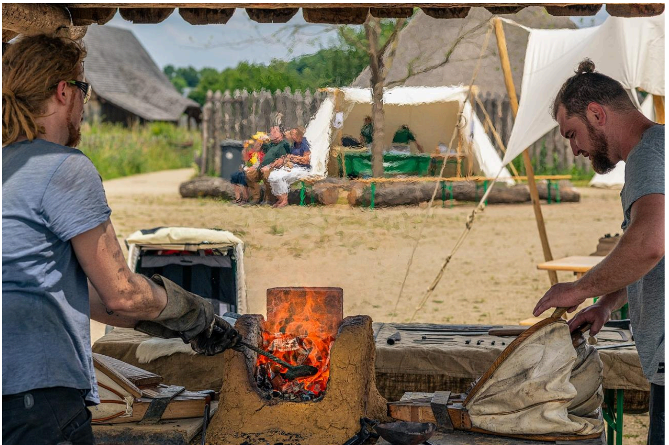
FIG 11C. FORGES USED FOR THE REFINING AND WELDING PROCESS AT THE OPEN-AIR LABORATORY DURING THE EXPERIMENT: MODIFIED FORGE FOR THE USE OF FOUR BELLOWS AT THE SAME TIME. PHOTO BY M. THUMM
