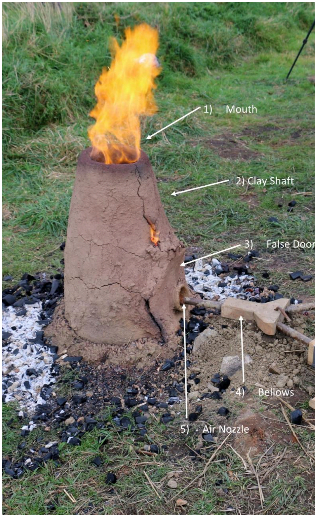
FIG 5. 1-METER-HIGH SHAFT FURNACE MID-SMELT, SHOWING MAIN ELEMENTS. 1) THE MOUTH OPENING OF THE FURNACE WHERE ORE AND CHARCOAL CAN BE ADDED. 2) HANDMADE CLAY SHAFT OF FURNACE WHICH ALLOWS THE CORRECT ATMOSPHERE TO REDUCE METAL ORE. 3) "FALSE DOOR" PROVIDING ACCESS TO THE INTERNAL FURNACE TO RETRIEVE BLOOM THROUGH A RELATIVELY THIN LAYER OF CLAY. 4) FORCED DRAFT PROVIDED BY A TWIN SET OF HAND BELLWS. 5) A CLAY AIR NOZZLE ALLOWING FORCED DRAFT TO ENTER THE FURNACE. THIS SHAFT SITS OVER A SLAG-PIT THAT COLLECTS NON-IRON (UNWANTED) MATERIAL. (PHOTO – UCD, CEAMC)
