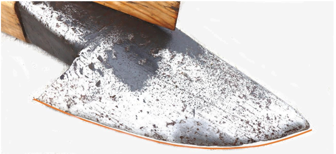
FIG 19. WEAR SIGNS ON AN ASSYMMETRICAL PLOUGH-SHARE FROM THE OPEN-AIR LABORATORY (AFTER FIVE YEARS OF REGULAR USE). PHOTO BY C. KROPP
