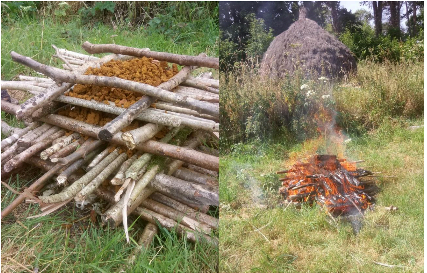
FIG 4. ROASTING C.60KG OF BOG IRON ORE USING A LAYERED PYRE CONSTRUCTION AT UCD CENTRE FOR EXPERIMENTAL ARCHAEOLOGY AND MATERIAL CULTURE. LEFT SHOWS THE LAYERED STRUCTURE ALLOWING A LARGE QUANTITY OF ORE TO BE ROASTED. RIGHT SHOWS THE STRUCTURE ONCE LIT AND BURNING DOWN (EARLY MEDIEVAL ROUNDHOUSE IN BACKGROUND). (PHOTOS – UCD, CEAMC)
