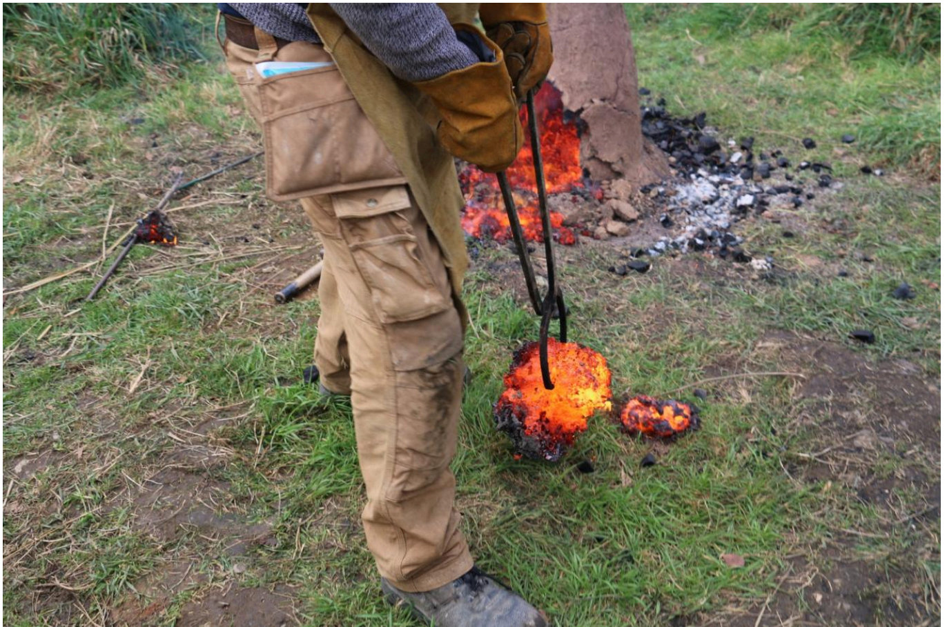
FIG 7C. RETRIEVING THE BLOOM AT THE END OF THE SMELT. THE BLOOM CAN BE SEEN TO BE A LARGE, GLOWING, AMORPHOUS PIECE OF MATERIAL THAT LOOKS SIMILAR IN APPEARANCE TO OTHER SLAG, VITREOUS MATERIAL, ETC. ALSO INSIDE THE FURNACE. (PHOTOS – UCD, CEAMC)
