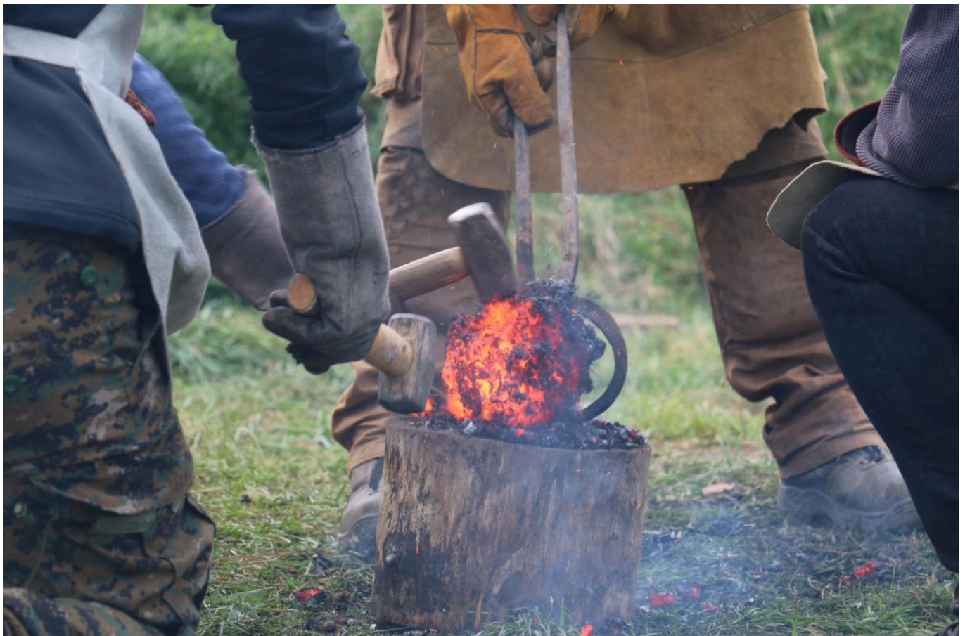
FIG 7D. RETRIEVING THE BLOOM AT THE END OF THE SMELT. THE BLOOM IS PLACED ON A HARD SURFACE (A WOODEN STUMP IN THIS CASE) AND HIT REPEATEDLY. DURING THIS, THE BLOOM IS ALSO SPLIT TO ALLOW
