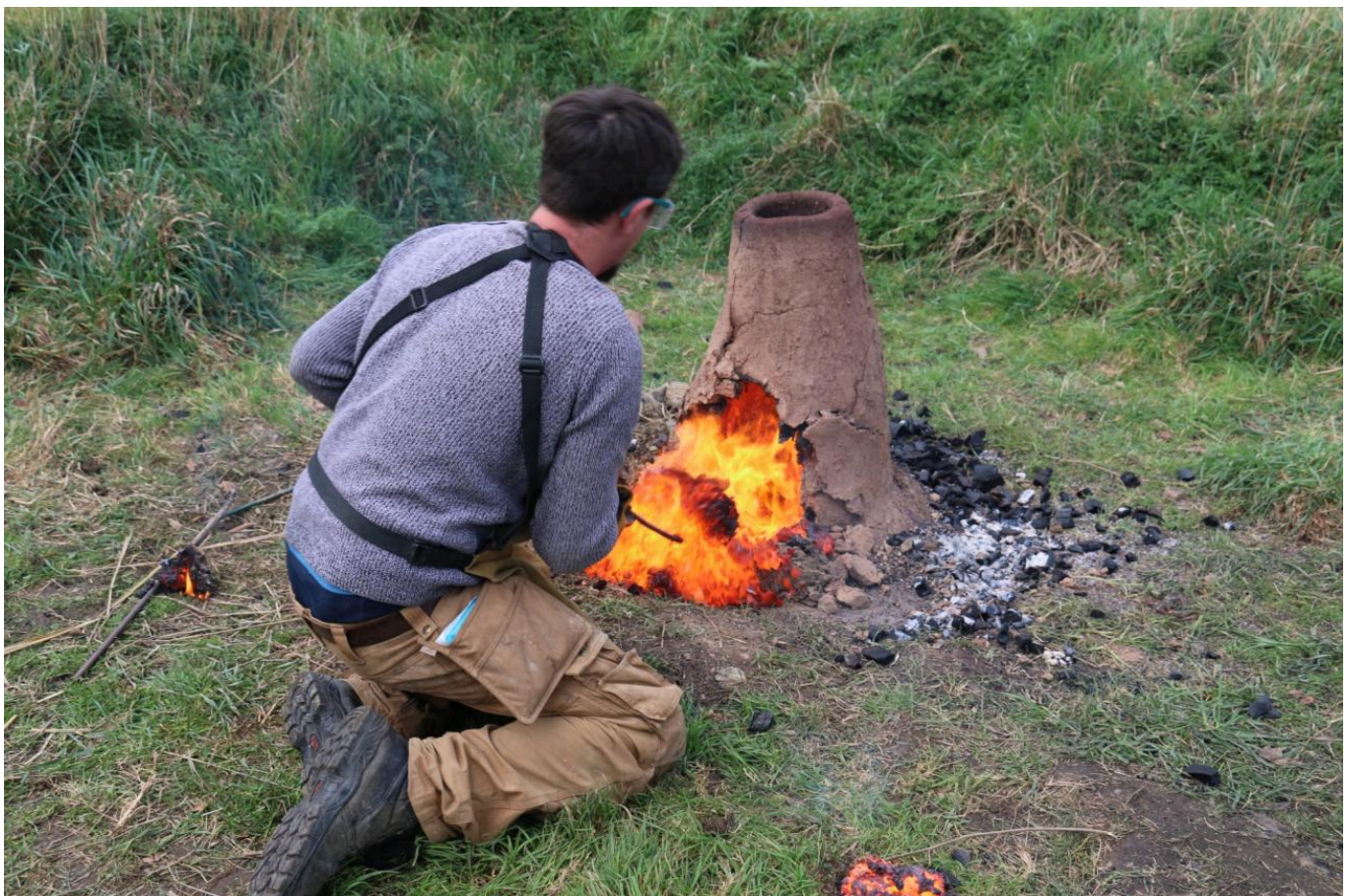
FIG 7B. RETRIEVING THE BLOOM AT THE END OF THE SMELT. THIS ALLOWS THE BLOOM TO BE IDENTIFIED AND GRABBED WITH A METAL TONGS. (PHOTOS – UCD, CEAMC)
