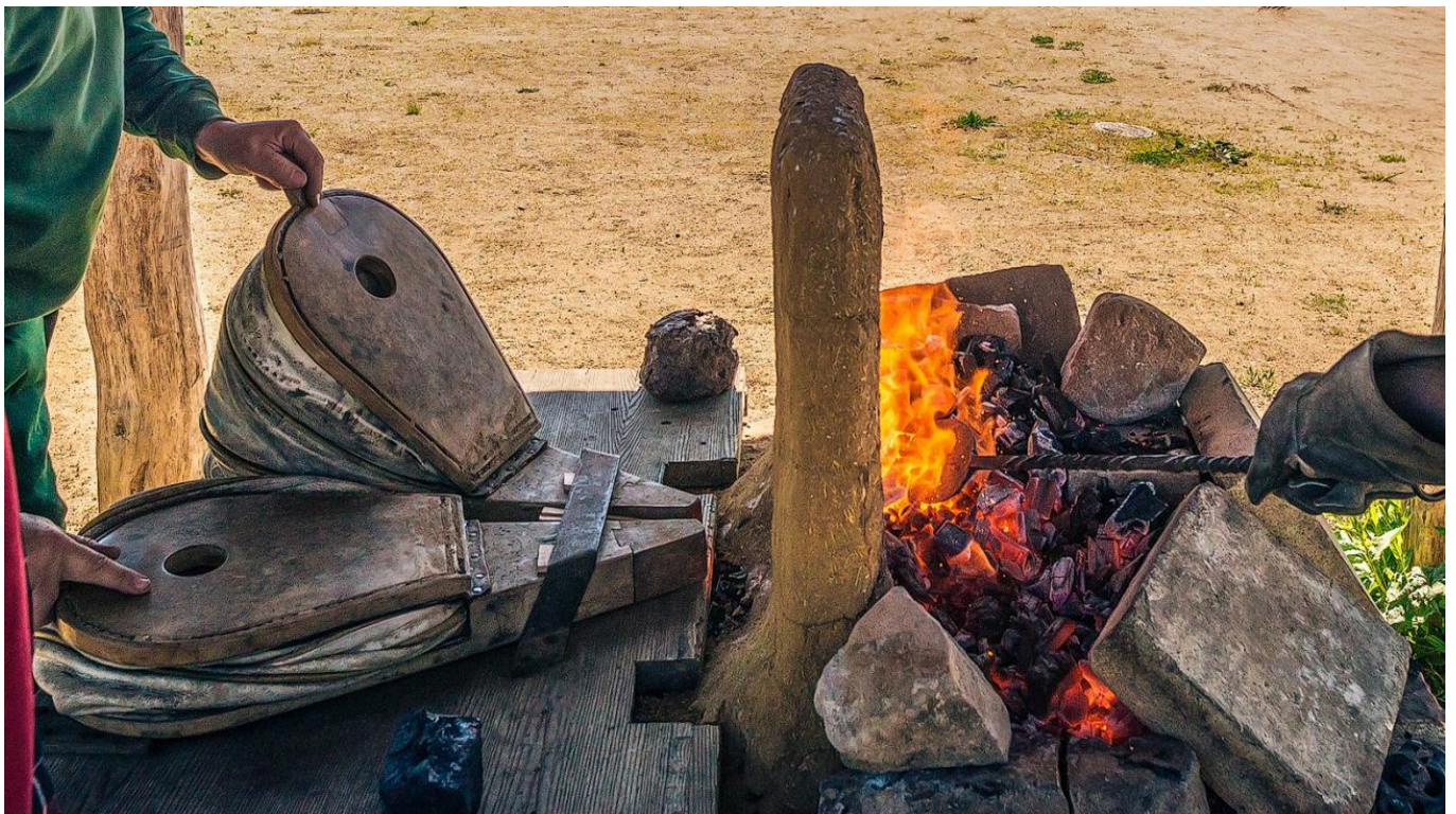
FIG 11B. FORGES USED FOR THE REFINING AND WELDING PROCESS AT THE OPEN-AIR LABORATORY DURING THE EXPERIMENT: REGULAR FORE AT THE OPEN-AIR LABORATORY OPERATED BY TWO BELLOWS. PHOTO BY M. THUMM
