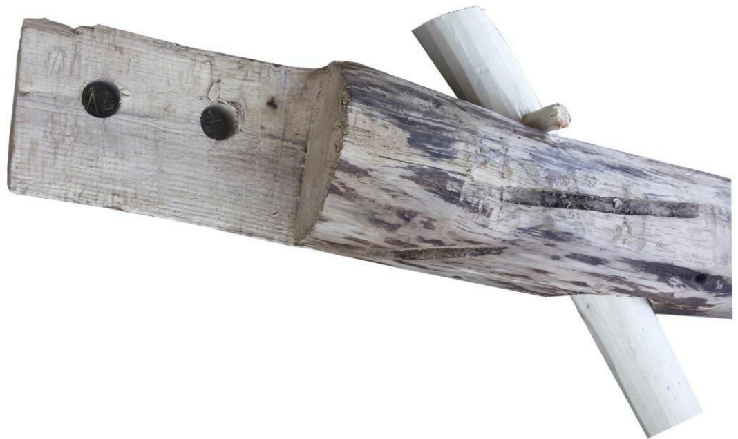
FIG 16B. CONSTRUCTION DETAILS OF THE ARD: CONNECTION-DETAILS OF THE BEAM EXTENSION. PHOTO BY V. TÖNGI
