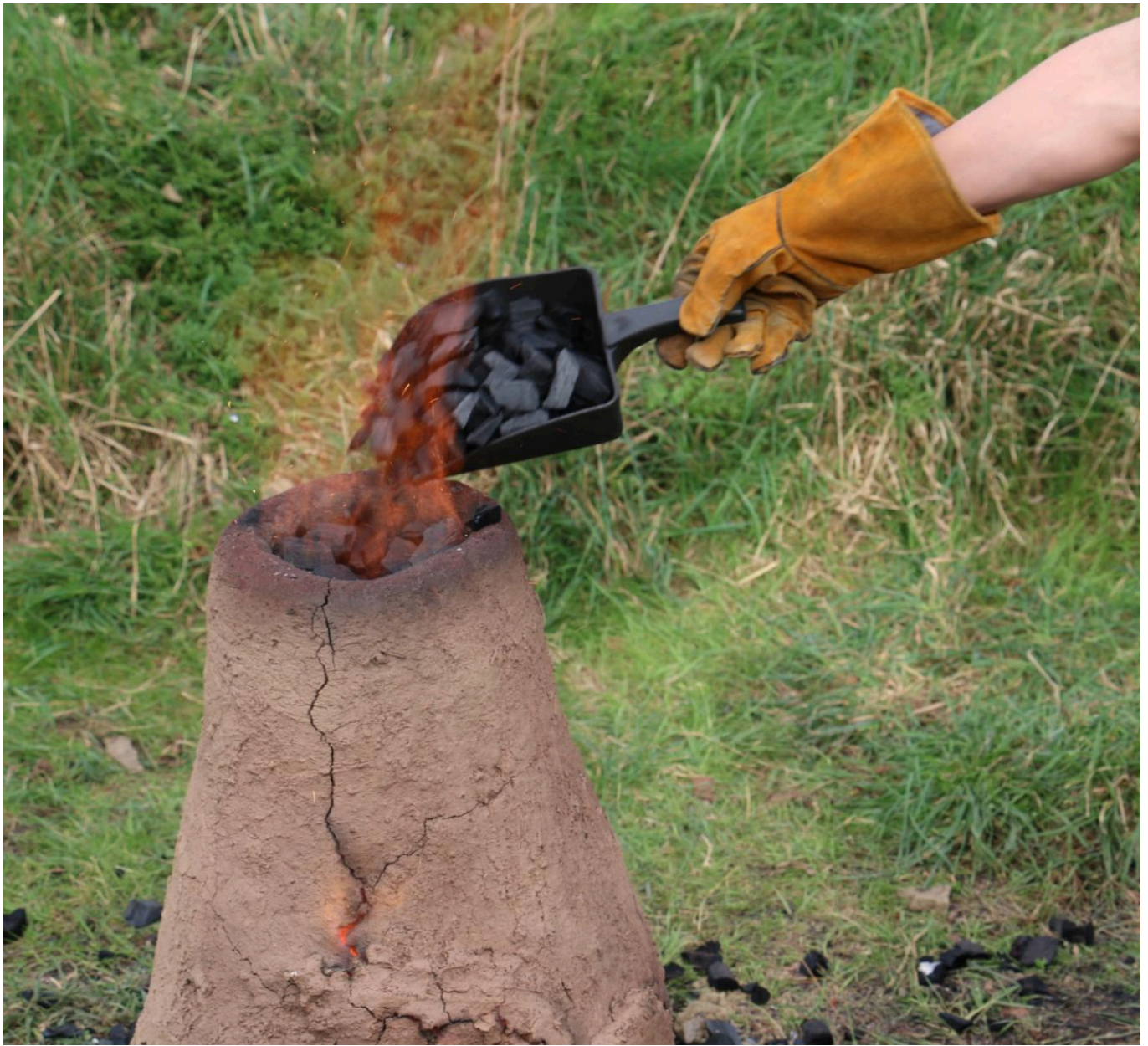
FIG 6. "CHARGING" THE FURNACE WITH ADDITIONAL CHARCOAL. AS FUEL BURNS OUT IN THE LOWER FURNACE (ROUGHLY AT GROUND LEVEL) THE LEVEL OF CHARCOAL AT THE MOUTH OF THE FURNACE DROPS, PROVIDING SPACE FOR ADDITIONAL MATERIAL TO BE ADDED IN LAYERS. FOR THIS SMELT, ORE WAS ADDED FIRST FOLLOWED QUICKLY BY DOUBLE THE WEIGHT OF CHARCOAL. THIS WAS ALLOWED TO BURN DOWN UNTIL SUFFICIENT SPACE (ROUGHLY 10-12CM) WAS ONCE AGAIN CREATED. (PHOTOS – UCD, CEAMC)
