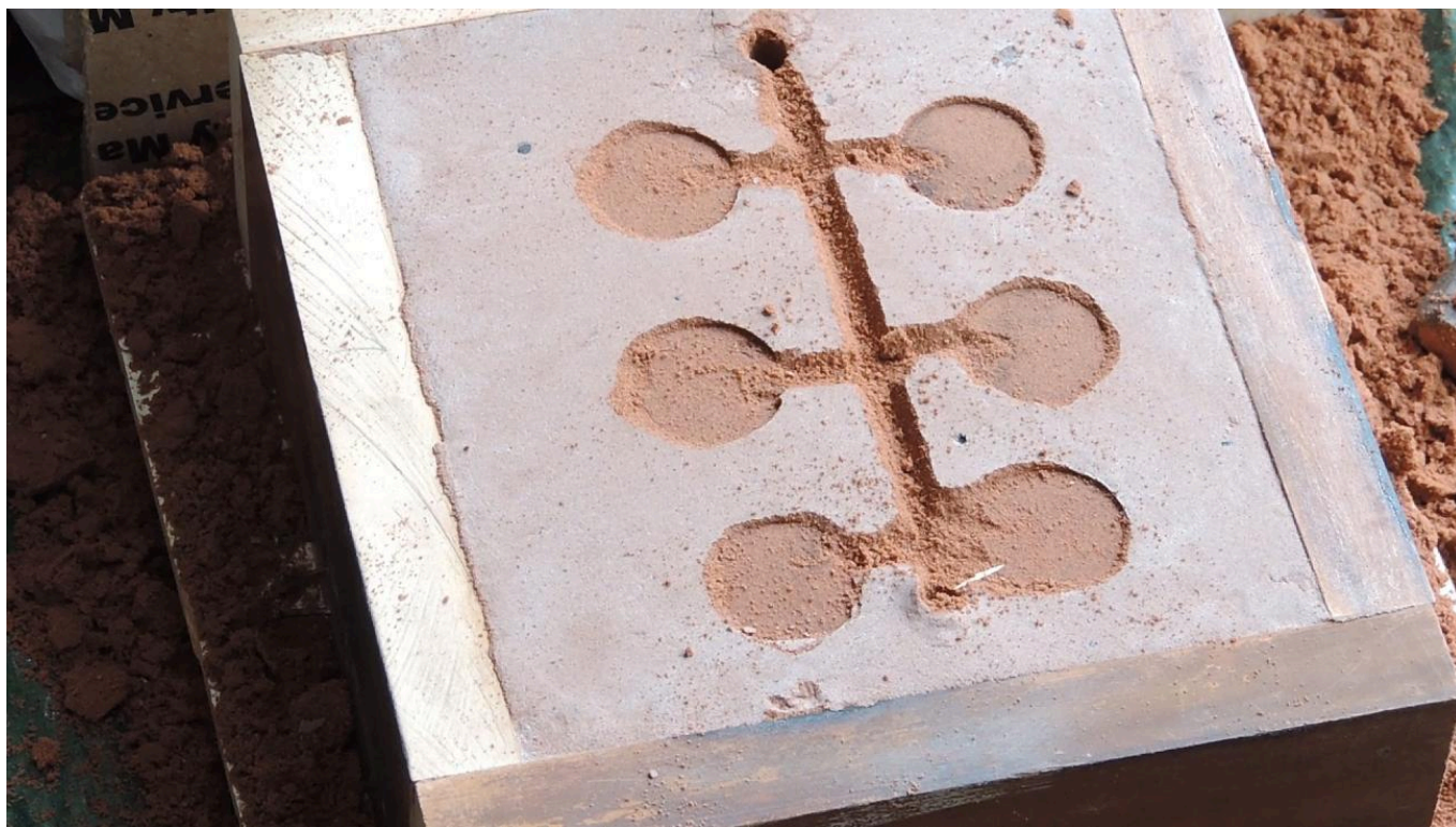
FIG 9A. : COPE & DRAG SAND MOULD LOWER HALF AFTER PACKING SHOWING DISK PATTERNS AND ADDED RUNNERS. PHOTO BY CHELSEA KAUFMAN
