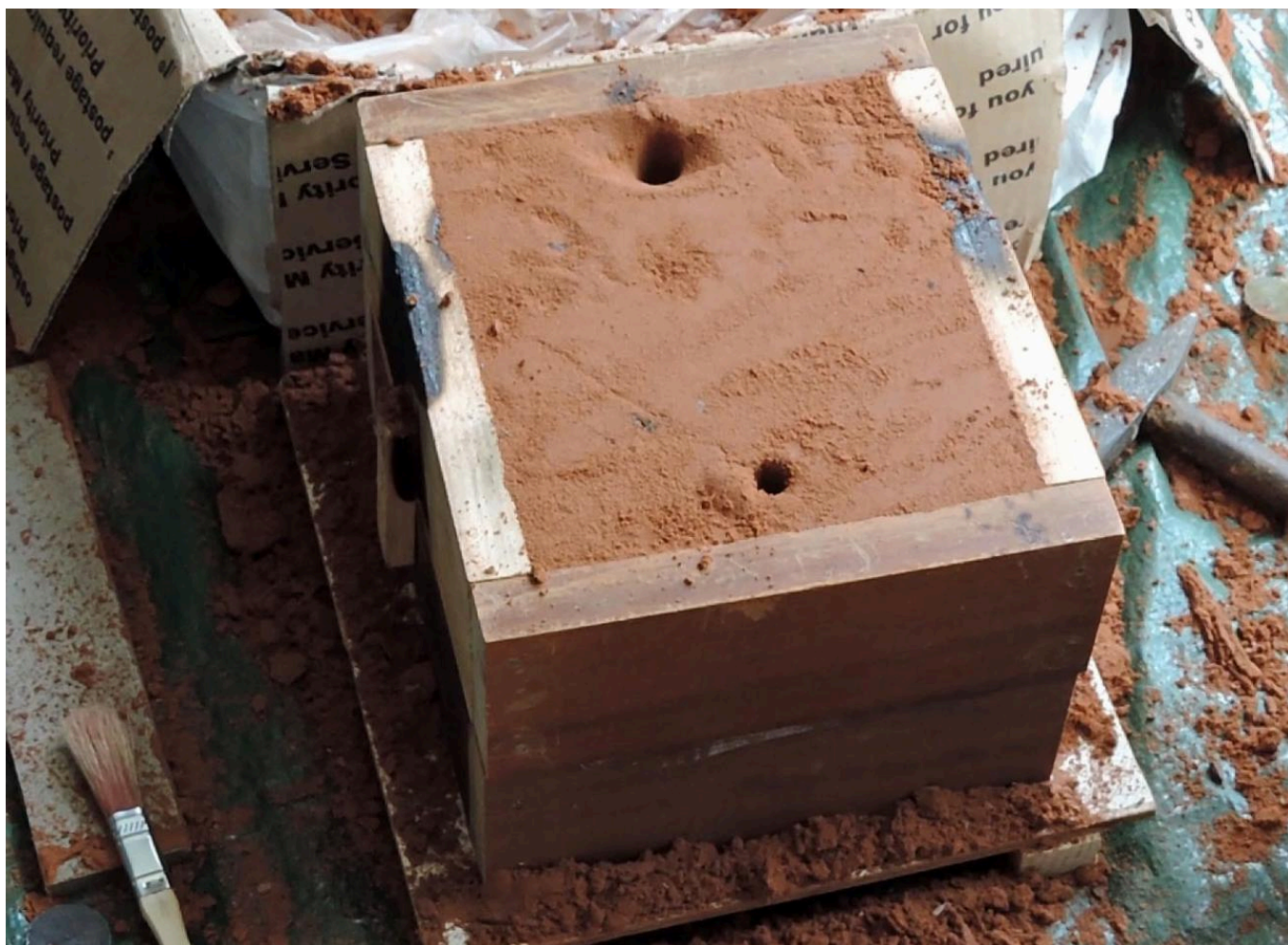
FIG 9B. COMPLETED AND CLOSED MOULD. PHOTO BY CHELSEA KAUFMAN
