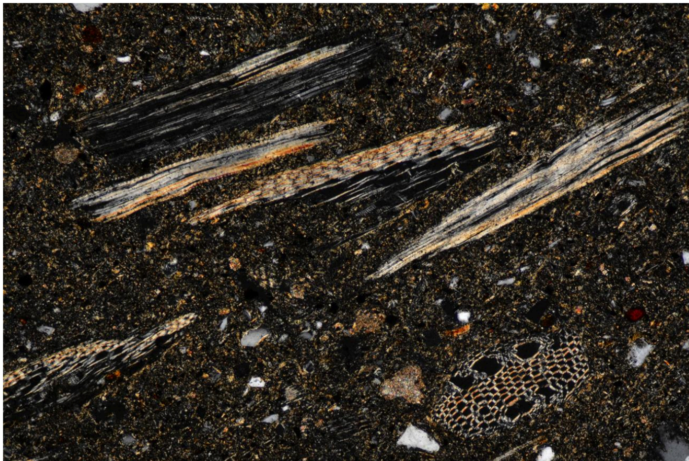
FIG 16B. PHOTOMICROGRAPH TAKEN WITH CROSS POLARIZED LIGHT OF THIN SECTION OF SAMPLE 9B SHOWING ORGANIC INCLUSIONS FROM HORSE DUNG: DETAIL AT 10X. PHOTO BY G. D'ERCOLE.
