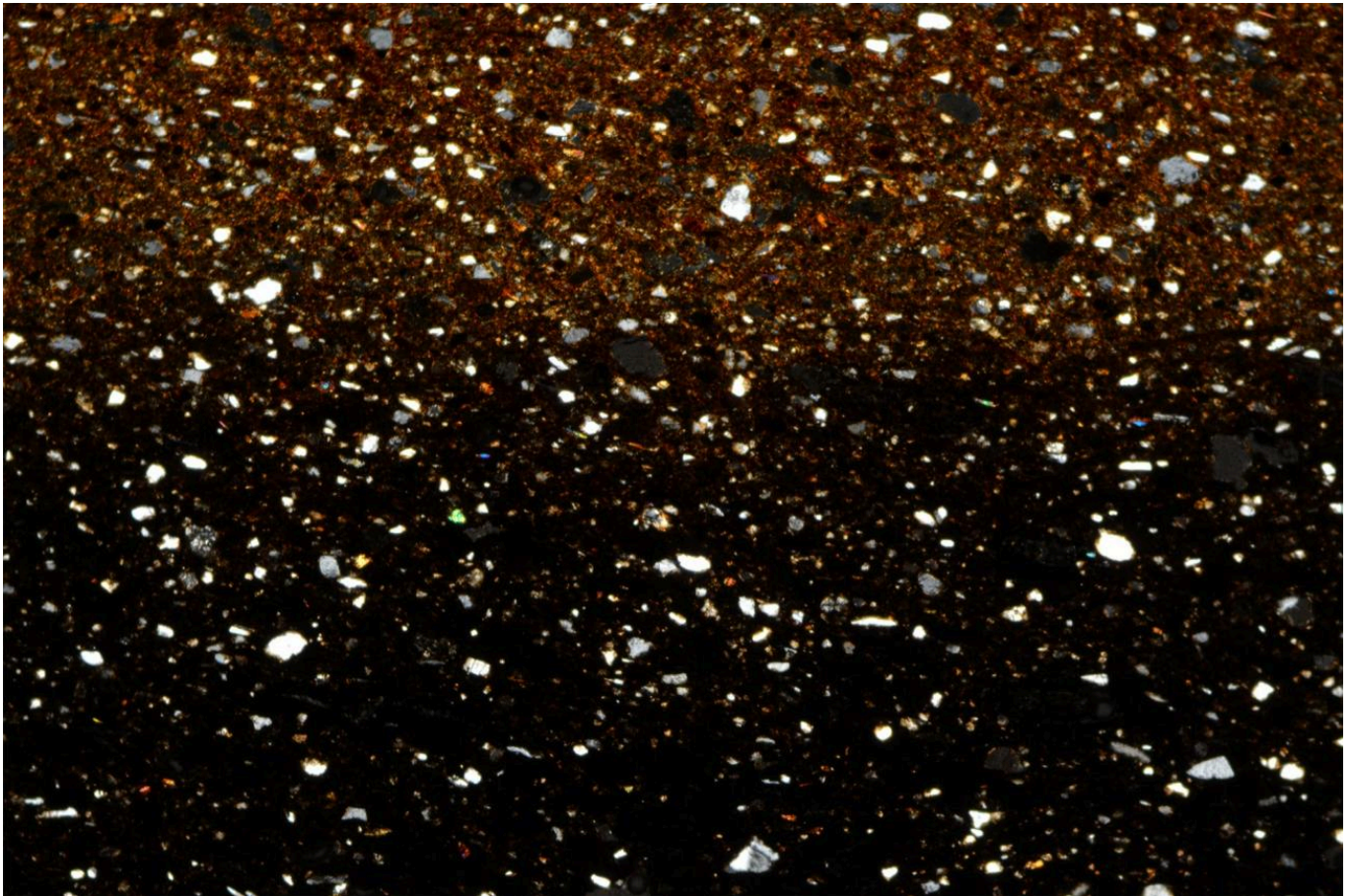
FIG 10. PHOTOMICROGRAPH TAKEN WITH CROSS POLARIZED LIGHT OF THIN SECTION SHOWING THE TEXTURE OF THE NEW KINGDOM NUBIAN STYLE SAMPLE SAV/S 77 (MAGNIFICATION AT 4X). PHOTO BY G. D'ERCOLE
