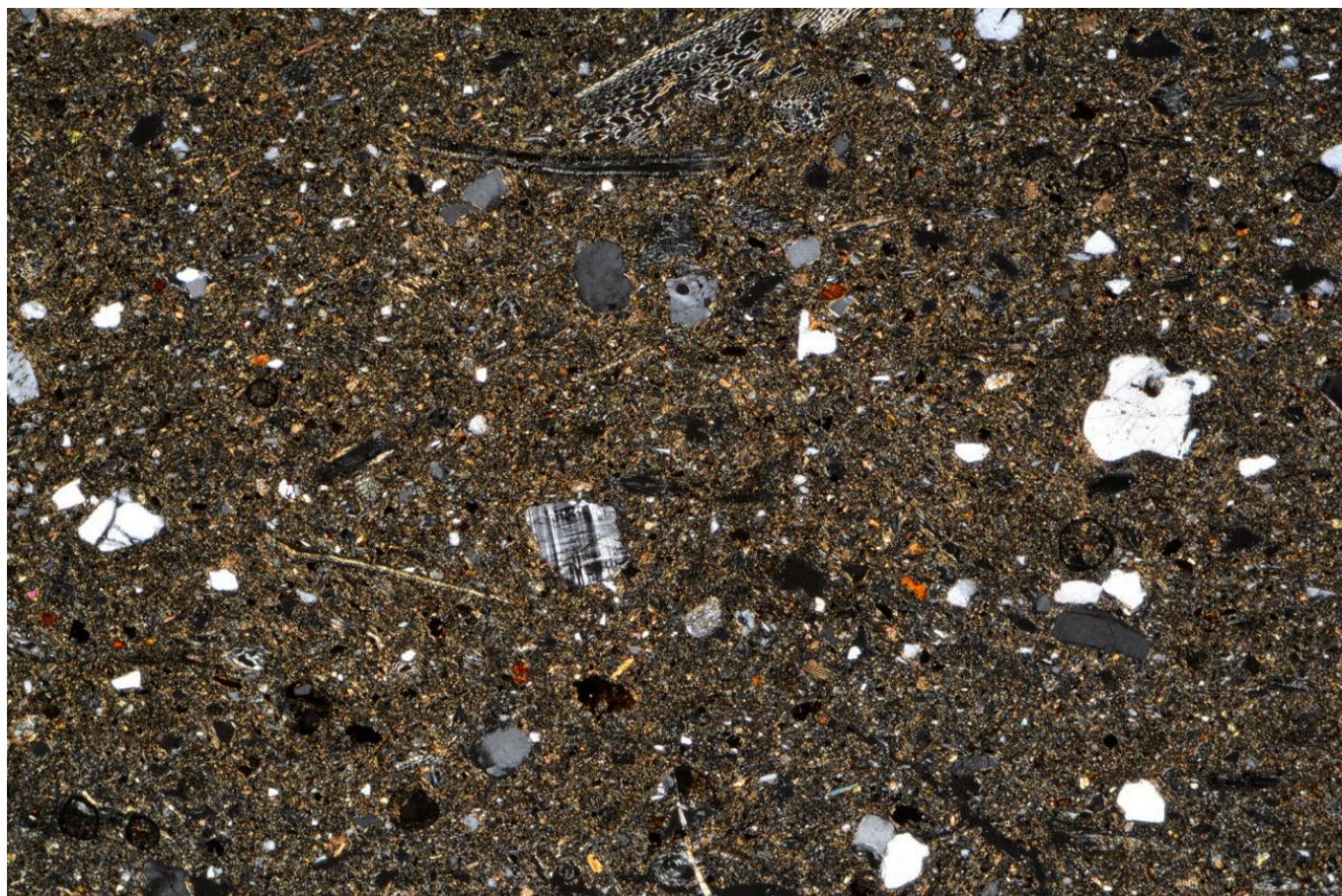
FIG 15. PHOTOMICROGRAPH TAKEN WITH CROSS POLARIZED LIGHT OF THIN SECTION OF SAMPLE 4A SHOWING ORGANIC INCLUSIONS FROM CATTLE DUNG (MAGNIFICATION AT 4X). PHOTO BY G. D'ERCOLE
