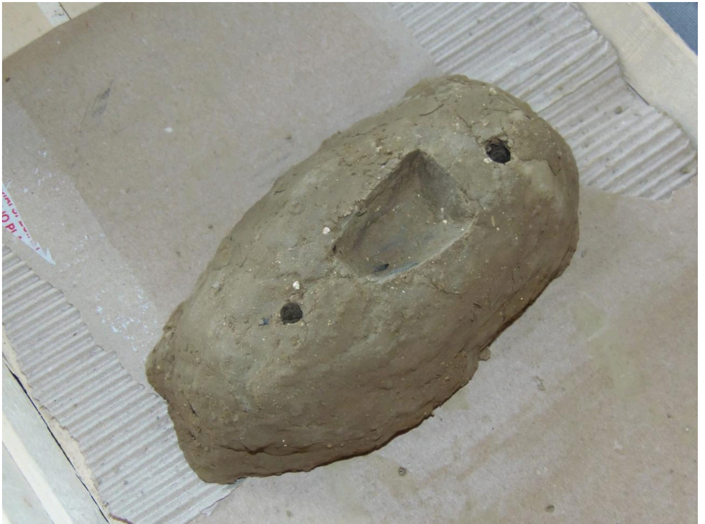
FIG 4. MAKING MF-1 REPLICA MOULD (EARTH). PHOTO BY MAURO FIORENTINI
