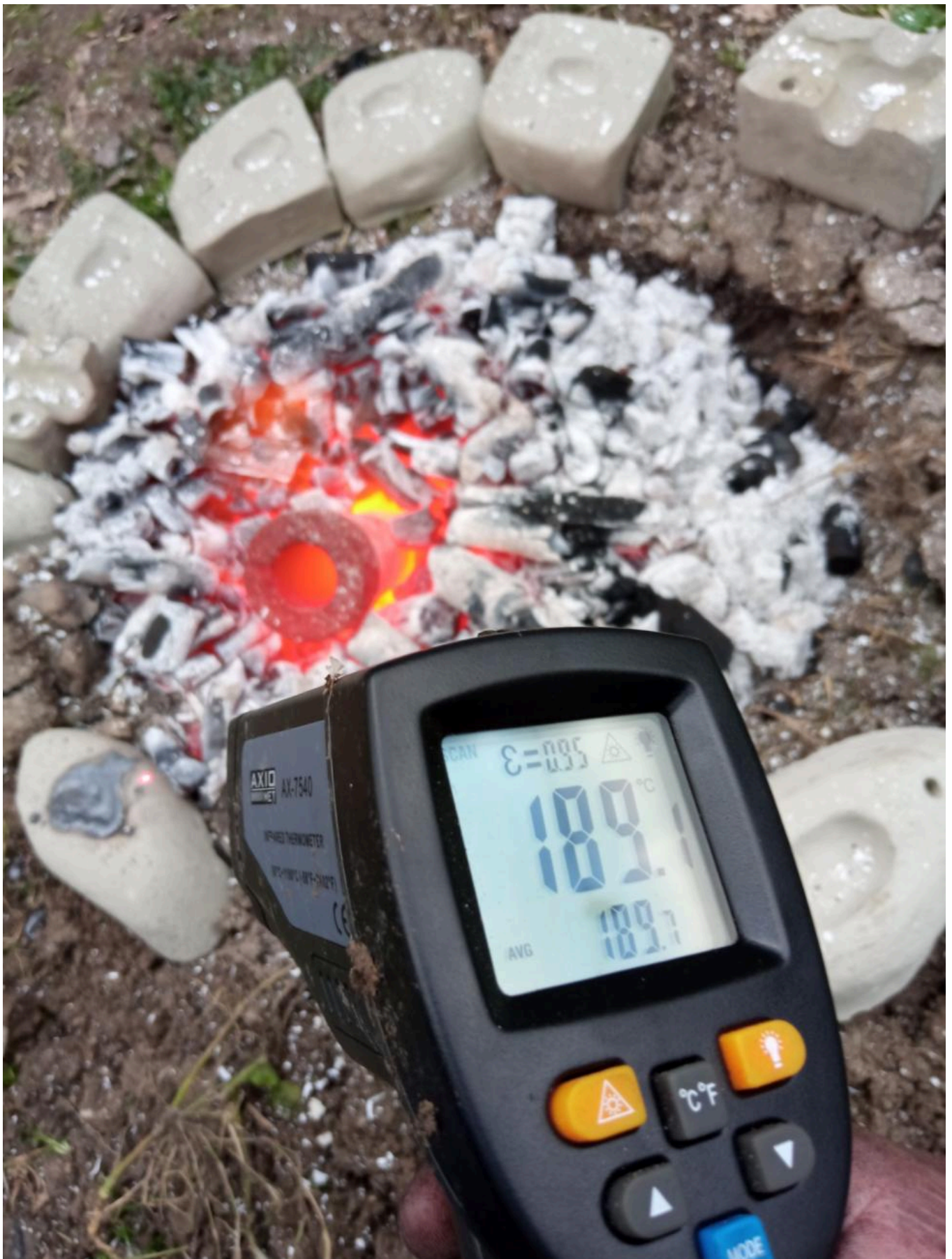
FIG 42. DURING THE MELTING, THE MAXIMUM RECORDED TEMPERATURE ON MF MAV-II SURFACE WAS LESS THAN 190° C, WHICH MEANS THE MARL SUSTAINED THE MELTING WITHOUT EVEN BEING FIRED PROPERLY. PHOTO BY MAURO FIORENTINI
