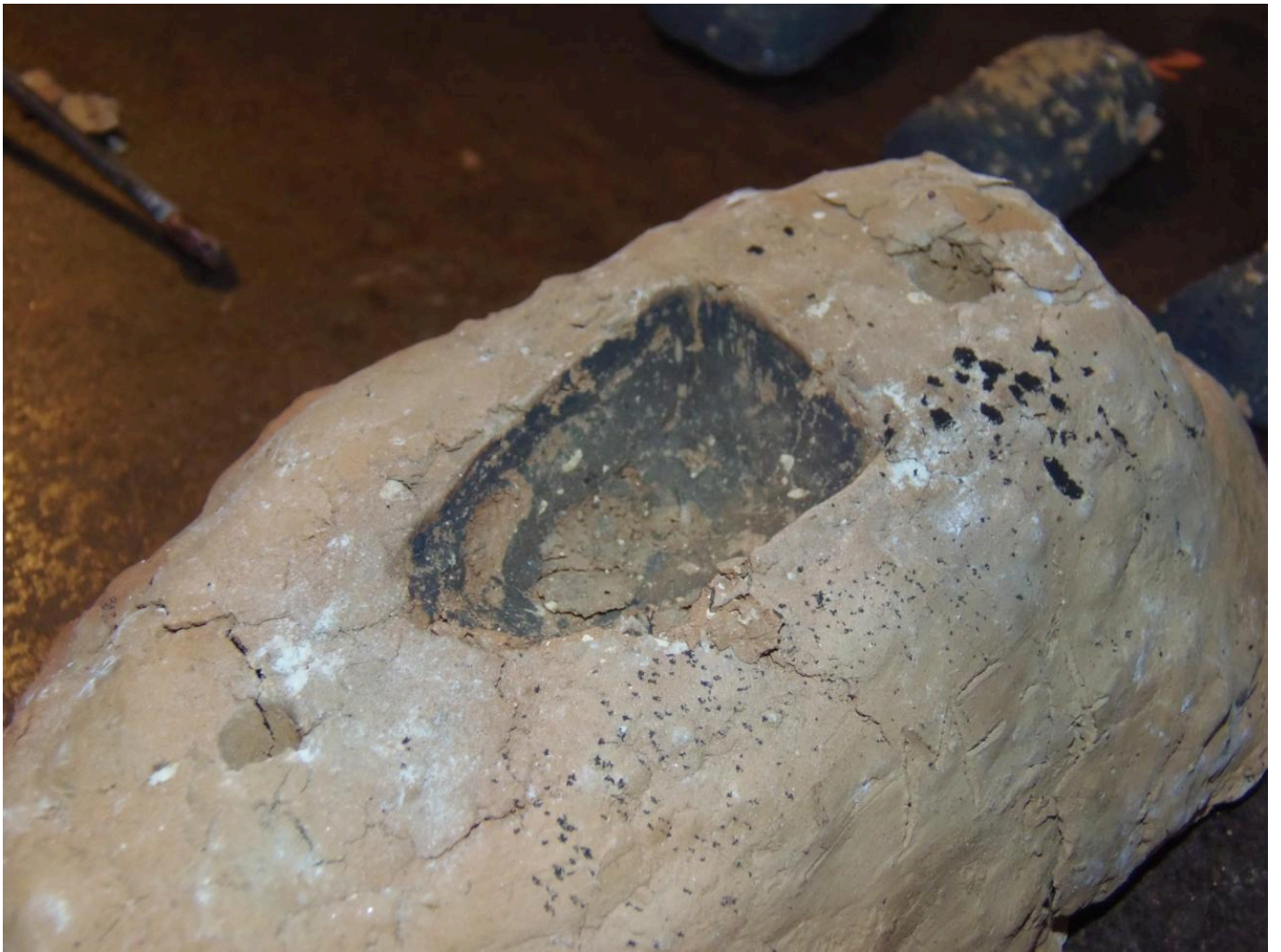
FIG 16. THIS PICTURE SHOW HOW THE HOLLOW OF MF-1 HAS WORN OUT AFTER FIVE CASTINGS. PHOTO BY MAURO FIORENTINI
