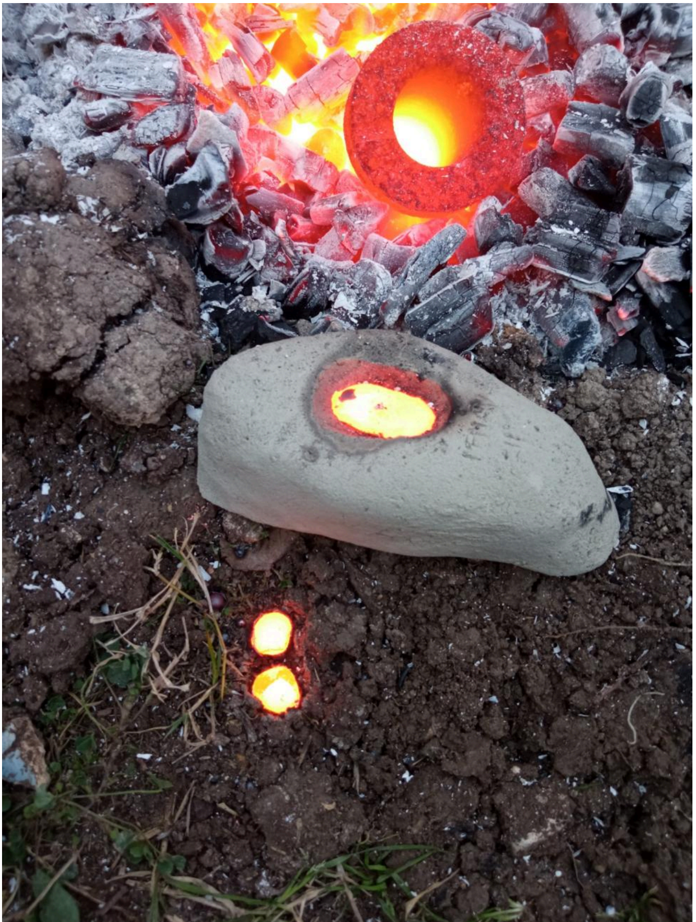
FIG 34. THE BACKUP CRUCIBLE, A MODERN ONE MADE OF GRAPHITE, WAS PUT IN THE FORGE AND FILLED OF COPPER. A SERIES OF THREE QUICK MELTINGS WERE SUCCESSFULLY PERFORMED, ALL USING MF MAV-II MOULD. DESPITE ITS TEMPERATURE BEING CONSTANTLY LOW (FIGURE 177), THE MOULD'S RESISTANCE TO THE THERMAL SHOCKS WAS OUTSTANDING, BEARING NO SIGNS OF DAMAGES AT THE END OF THE ACTIVITY. BOILING COPPER WAS A CONSTANT, HAVING HAPPENED AT EVERY CASTING. PHOTO BY MAURO FIORENTINI
