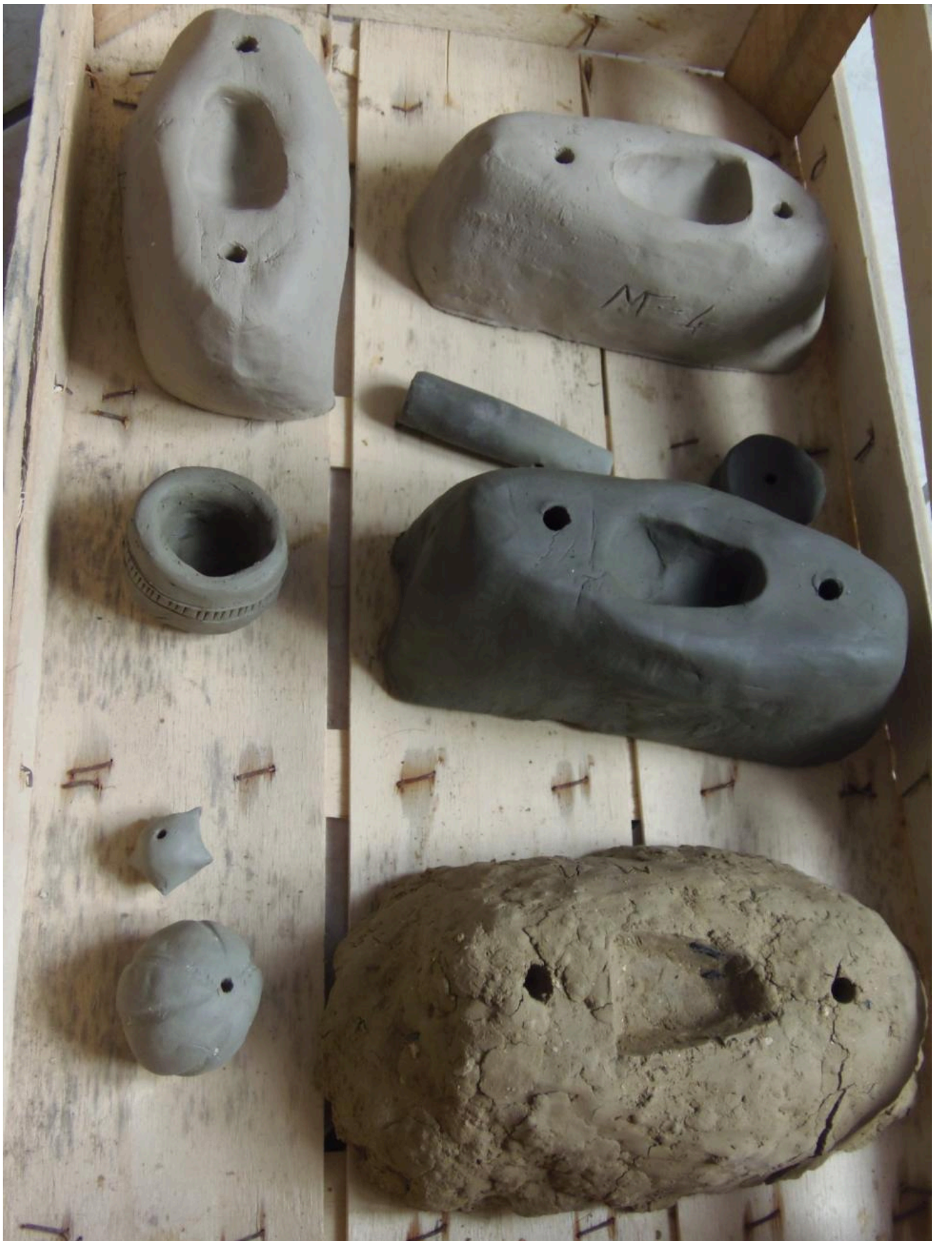
FIG 6. THE FIRST FOUR MOULDS, THE MOSCOSI DI CINGOLI CRUCIBLE REPLICA AND OTHER CLAY OBJECTS DRYING. PHOTO BY MAURO FIORENTINI
