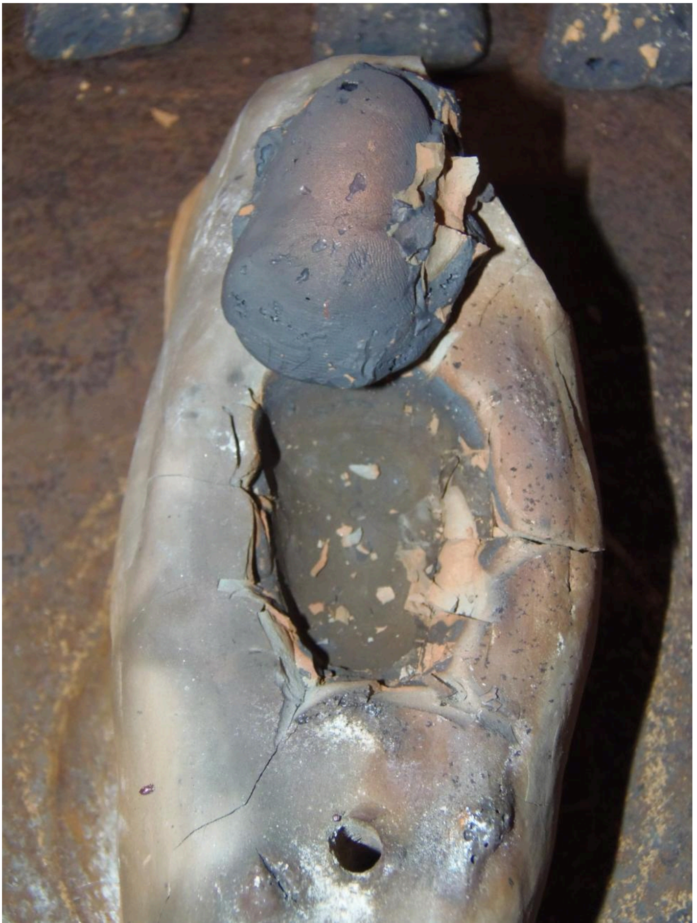
FIG 14. THIS PICTURE SHOWS HOW THE HOLLOW OF MF-2 HAS WORN OUT AFTER FIVE CASTINGS. PHOTO BY MAURO FIORENTINI
