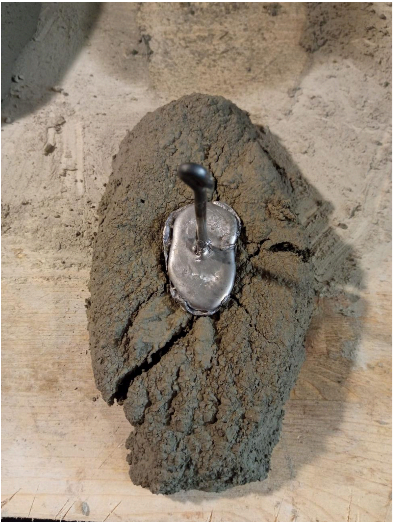
FIG 29. THE UNSUCCESSFUL METHOD OF SETTLING HAS BEEN TESTED WITH SCHLIER MARL TOO, BUT IT WAS A FAILURE AS WELL. WHAT WAS SUPPOSED TO BECOME MOULD MF MAV-I, OBTAINED WITH THIS METHOD, HAD TO BE DISCARDED DUE TO THE CRACKS THAT GENERATED DURING ITS DRYING. PHOTO BY MAURO FIORENTINI
