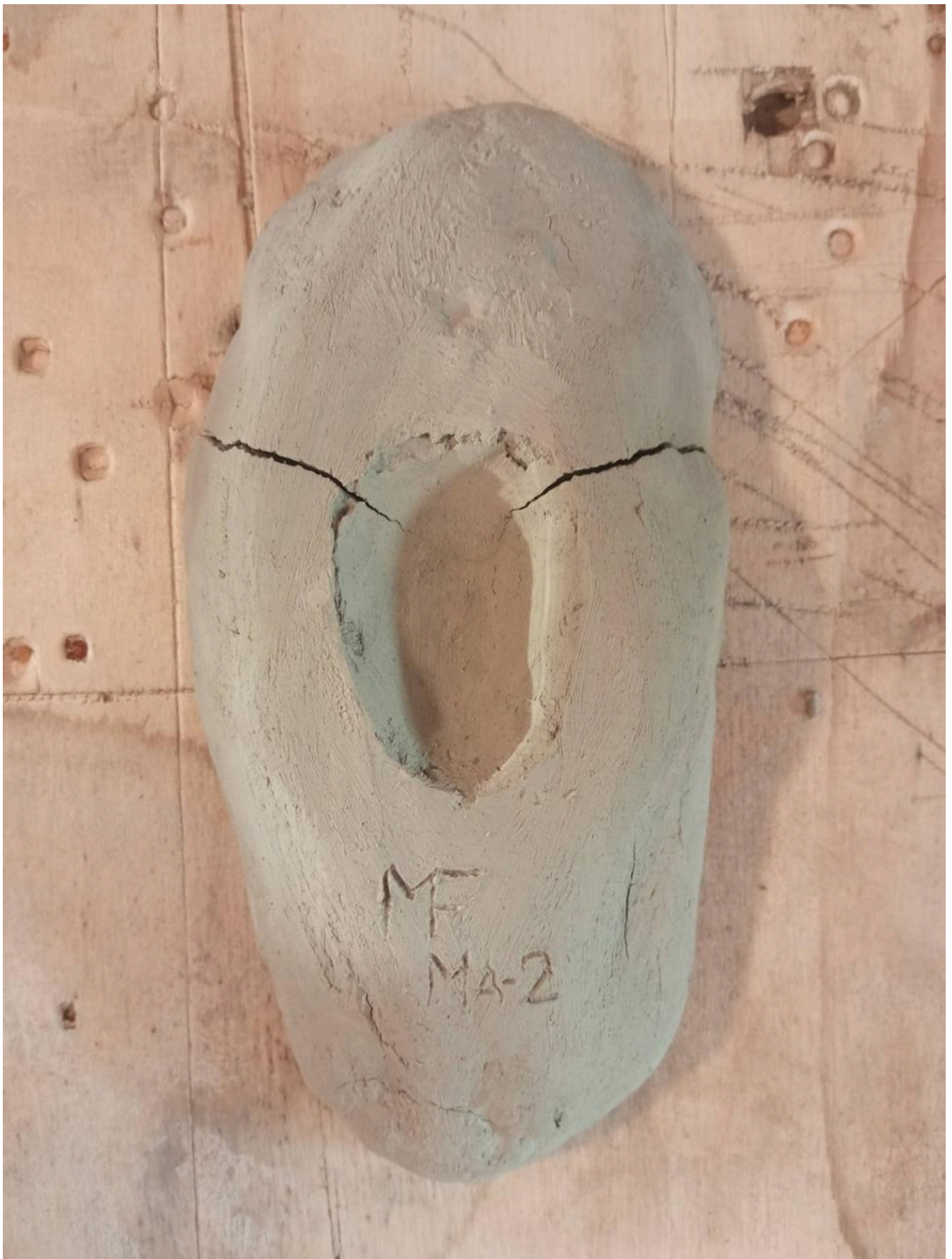
FIG 23. MF MA-2 BEGUN TO CRACK WHILE DRYING. PHOTO BY MAURO FIORENTINI
