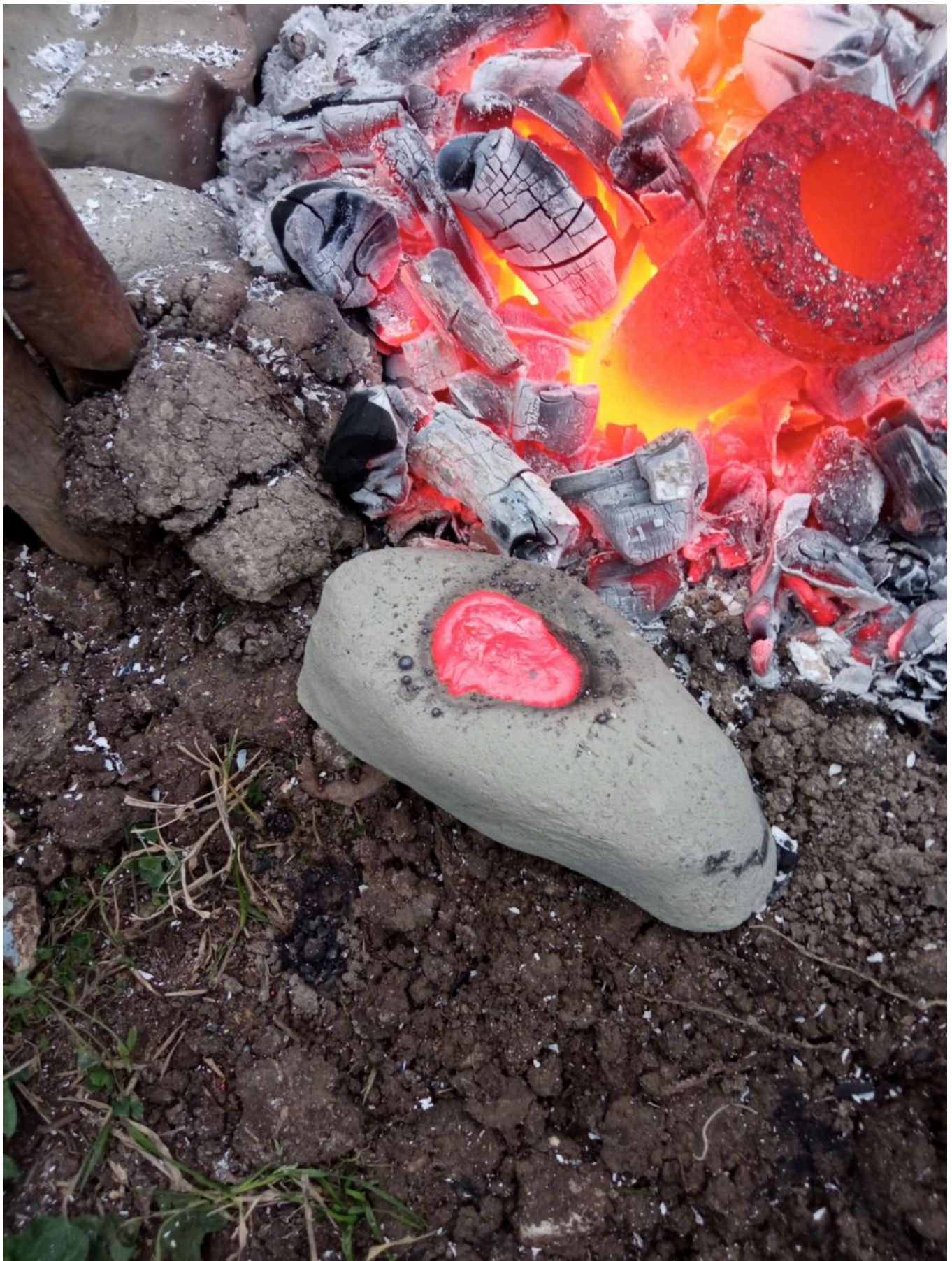
FIG 35. THE BACKUP CRUCIBLE, A MODERN ONE MADE OF GRAPHITE, WAS PUT IN THE FORGE AND FILLED OF COPPER. A SERIES OF THREE QUICK MELTINGS WERE SUCCESSFULLY PERFORMED, ALL USING MF MAV-II MOULD. DESPITE ITS TEMPERATURE BEING CONSTANTLY LOW (FIGURE 177), THE MOULD'S RESISTANCE TO THE THERMAL SHOCKS WAS OUTSTANDING, BEARING NO SIGNS OF DAMAGES AT THE END OF THE ACTIVITY. BOILING COPPER WAS A CONSTANT, HAVING HAPPENED AT EVERY CASTING. PHOTO BY MAURO FIORENTINI
