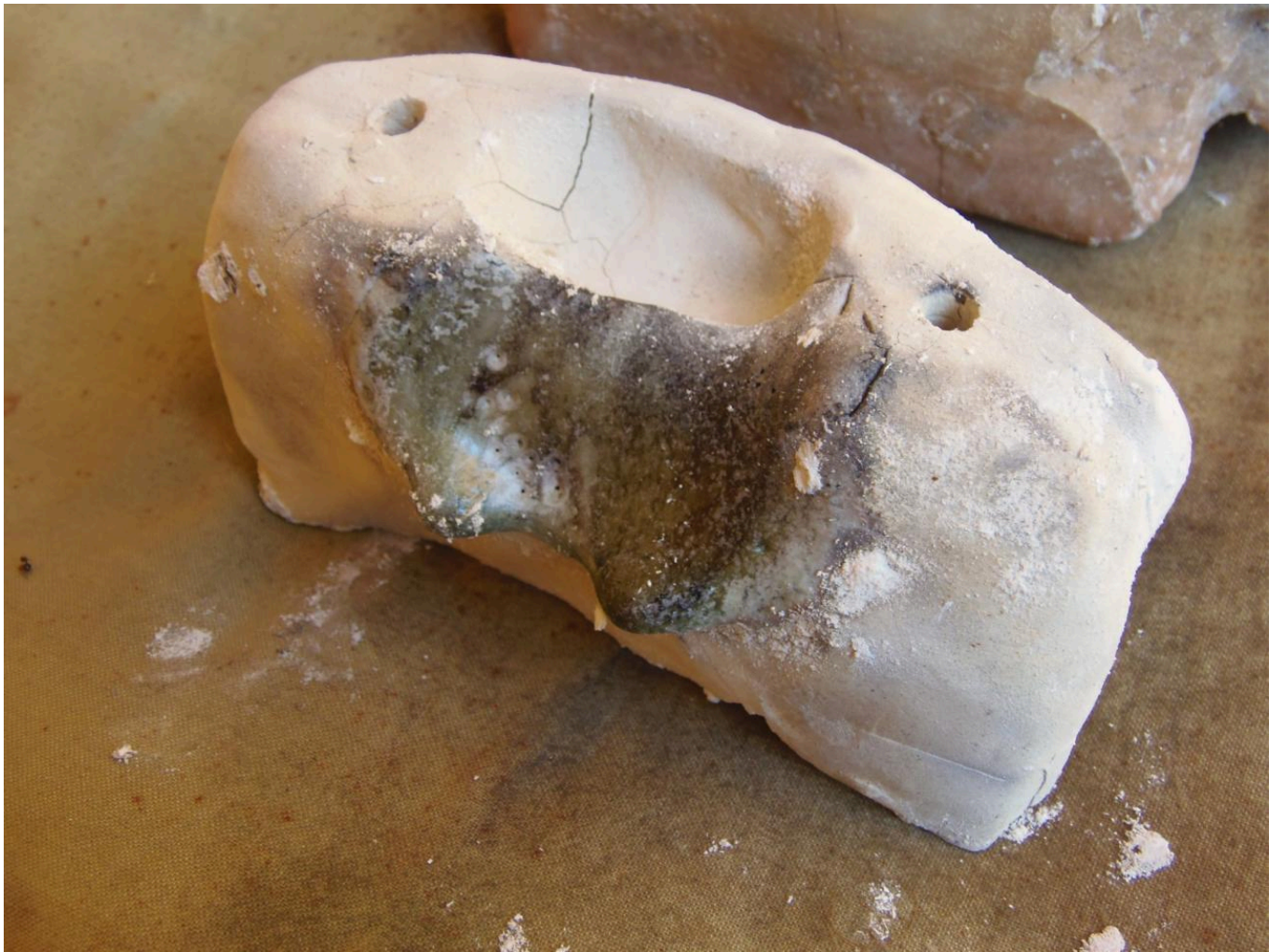
FIG 8. TWO OF THE MOULDS HAD TO BE DISCARDED AFTER THE FIRING. PHOTO BY MAURO FIORENTINI
