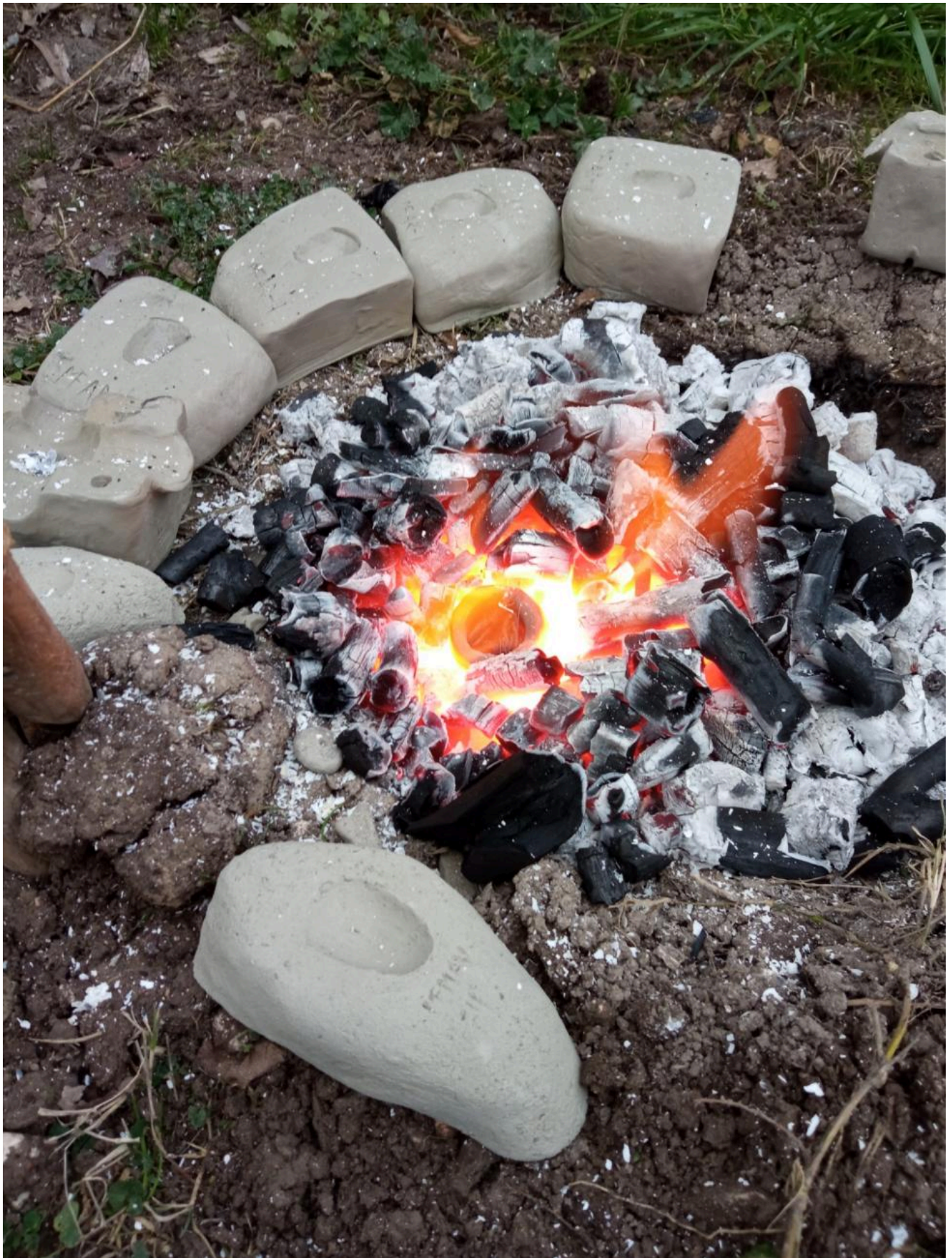
FIG 32. AS THE FIRE IS LIT AND THE TEMPERATURE RISES (REACHING A RECORDED MAXIMUM OF 1027° C), THE MOULDS ARE PUT CLOSER TO THE FIRE. PHOTO BY MAURO FIORENTINI
