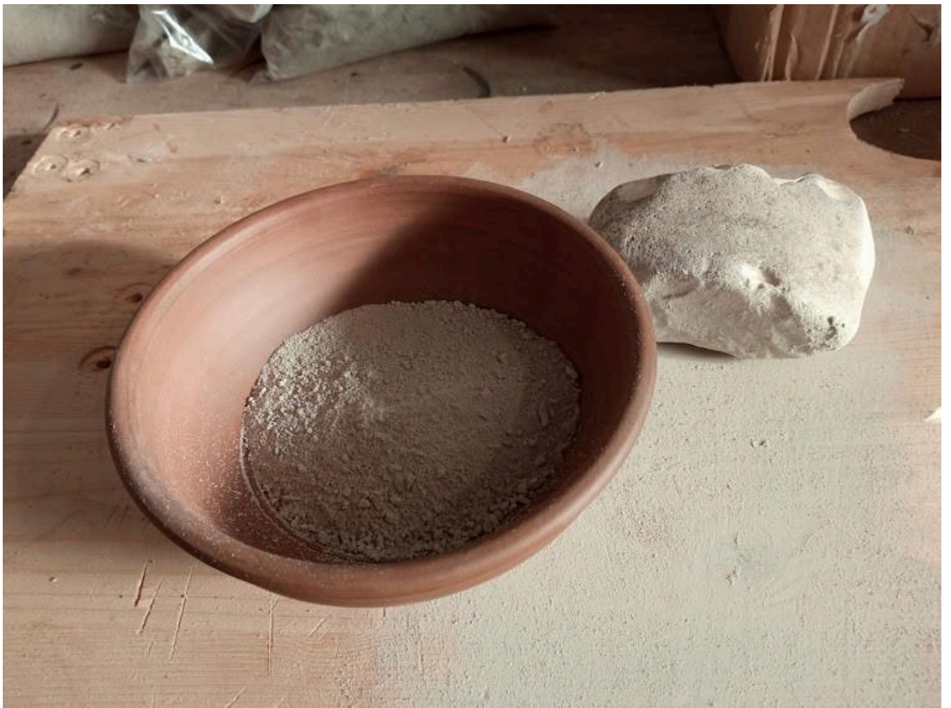
FIG 20. USING A STONE TOOL TO CRUSH AND PULVERIZE THE MARL FROM APIRO. PHOTO BY MAURO FIORENTINI
