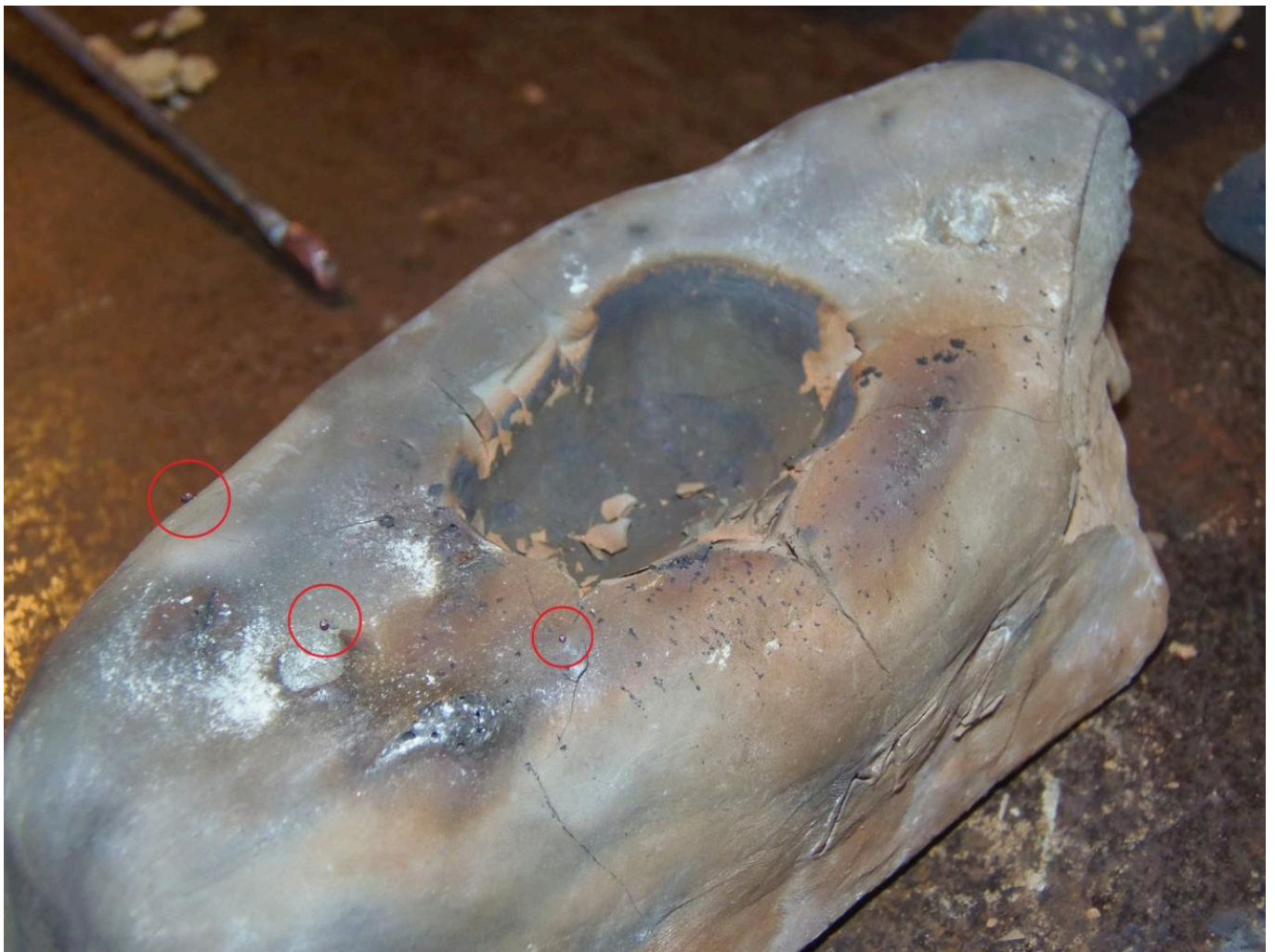
FIG 17. PARTICULAR OF METAL PRILLS STUCK ON MF-2'S SURFACE. PHOTO BY MAURO FIORENTINI
