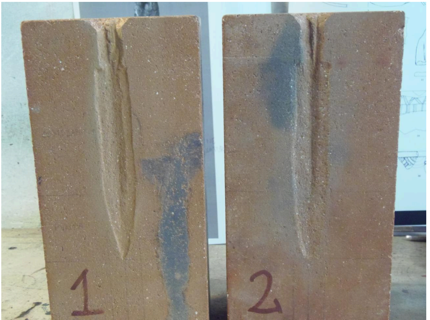
FIG 9. THE MOULDS FOR THE BAFFONI CAVE BRONZE DAGGER REPLICAS. PHOTO BY MAURO FIORENTINI
