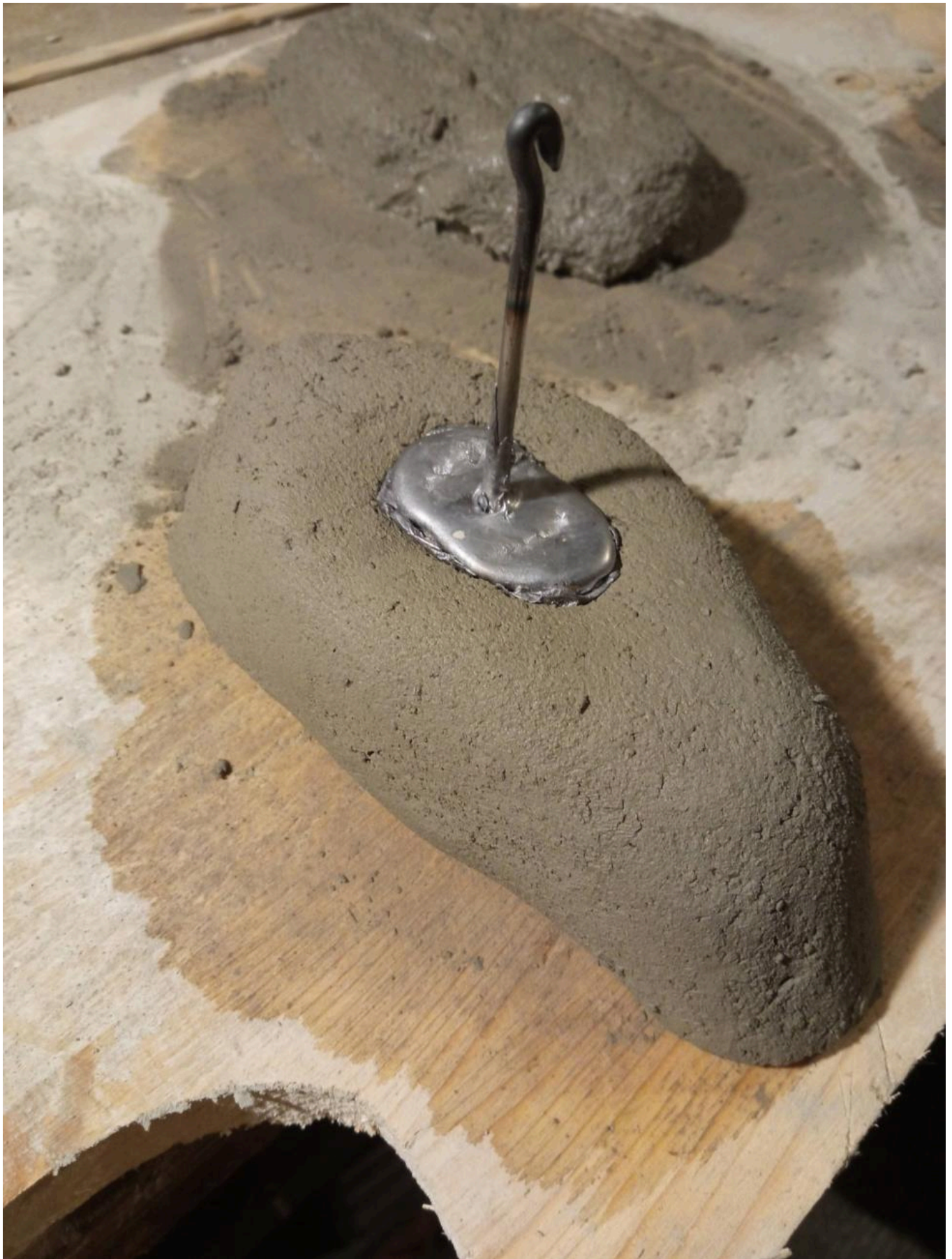
FIG 27. THE LEAD STAMP HAS BEEN USED TO MAKE MORE MOULDS MADE OF COMMERCIAL RED CLAY AND MARL TAKEN FROM SCHLIER BLOCKS NEAR GUBBIO, AMONG WHICH MF MAV-II IS SHOWN HERE. THE SECOND DAS STAMP HAS BEEN PUT INTO EACH HOLLOW TO TEST THEIR SIMILARITY WITH THE ORIGINAL HOLLOW. PHOTO BY MAURO FIORENTINI
