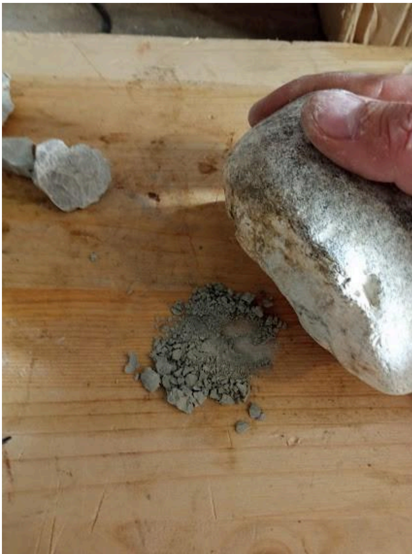
FIG 19. USING A STONE TOOL TO CRUSH AND PULVERIZE THE MARL FROM APIRO. PHOTO BY MAURO FIORENTINI
