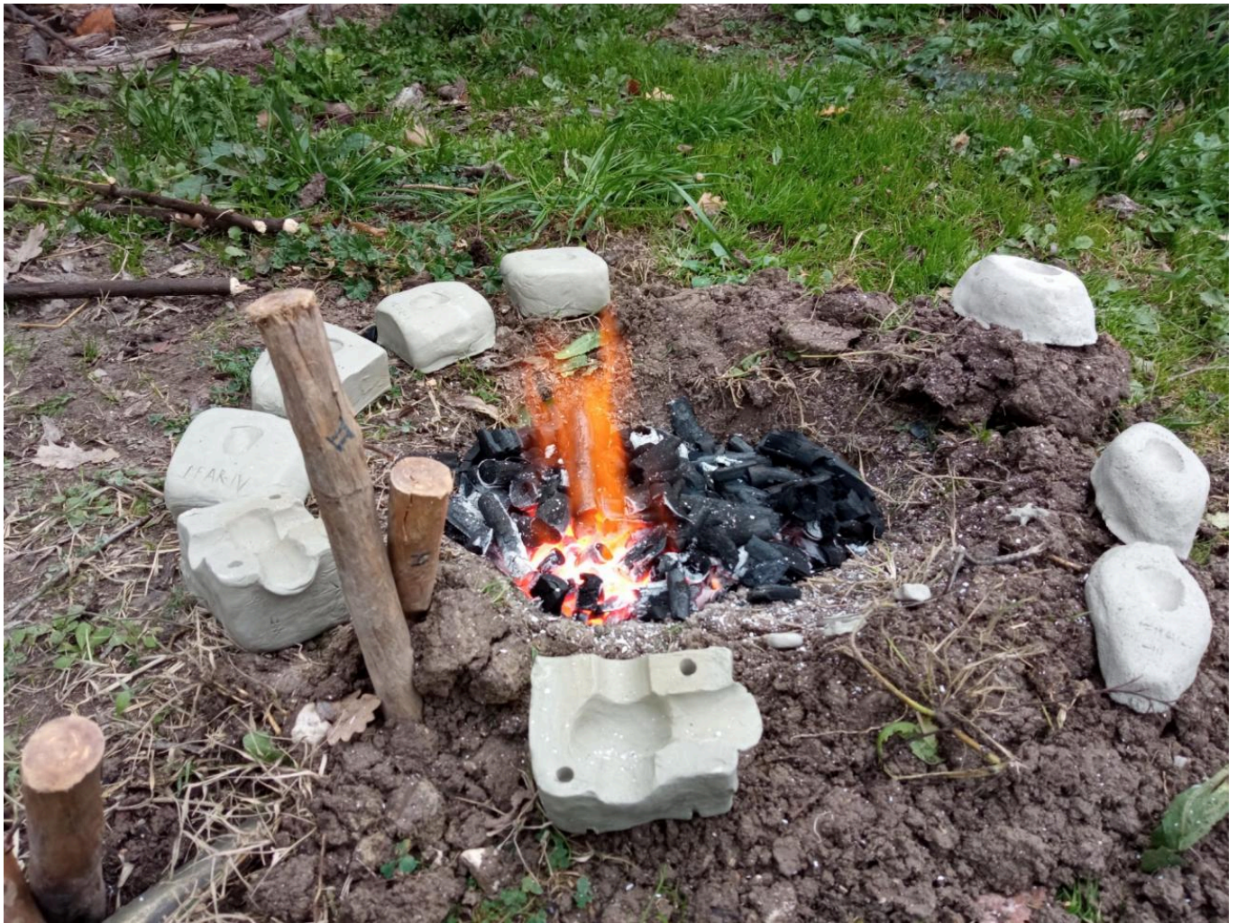
FIG 31. THE TRADITIONAL FORGE SETUP, CONSISTING IN A FIRE PIT WHERE HARDWOOD COAL WOULD BE FIRED AND HEATHEN UP USING A LEATHER BAG BELLOWS. CRUCIBLES AND THONGS, EITHER HISTORICAL REPLICAS AND MODERN BACKUPS, COMPLETE THE PLANT, TOGETHER WITH RECYCLED COPPER WIRE AND A MODERN BLOWTORCH TO IGNITE THE FIRE. SEVEN MOULDS ARE PUT AROUND THE PIT, TOGETHER WITH OTHER CLAY ITEMS THAT ARE NOT RELATED TO THE BAFFONI CAVE RESEARCH. PHOTO BY MAURO FIORENTINI
