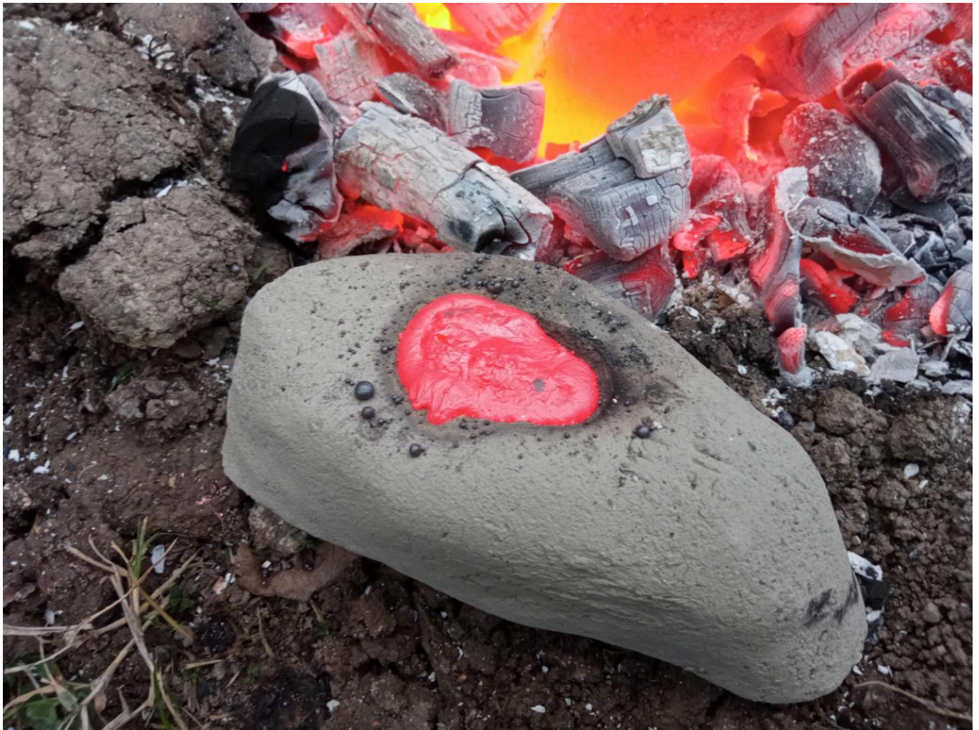
FIG 36. THE BACKUP CRUCIBLE, A MODERN ONE MADE OF GRAPHITE, WAS PUT IN THE FORGE AND FILLED OF COPPER. A SERIES OF THREE QUICK MELTINGS WERE SUCCESSFULLY PERFORMED, ALL USING MF MAV-II MOULD. DESPITE ITS TEMPERATURE BEING CONSTANTLY LOW (FIGURE 177), THE MOULD'S RESISTANCE TO THE THERMAL SHOCKS WAS OUTSTANDING, BEARING NO SIGNS OF DAMAGES AT THE END OF THE ACTIVITY. BOILING COPPER WAS A CONSTANT, HAVING HAPPENED AT EVERY CASTING. PHOTO BY MAURO FIORENTINI
