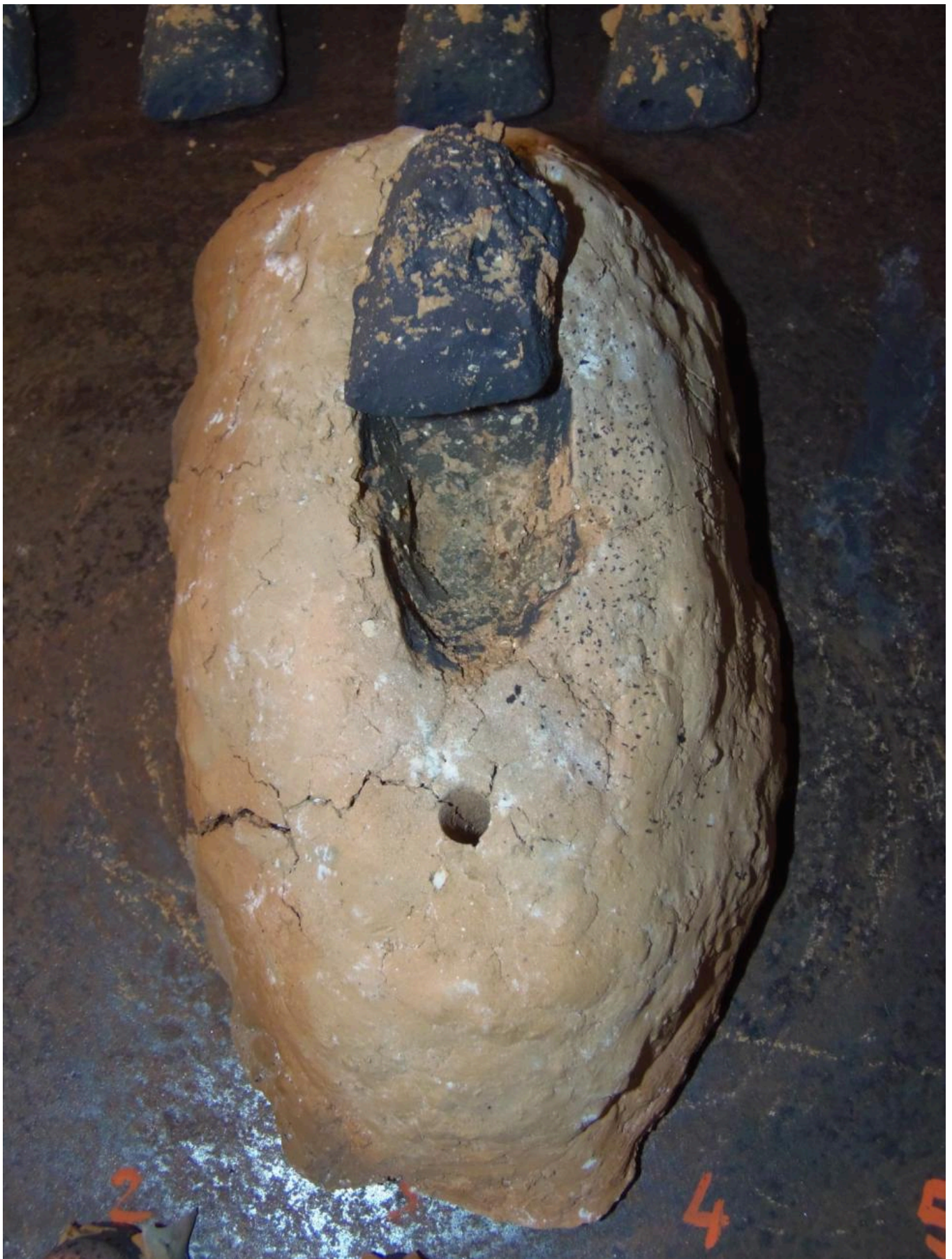
FIG 15. THIS PICTURE SHOW HOW THE HOLLOW OF MF-1 HAS WORN OUT AFTER FIVE CASTINGS. PHOTO BY MAURO FIORENTINI
