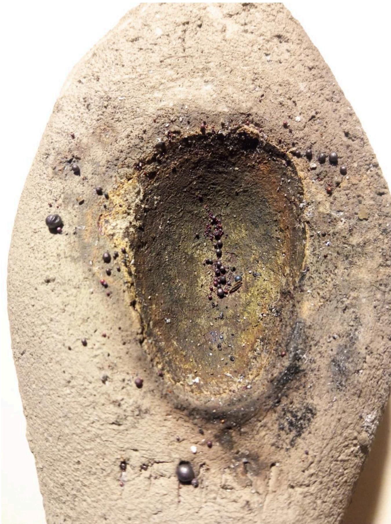
FIG 38. MF MAV-II WITH F4 PULLED OUT. DUE TO THE BOILING OF MELTED COPPER DURING THE CASTINGS, THE MOULD'S SURFACE IS COVERED WITH METAL SPHERES OF VARIOUS SIZES. THESE CAN STILL BE SEEN IN THE SPECIMEN'S SURFACE, WHICH VALIDATES THE HYPOTHESIS THAT IT WAS EITHER USED TO MELT METAL IN IT OR IT WAS PUT CLOSE TO A SOURCE OF BOILING METAL. THE COLOR OF MF MAV-II'S HOLLOW AFTER THREE CASTINGS CLOSELY RESEMBLES THAT OF THE SPECIMEN'S, SUGGESTING THAT THE LATTER WAS EFFECTIVELY USED AS A MOULD FOR COPPER OR COPPER ALLOY INGOTS. PHOTO BY MAURO FIORENTINI
