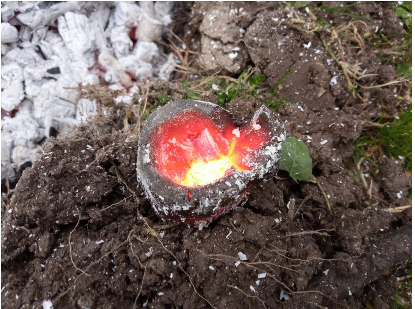
FIG 33. COPPER WIRES WERE PUT INTO THE MOSCOSI DI CINGOLI CRUCIBLE REPLICA, AND IT HAS BEN PUT INTO THE FIRE. ADDING COAL HELPED TO RISE THE TEMPERATURE... A BIT TOO MUCH, IN FACT THE CRUCIBLE MELTED AND THIS FIRST ATTEMPT AT MELTING THE METAL MUST BE CONSIDERED A FAILURE. PHOTO BY MAURO FIORENTINI
