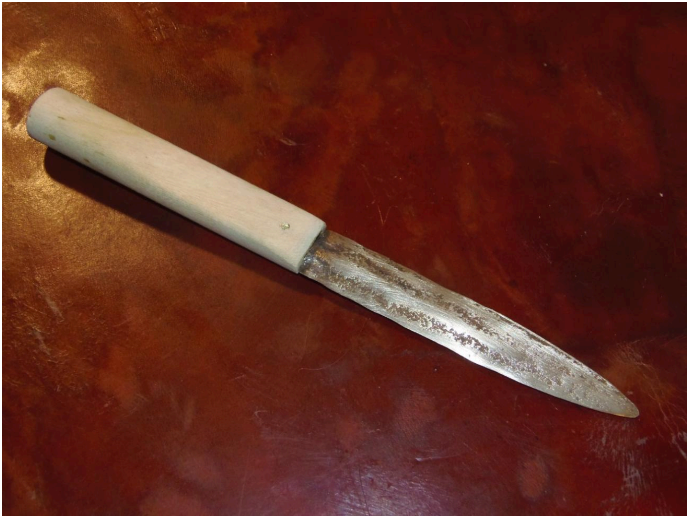
FIG 10. B-3 AFTER BEING POLISHED WITH THE WHETSTONE AND HAFTED. PHOTO BY MAURO FIORENTINI
