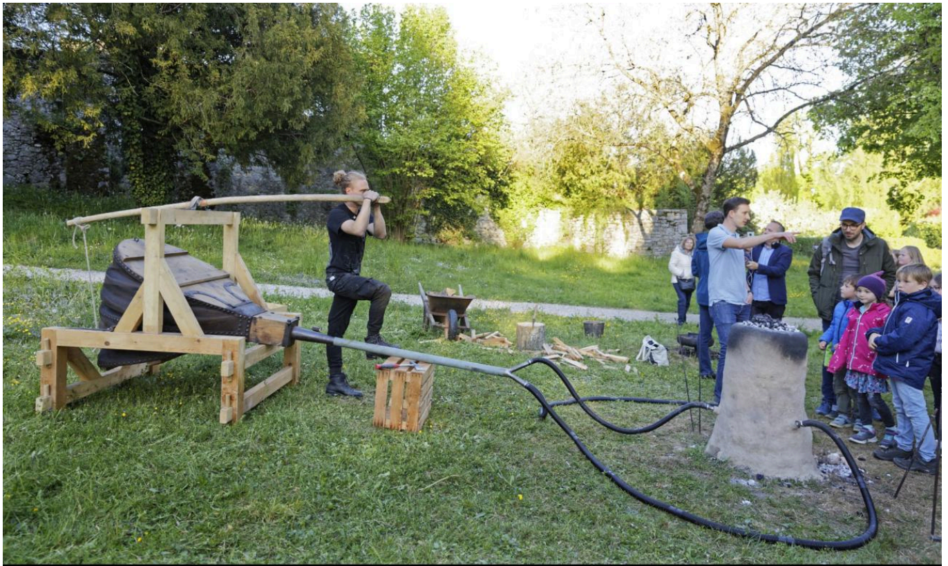
FIG 4. LIVE DEMONSTRATION OF A BLOOMERY BY UELI ZAHNER WITH BELLOWS FOR SMELTING IRON ORE AND (SUBSEQUENT) FURNACE OPENING. PHOTO BY IRIS KREBS
