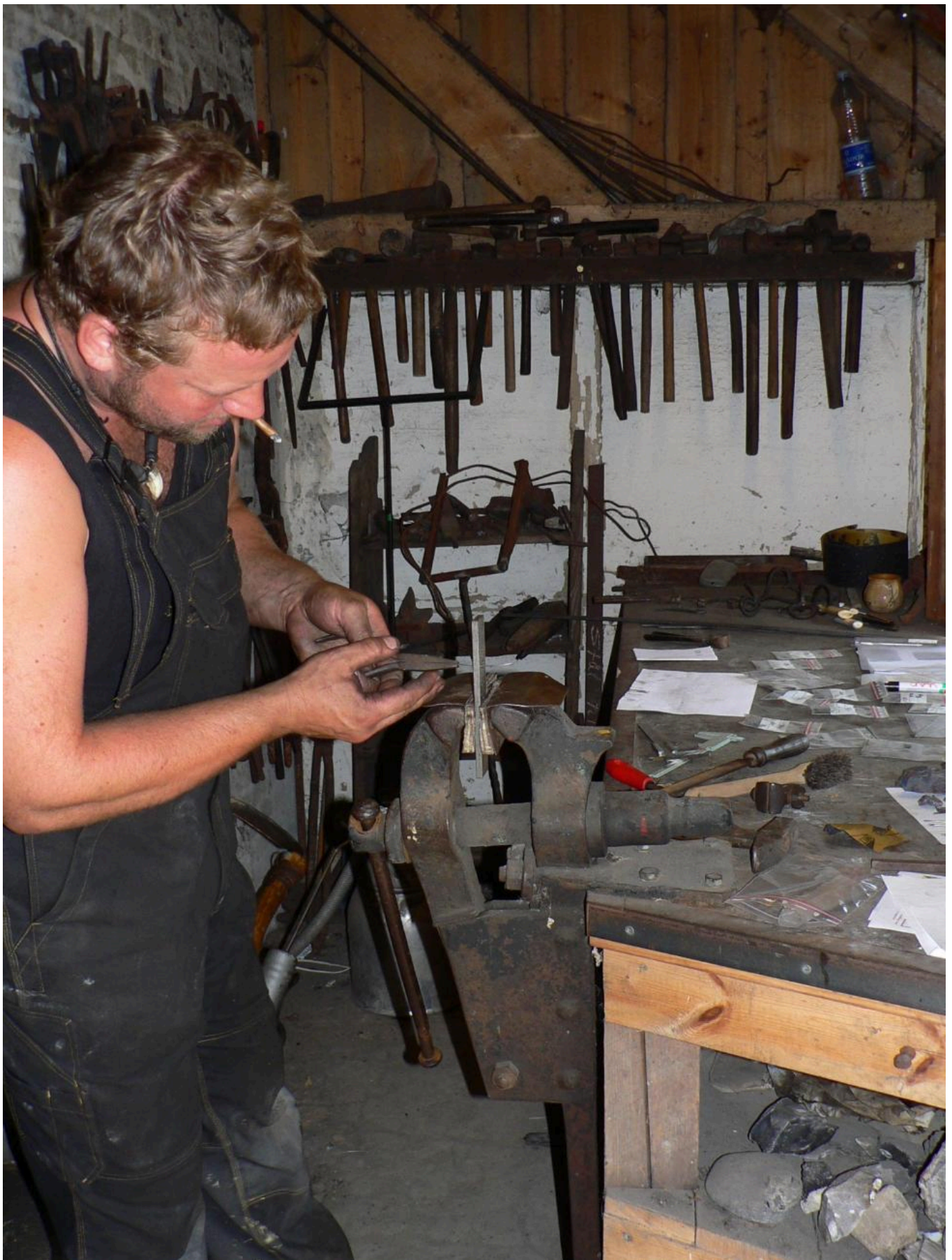
FIG 11. THE SMITH CAREFULLY ASSESSED THE QUALITY OF THE IRON WIRE BEFORE EACH DRAW. PHOTO BY H. LYGSTRØM
