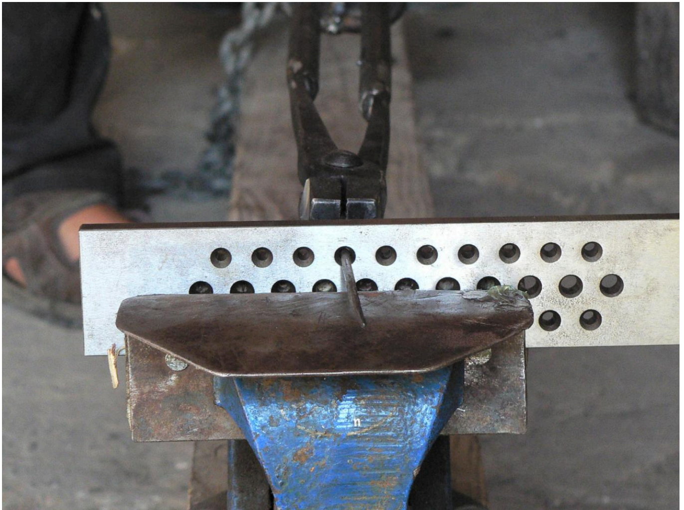
FIG 9. THE IRON FROM THE GULDFORHOVED BLOOM WAS STABLE WITHOUT MAJOR SLAG INCLUSIONS, BUT THE SMITH WAS NEVERTHELESS CAREFUL TO CUT OFF PARTS WITH MINOR SLAG INCLUSIONS. PHOTO BY H. LYGSTRØM
