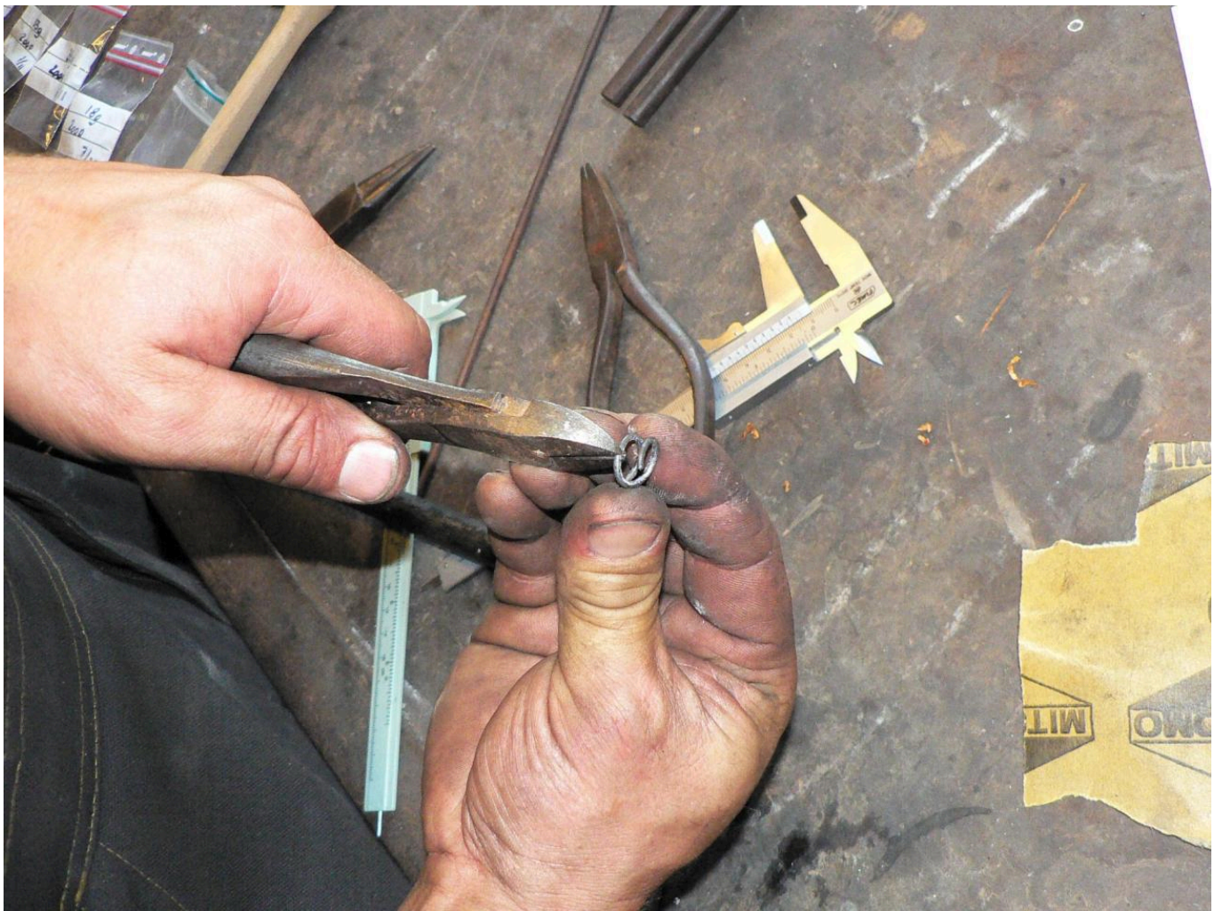
FIG 14. THE SPIRALS WERE CUT SO THEY OVERLAPPED SLIGHTLY. PHOTO BY H. LYGSTRØM
