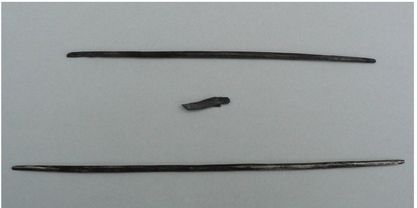
FIG 5. DESPITE THE POINTS BEING ANNEALED AND SUBSEQUENTLY FILED MANY RODS BROKE INTO SEVERAL PIECES DURING THE FIRST DRAW. PHOTO BY H. LYGSTRØM
