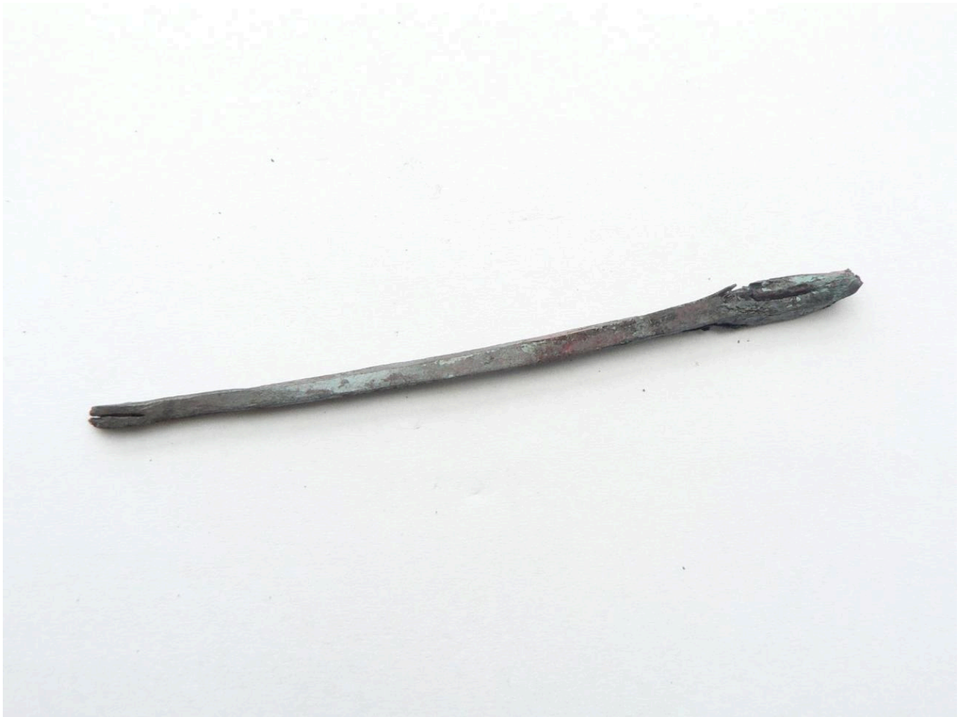
FIG 4. BOG ORE IRON ALWAYS CONTAINS SOME SLAG - AS VISIBLE IN THIS 11 CM LONG ROD MADE OF STORE DYREHAVE BOG ORE. PHOTO BY H. LYGSTRØM
