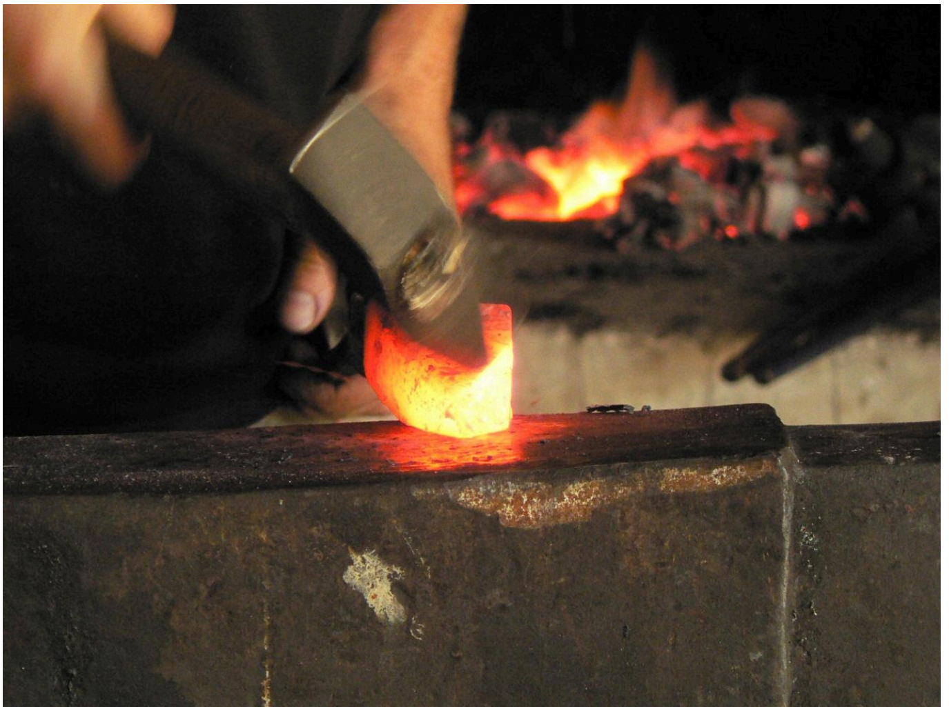
FIG 10. THE BILLET FROM THE IKAST BLOOM HAD A CONTENT OF LESS THAN 0.1% CARBON AND 0.3% PHOSPHORUS. PHOTO BY H. LYGSTRØM
