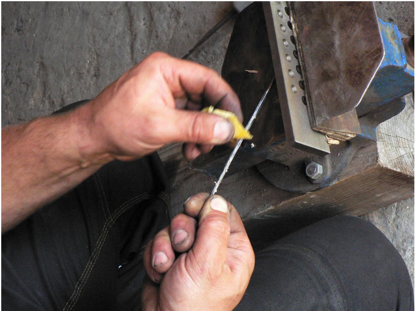
FIG 7. THE SMITHS DECIDED TO REDUCE THE FRICTION BY RUBBING THE WIRE WITH BEESWAX AFTER EACH ANNEALING AND FILING. PHOTO BY H. LYGSTRØM
