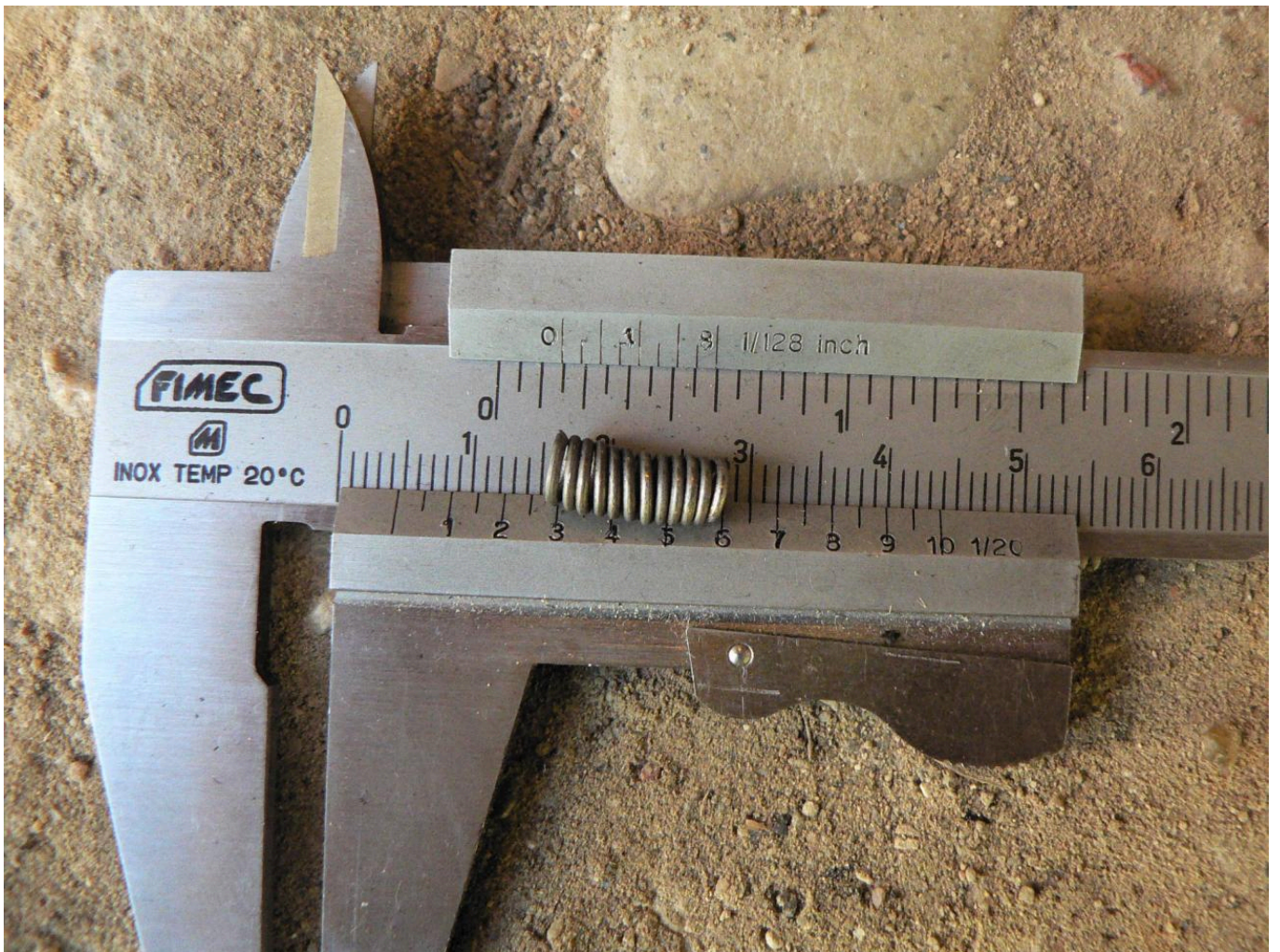
FIG 13. THE WIRE WAS EASILY WRAPPED TO A SPIRAL AROUND A MANDREL. THE SMALLEST MANDREL WE WRAPPED AROUND WAS 4 MM IN DIAMETER. PHOTO BY H. LYGSTRØM
