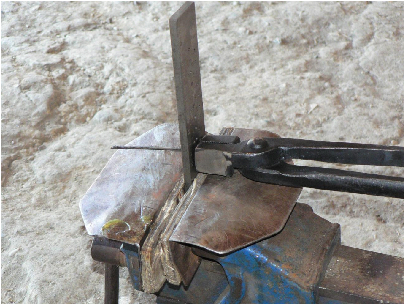
FIG 8. A PAIR OF PLIERS WITH SERRATED JAWS PROVIDED A SIGNIFICANTLY BETTER GRIP DURING DRAWING. PHOTO BY H. LYGSTRØM
