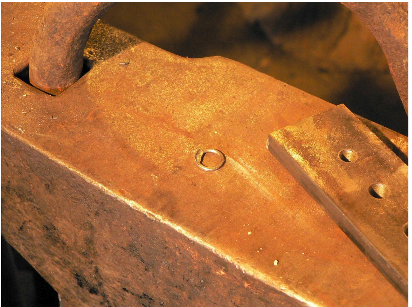
FIG 15. AFTER CUTTING THE RINGS WERE STRUCK TOGETHER WITH A HAMMER. THE SOFT IRON ADHERED EASILY WITHOUT HEATING. PHOTO BY H. LYGSTRØM
