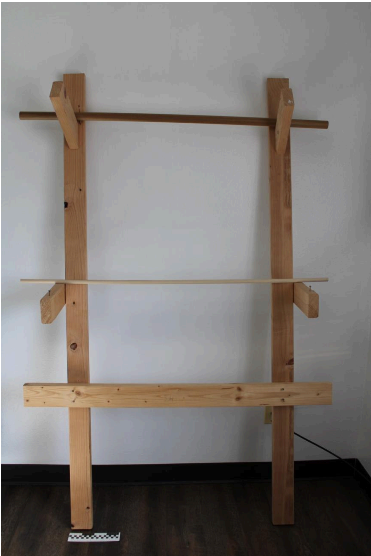
FIG 4. THE WARP WEIGHTED LOOM CONSTRUCTED FOR THESE EXPERIMENTS. PHOTO BY VICTORIA PRIOLA.
