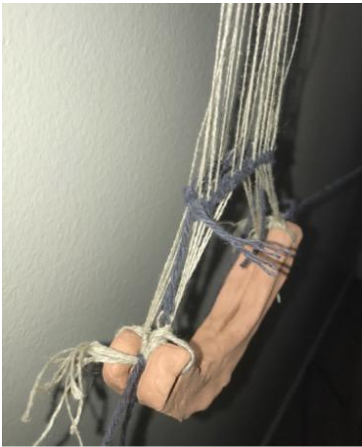
FIG 7. THE THIN CRESCENTS PROVIDED VERY LITTLE SEPARATION BETWEEN THE TWO SHEDS IN BAND WEAVING. PHOTO BY VICTORIA PRIOLA.
