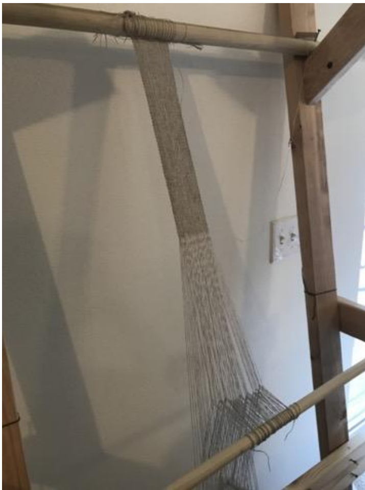
FIG 16. THE COUNTER SHED CREATED BY THE HEDDLE BAR FOR WARP WEIGHTED WEAVING. PHOTO BY VICTORIA PRIOLA.
