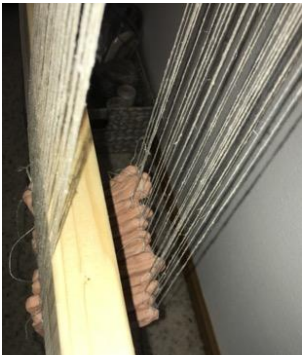
FIG 15. THE NATURAL SHED CREATED BY THE CRESCENTS FOR WARP-WEIGHTED WEAVING. PHOTO BY VICTORIA PRIOLA.
