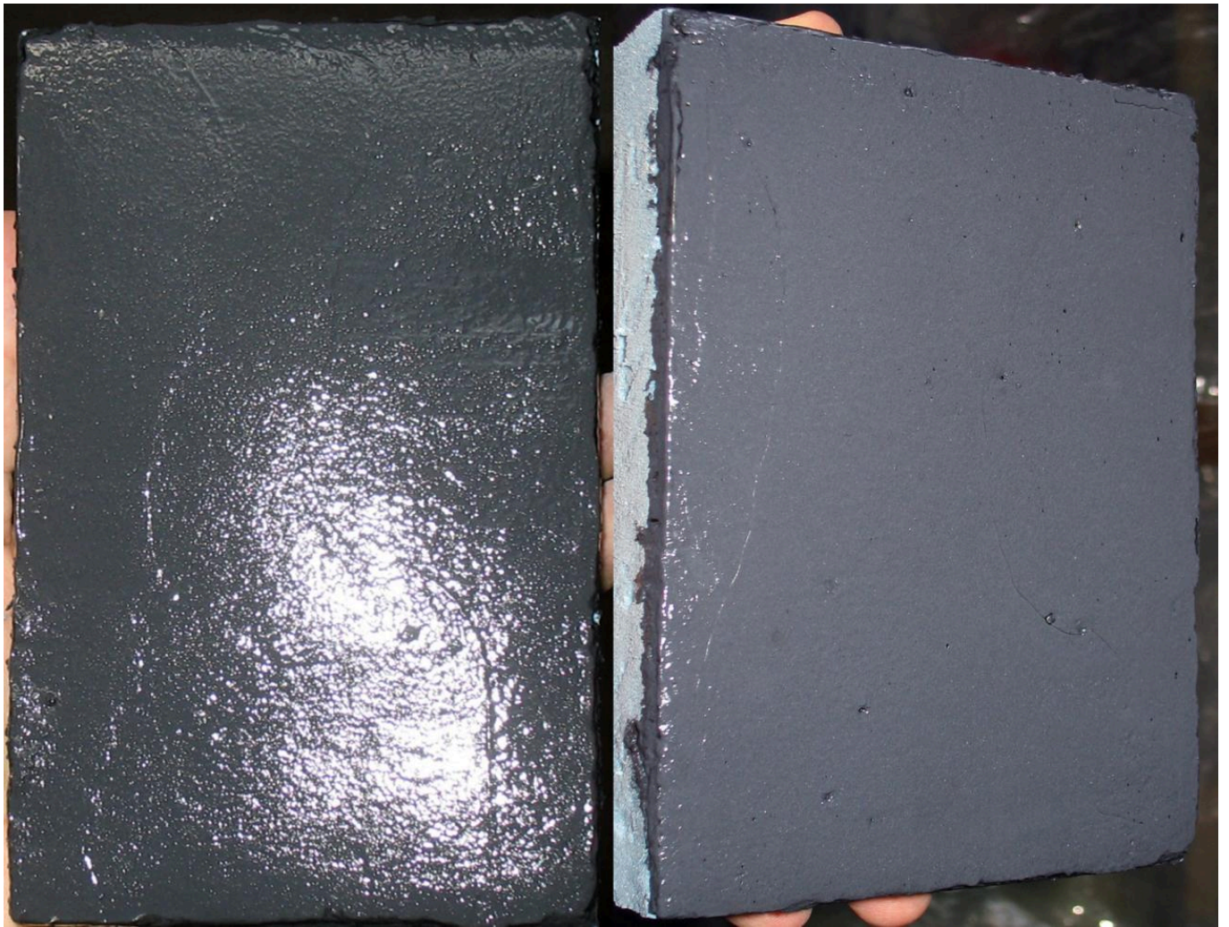
FIG 22. SAMPLE 1914 AINEIABOX. ON THE LEFT IS THE FRESH SAMPLE. ON THE RIGHT PICTURE IS THE SAMPLE PHOTOGRAPHED AT AN ANGLE 40 MINUTES LATER. NOTE THE HOLES FROM PUNCTURING THE BLISTERS. PHOTO BY ANTONIS VLAVOGILAKIS
