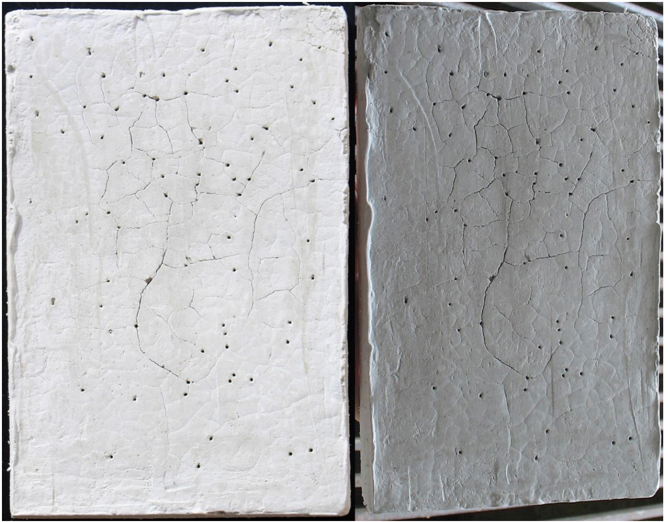
FIG 3. SAMPLE 15513 ASH. THE SURFACE OF THE SAMPLE WAS PHOTOGRAPHED AT DIFFERENT ANGLES TO SHOW THE SURFACE TEXTURE AND THE EXTENT OF THE CRACKING. PHOTO BY ANTONIS VLAVOGILAKIS
