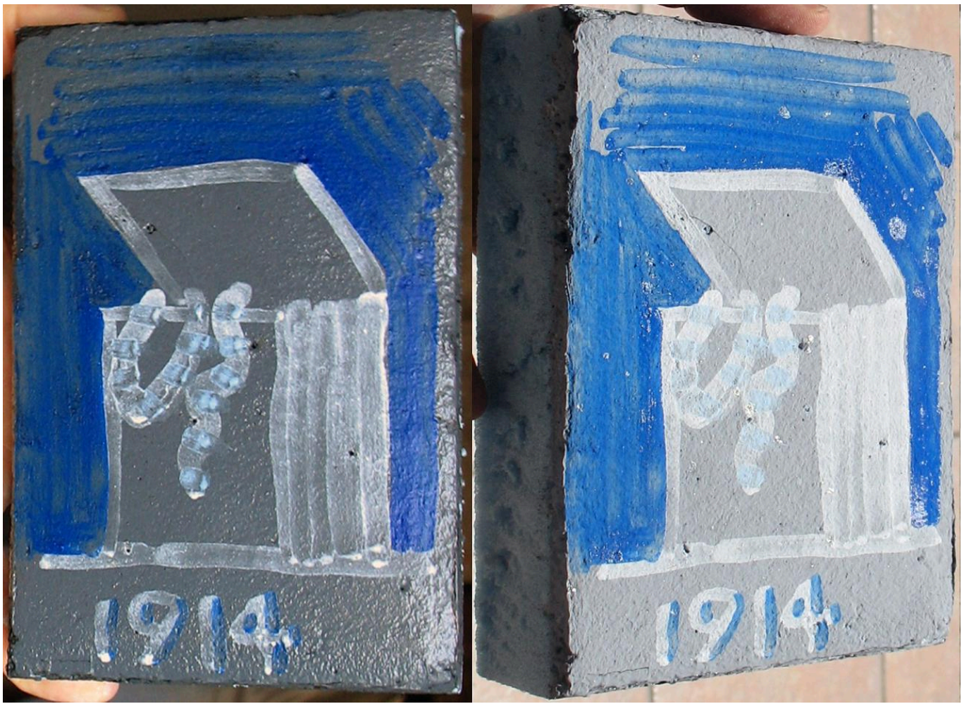
FIG 23. SAMPLE 1914 AINEIABOX. ON THE LEFT IS THE FRESH SAMPLE. ON THE RIGHT IS THE SAMPLE PHOTOGRAPHED TWO DAYS LATER. NOTE THE GLOSSY STAINS THAT APPEARED IN VARIOUS PARTS OF THE SURFACE. PHOTO BY ANTONIS VLAVOGILAKIS
