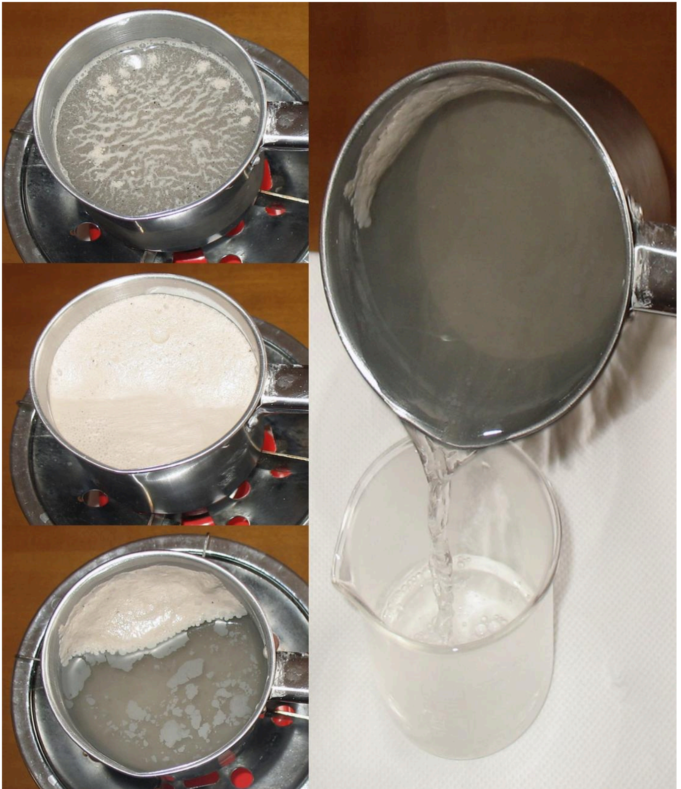
FIG 15. ON THE LEFT TOP PICTURE, THE ASH AND WATER MIXTURE IS STARTING TO HEAT. IN THE MIDDLE LEFT PICTURE MIXTURE IS CLOSE TO BOILING AND IS STARTING TO FOAM. THE BOTTOM LEFT PICTURE IS TAKEN AFTER THE MIXTURE HAS BOILED AND SOME MOST OF THE FOAM HAS BEEN REMOVED. ON THE RIGHT, THE LYE PRODUCED IS DRAINED TO A GLASS CONTAINER. NOTE THE ASH THAT HAS ACCUMULATED ON THE BOTTOM OF THE METAL POT. PHOTO BY ANTONIS VLAVOGILAKIS
