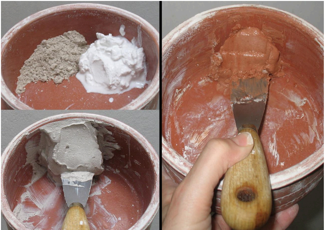
FIG 7. SAMPLE 14613-13913 ASH MIXTURES. ON THE PICTURES ON THE LEFT THE PREPARATION OF THE ASH AND LIME MIXTURE. ON THE RIGHT IS THE LIME, ASH, AND BRICK POWDER MIXTURE. PHOTO BY ANTONIS VLAVOGILAKIS
