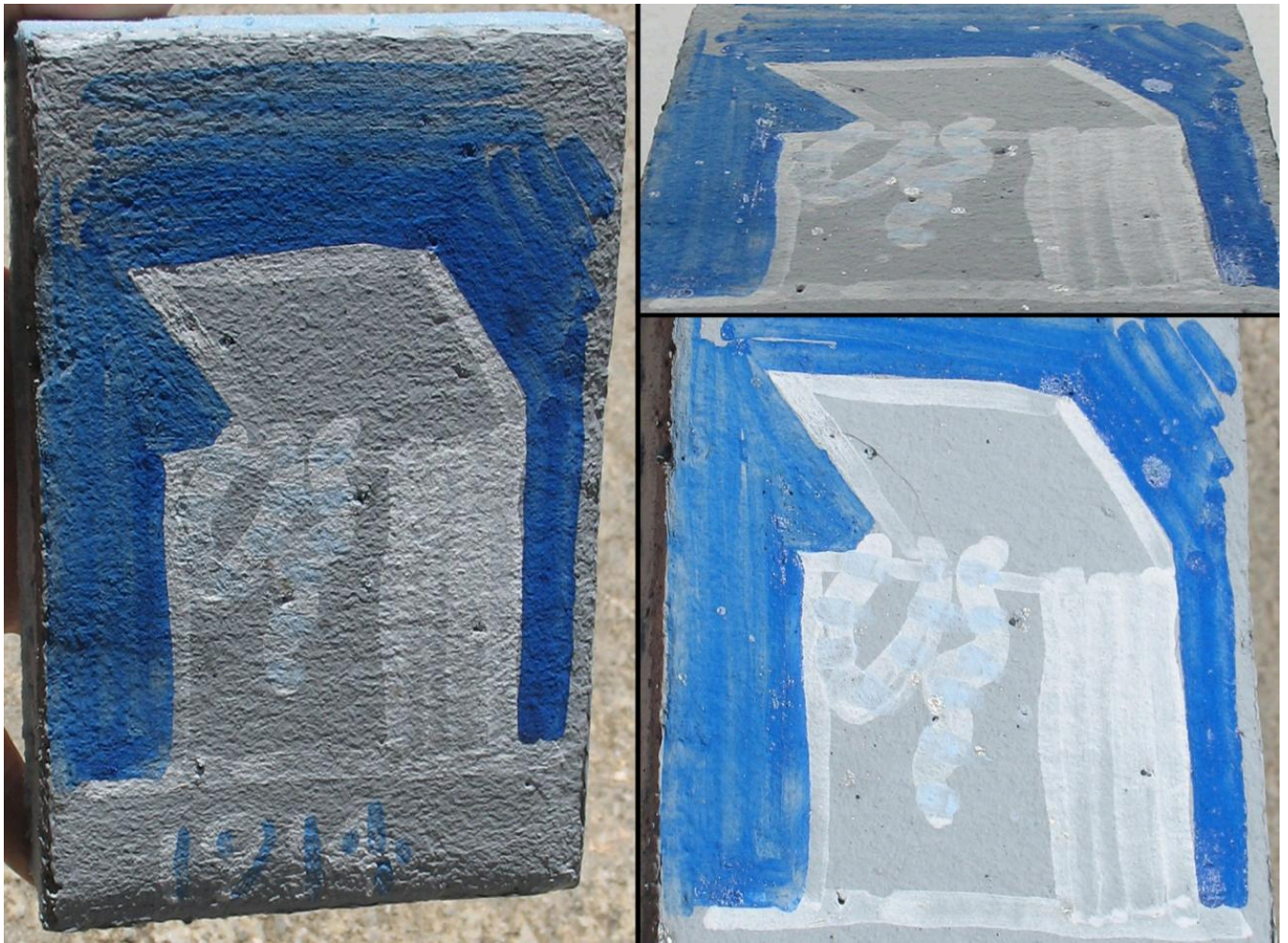
FIG 24. SAMPLE 1914 AINEIABOX. THREE PHOTOGRAPHS OF THE DRY SAMPLE WERE TAKEN AT DIFFERENT ANGLES. NOTE THE SURFACE TEXTURE ON THE LEFT PICTURE AND THE GLOSSY STAINS ON THE PICTURES ON THE RIGHT. PHOTO BY ANTONIS VLAVOGILAKIS
