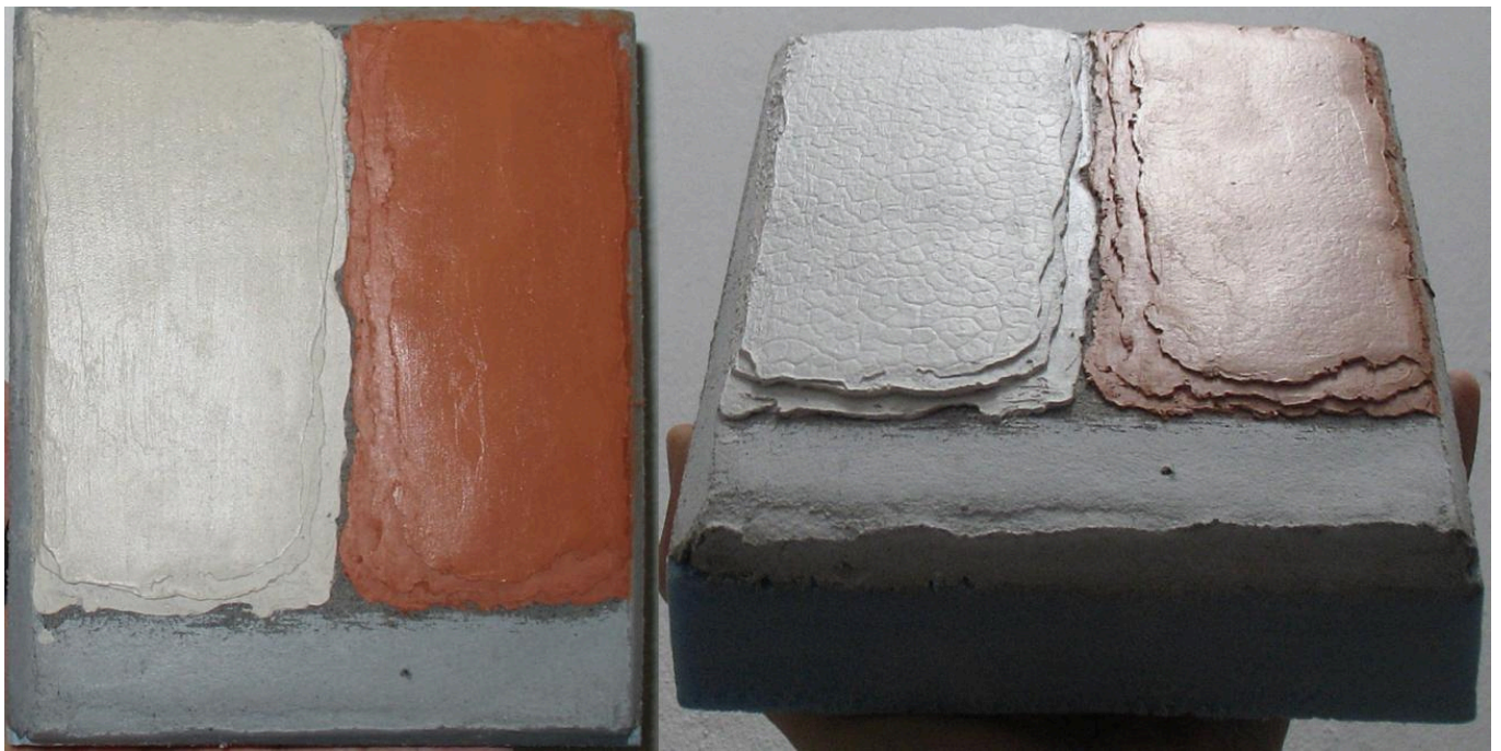
FIG 9. SAMPLE 14613-13913 ASH. ON THE LEFT IS THE FRESH SAMPLE. ON THE RIGHT, THE SAMPLE WAS PHOTOGRAPHED TWO DAYS LATER. NOTE THE DIFFERENCE IN THE SURFACE TEXTURE BETWEEN THE DOSES OF 2A AND 2B IN BOTH PICTURES. PHOTO BY ANTONIS VLAVOGILAKIS
