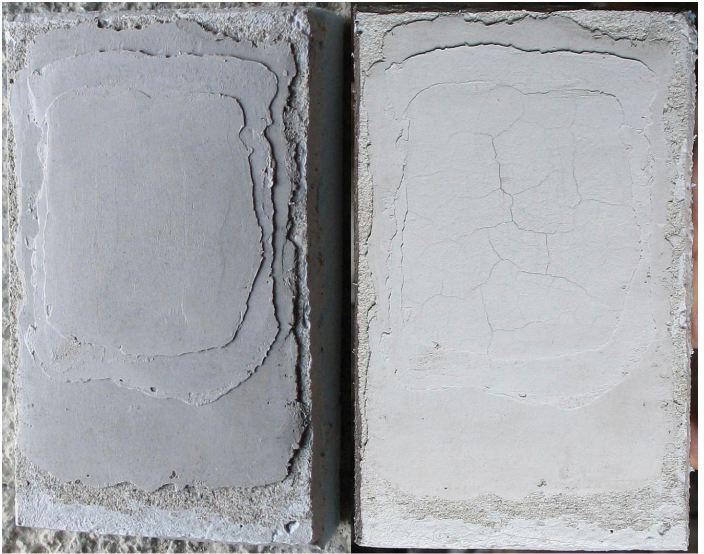
FIG 17. SAMPLE 281113 ASH. ON THE LEFT PICTURE IS THE FRESH SAMPLE. ON THE RIGHT IS THE SAMPLE PHOTOGRAPHED TWO DAYS LATER SHOWING THE CRACKS. PHOTO BY ANTONIS VLAVOGILAKIS
