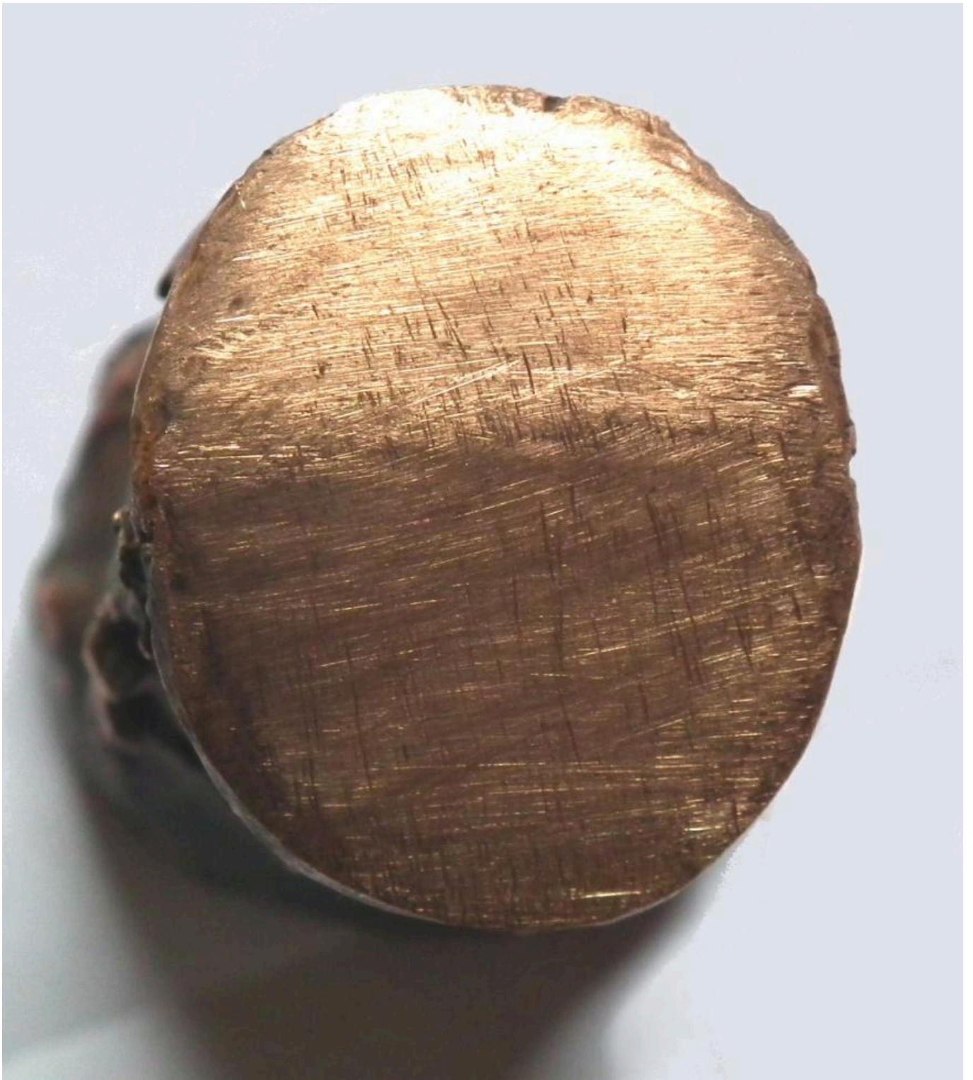
FIG 9. FINE SCRATCHES CAN BE SEEN ON THE FACE OF THE HAMMER AFTER SANDING WITH GRITSTONE. LARGER SCRATCHES CAN BE SEEN UNDERNEATH THE FINER ONES, ILLUSTRATING THE PROCESS OF STARTING WITH A COARSER ABRASIVE AND CONTINUING WITH A FINER ONE.
