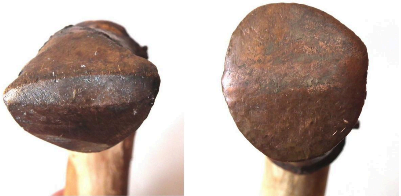
FIG 10. EVIDENCE OF HANDEDNESS IN WEAR: BEFORE USE BOTH OF THESE HAMMERS HAD SYMMETRICAL FACES. THE HAMMER ON THE LEFT SHOWS MORE WEAR ON THE PROPER LEFT (THE HAMMER'S LEFT) OF THE HAMMER, WHERE THE APEX IS WIDER AND MORE FLATTENED THAN ON THE PROPER RIGHT. ON THE OTHER HAMMER, THE UPPER PROPER RIGHT OF THE HAMMER IS FLATTENED AND DISTORTED (INCLUDING BURRING) AND THE APEX IS MORE FLATTENED ON THAT SIDE.
