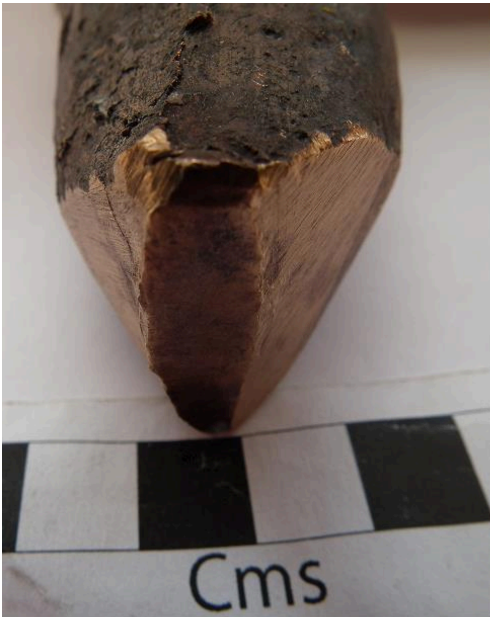
FIG 8. BEFORE USE THE HAMMER FACE WAS WEDGE-SHAPED. AFTER USE THE PEAK OF THE WEDGE IS FLATTENED AND BURRING CAN BE SEEN ALONG THE TOP EDGE OF THE FACE (ON THE LEFT).
