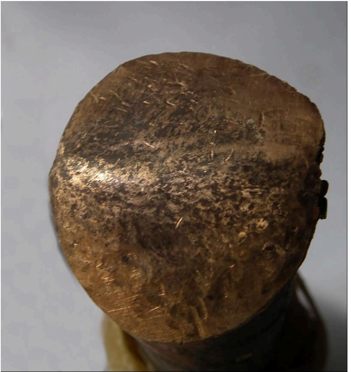
FIG 7. HAMMER FACE AFTER USE WITH A CHISEL.
