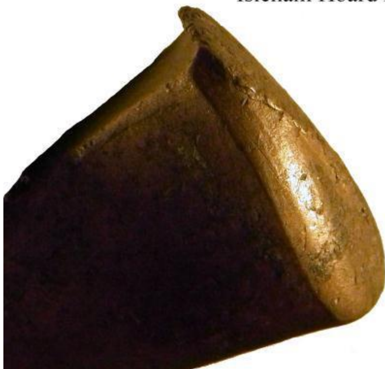
FIG 5. AN EXAMPLE OF A BURRED HAMMER FACE (COURTESY OF ST EDMUNDSBURY HERITAGE SERVICE).
