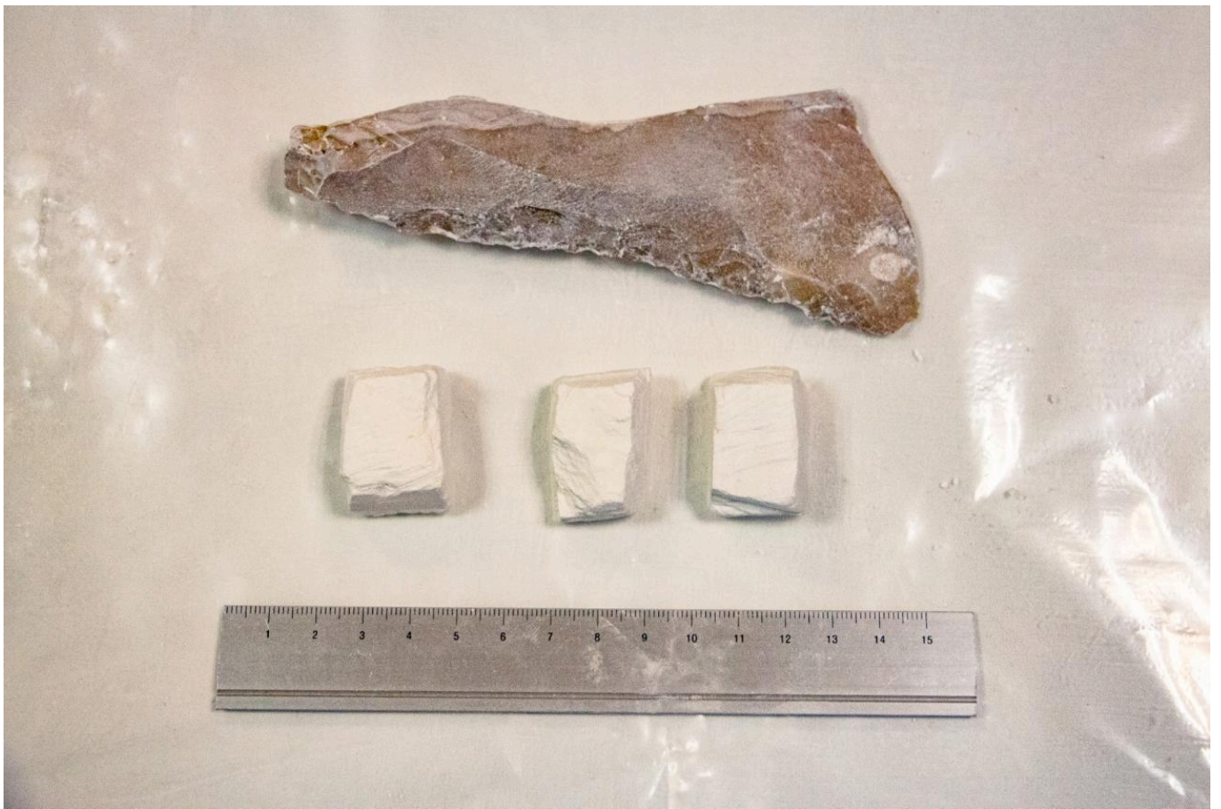
FIG 3. FINAL STEATITE BLOCKS, READY FOR DRILLING. PHOTO BY NOAM KODESH
