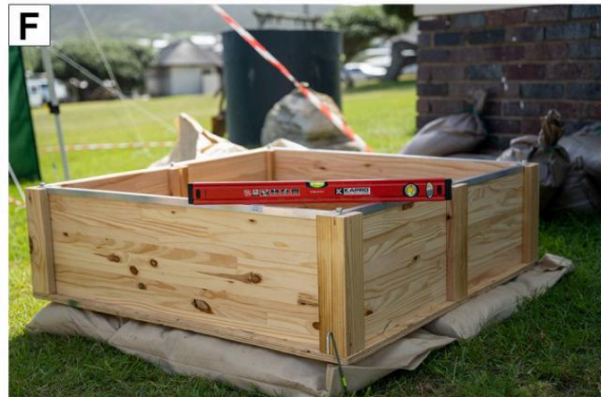
FIG 5. SETTING UP EXPERIMENTAL BOXES A) MAIN ELEMENTS OF AN EXPERIMENTAL BOX (DISASSEMBLED); B) ASSEMBLING OF AN EXPERIMENTAL BOX; C) POSITION OF EXPERIMENTAL BOXES INSIDE EXPERIMENTAL CAMP AREA; D) CLOSE-UP VIEW OF AN EXPERIMENTAL BOX; E) PUTTING SANDBAGS ON THE GROUND TO LEVEL THE SURFACE BELOW THE BOXES; F) BOX LEVELLED. PHOTOS BY MAGNUS HAALAND. COMPILED BY MAGNUS HAALAND
