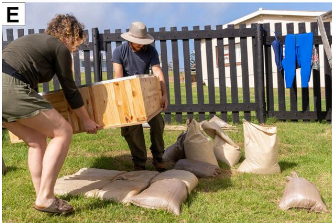
FIG 5. SETTING UP EXPERIMENTAL BOXES A) MAIN ELEMENTS OF AN EXPERIMENTAL BOX (DISASSEMBLED); B) ASSEMBLING OF AN EXPERIMENTAL BOX; C) POSITION OF EXPERIMENTAL BOXES INSIDE EXPERIMENTAL CAMP AREA; D) CLOSE-UP VIEW OF AN EXPERIMENTAL BOX; E) PUTTING SANDBAGS ON THE GROUND TO LEVEL THE SURFACE BELOW THE BOXES; F) BOX LEVELLED. PHOTOS BY MAGNUS HAALAND. COMPILED BY MAGNUS HAALAND
