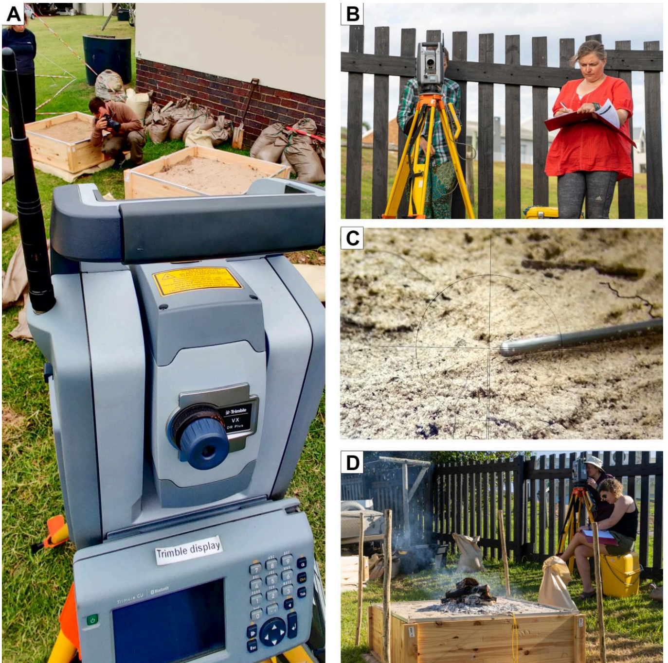
FIG 6. SPATIAL SETUP AND RECORDING OF THE EXPERIMENTAL AREA AND BOXES USING A TOTAL STATION : A) PERSPECTIVE OF THE TOTAL STATION OVERLOOKING THE EXPERIMENTAL CAMP; B) OPERATION OF THE TOTAL STATION; C) LOCATING A COORDINATE THROUGH THE OBJECTIVE (LENS) OF TOTAL STATION; D) LOCATION OF THE TOTAL STATION IN RELATION TO THE EXPERIMENTAL FIRE. PHOTOS BY MAGNUS HAALAND AND OLE F. UNHAMMER. COMPILED BY MAGNUS HAALAND
