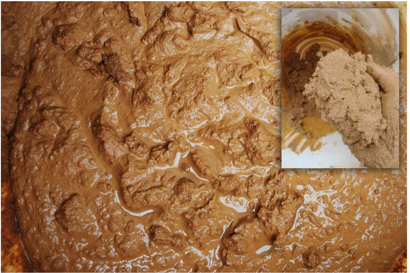
FIG 4. PHOTOGRAPHS TAKEN TO SHOW THE TEXTURE OF BEFORE THE ADDITION OF SAND (LEFT) AND AFTER (RIGHT). PHOTO BY BRIANNA JENKINS
