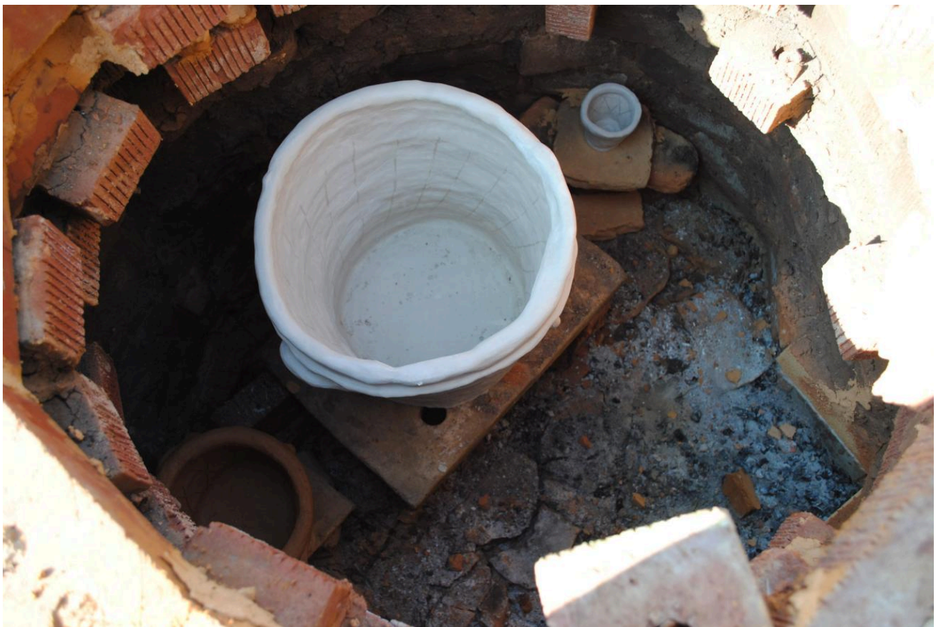
FIG 13. DEPICTS THE LOCATION OF THE CERAMIC VESSELS INSIDE THE KILN UPON THE FIRINGS. PHOTO BY BRIANNA JENKINS
