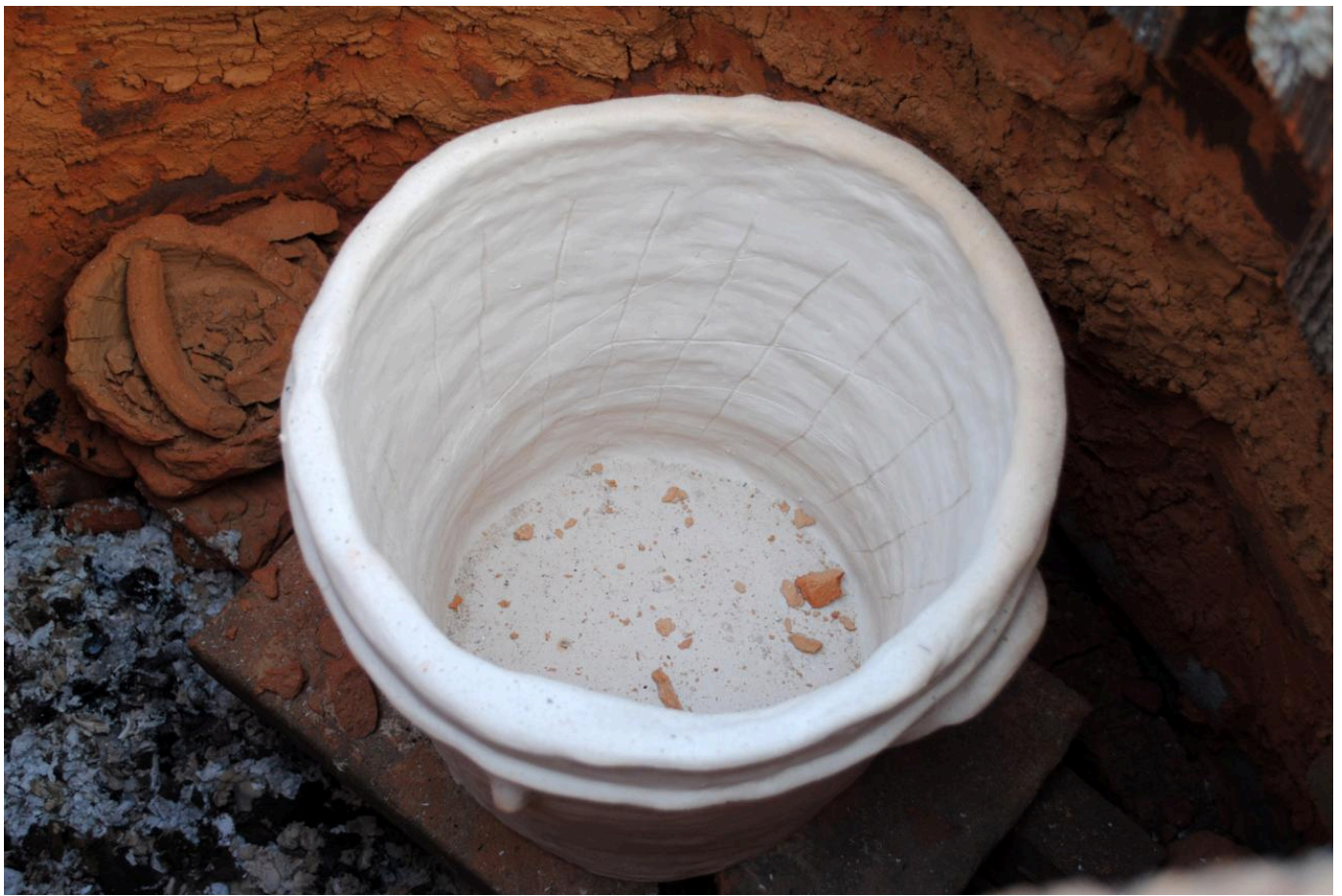
FIG 14A. THE FINAL RESULT OF THE KILN AFTER FIRING WAS UNSUCCESSFUL. THE LARGE VESSEL DID NOT REACH TEMPERATURE AND THE RED LOCAL CLAY PILOT TEST ENDED UP BREAKING. PHOTO BY BRIANNA JENKINS
