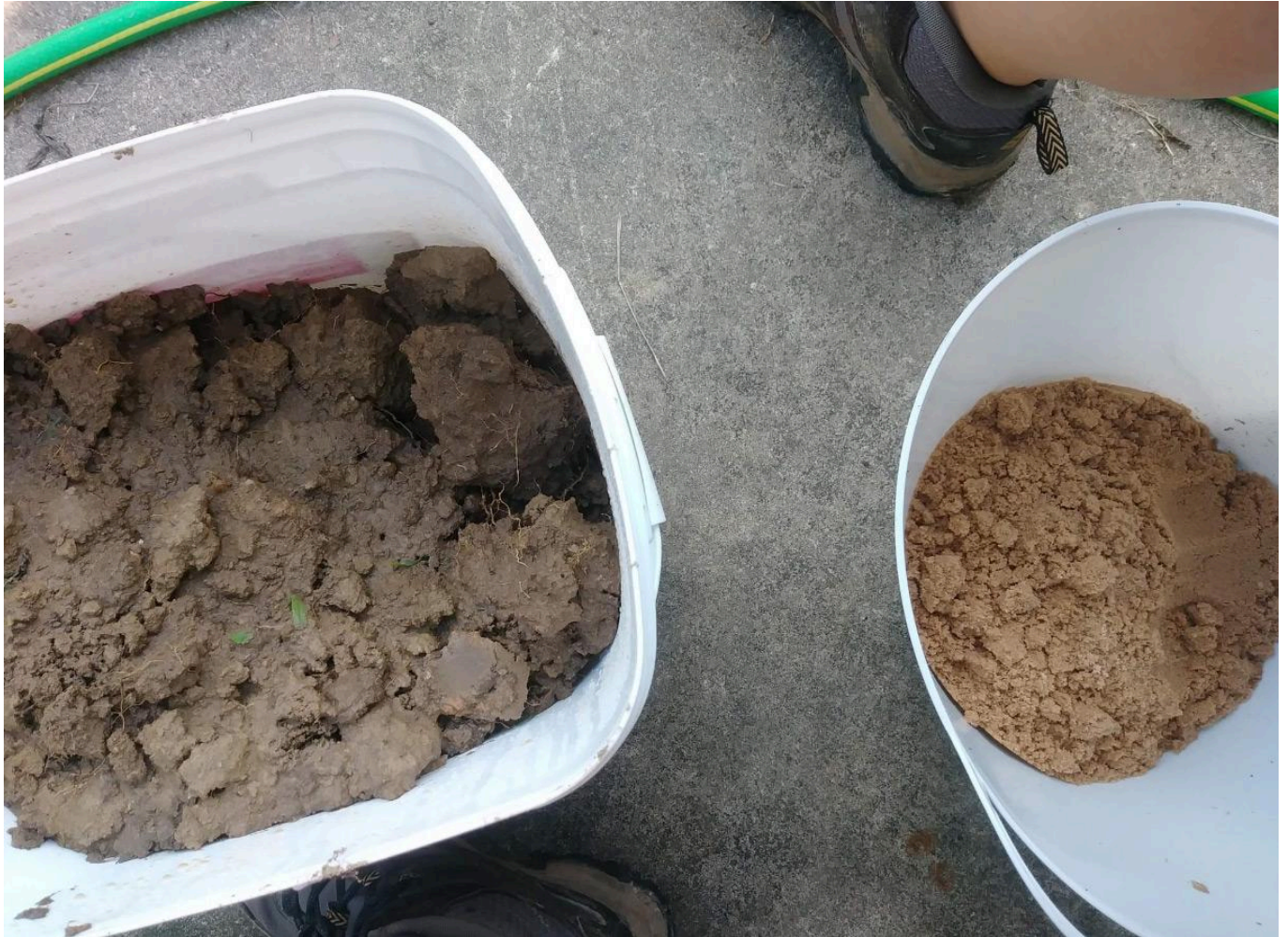
FIG 3. DEPICTS THE COLOR OF THE CLAY USED FOR THE PILOT TEST IN MUDBRICKS, AS WELL AS THE SAND. PHOTO BY BRIANNA JENKINS
