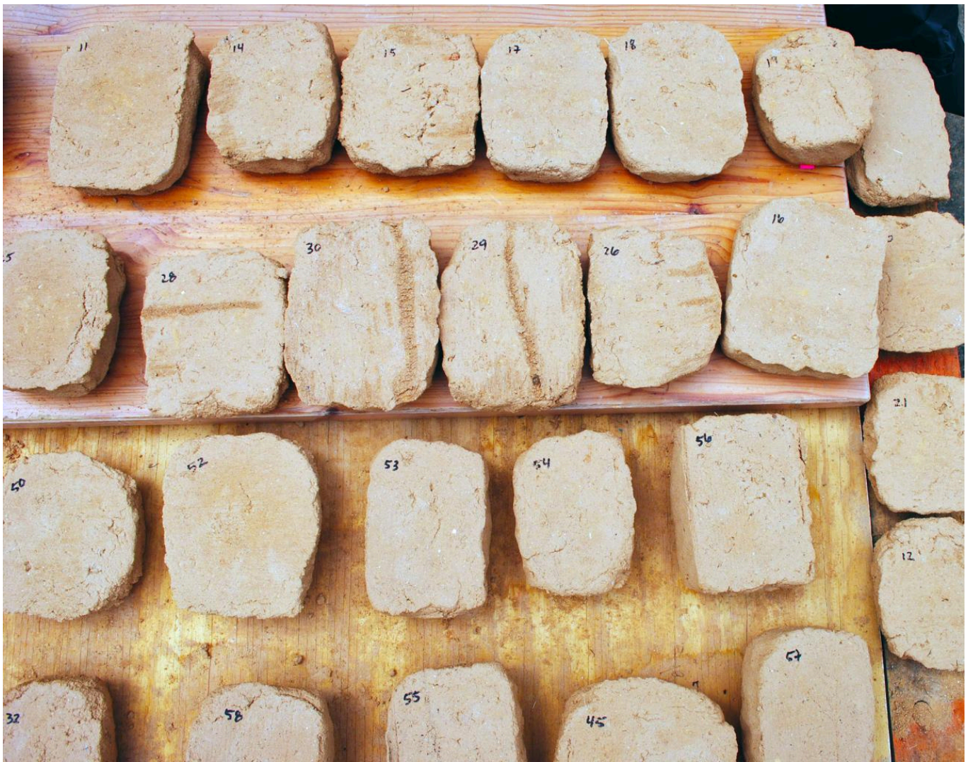
FIG 5. THE FINAL MUDBRICKS HAD BEEN LEFT TO SUNBAKE AND AWAIT THE KILN CONSTRUCTION. PHOTO BY BRIANNA JENKINS
