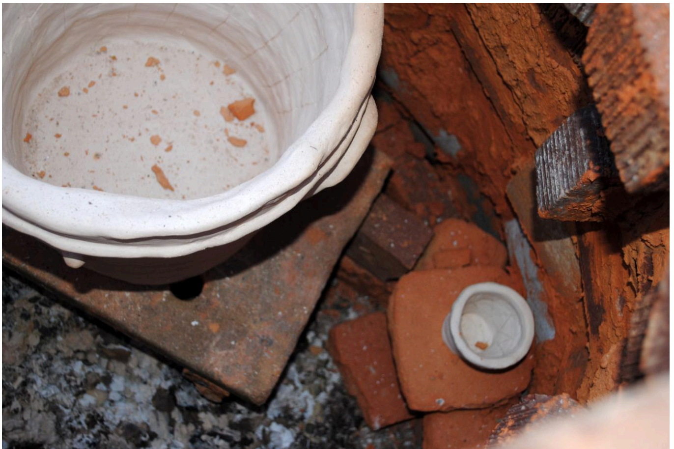
FIG 14B. THE FINAL RESULT OF THE KILN AFTER FIRING WAS UNSUCCESSFUL. THE LARGE VESSEL DID NOT REACH TEMPERATURE AND THE RED LOCAL CLAY PILOT TEST ENDED UP BREAKING. PHOTO BY BRIANNA JENKINS
