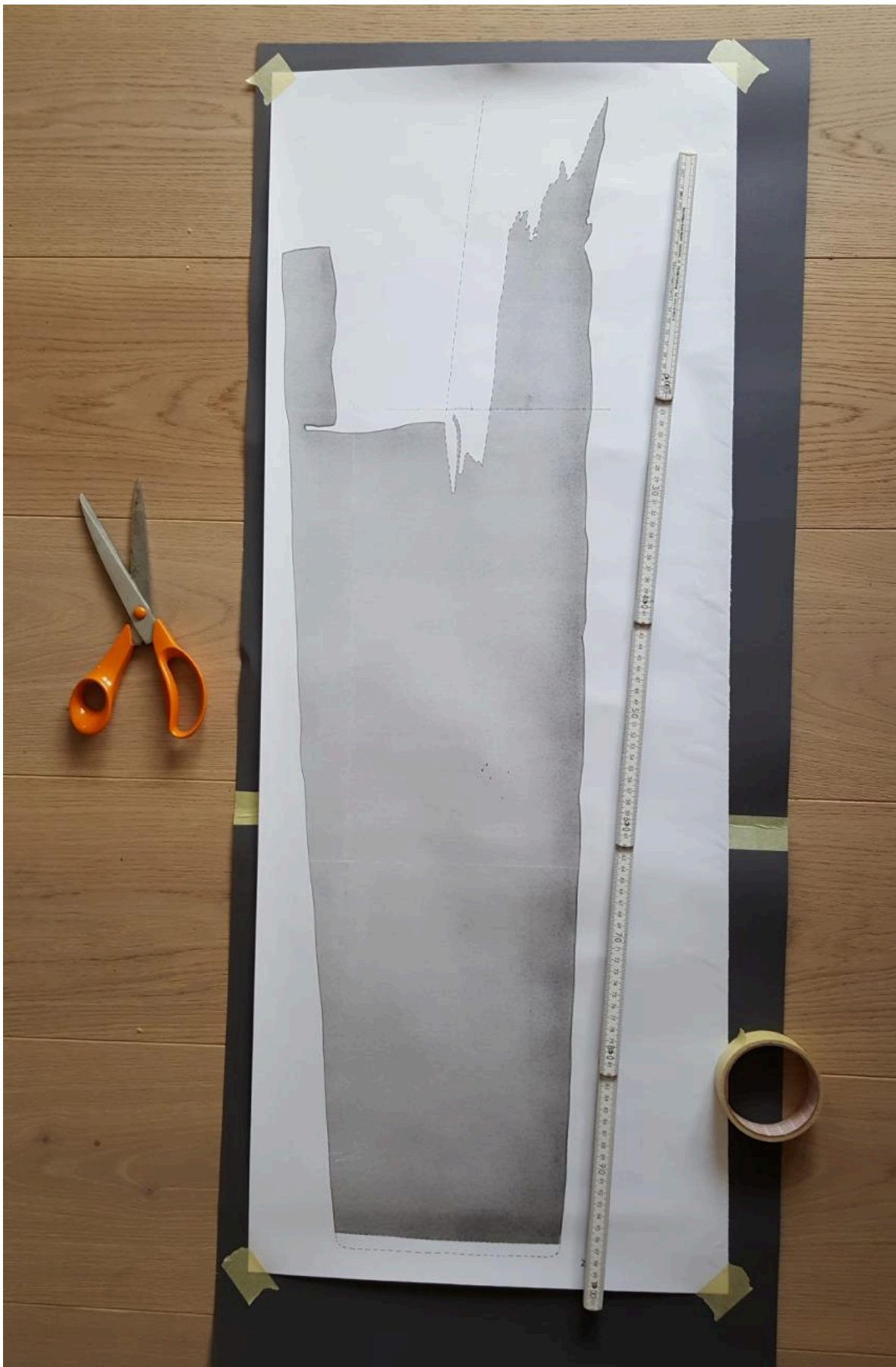
FIG 9. CREATION OF THE PATTERN. AN ENLARGED SCAN OF THE TECHNICAL DRAWING (EGG, APPENDIX 8) WAS PLACED ON RIGID CARDBOARD. THE CALCULATED 2.5 CENTIMETERS ARE THEN ADDED TO THE WIDTH. PHOTO BY MARKUS KLEK
