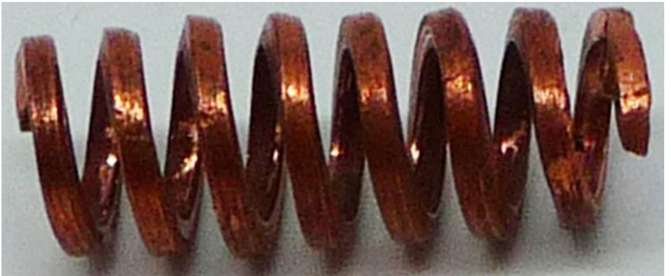
FIG 10. COIL OPENED TO THE CORRECT PITCH. PHOTO BY DAVID SIM
