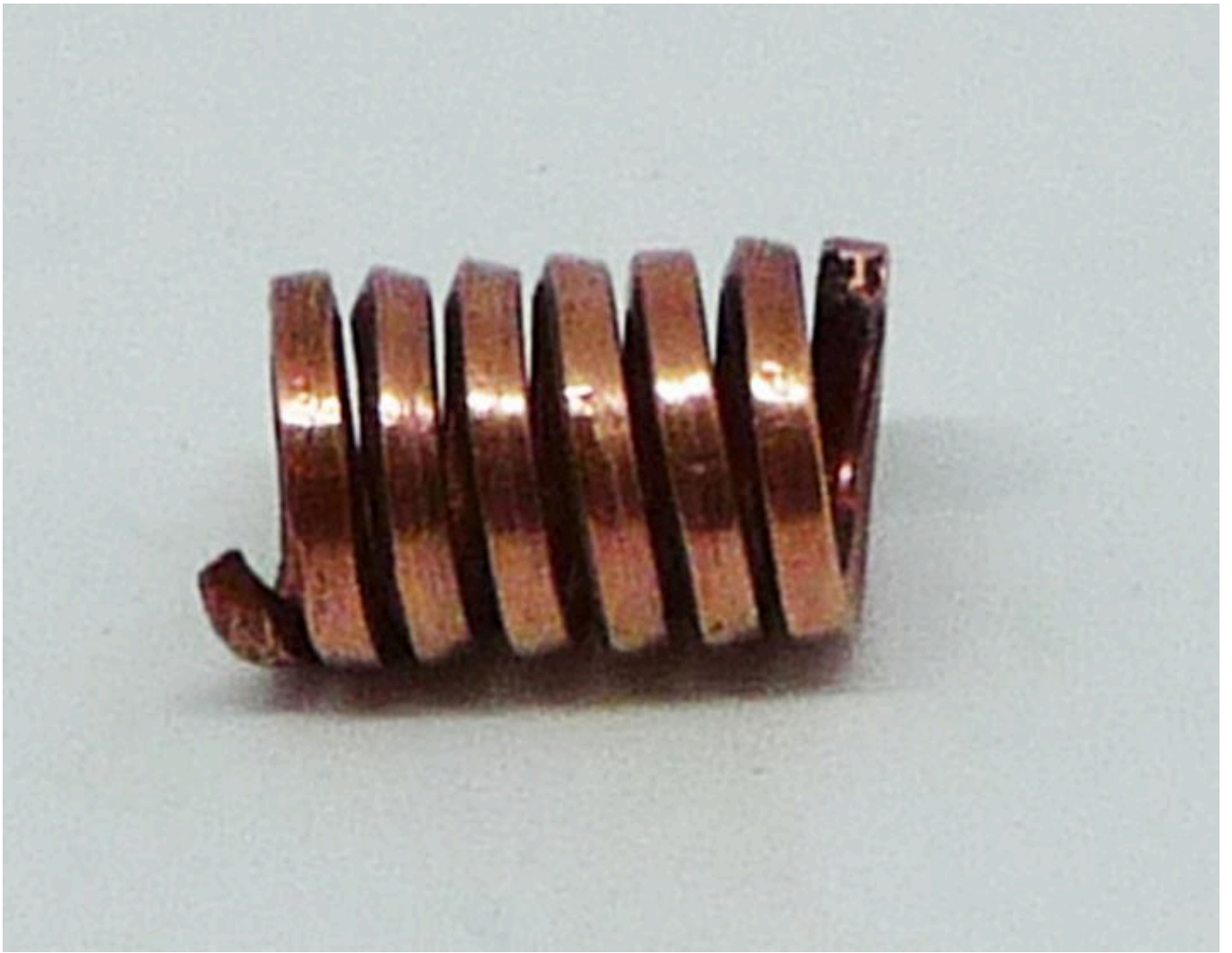
FIG 9. COIL WOUND ON A ROD. PHOTO BY DAVID SIM
