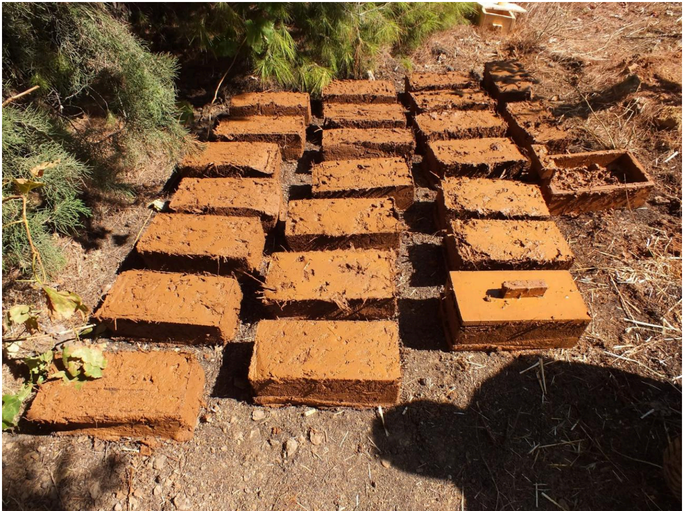
FIG 12. FINISHED MUDBRICKS WITH THE MOULD (CENTRE RIGHT) AND ITS LID THAT ALLOWED FOR EASIER PRESSING OF THE BRICK FROM THE MOULD (ON BOTTOM RIGHT BRICK).
