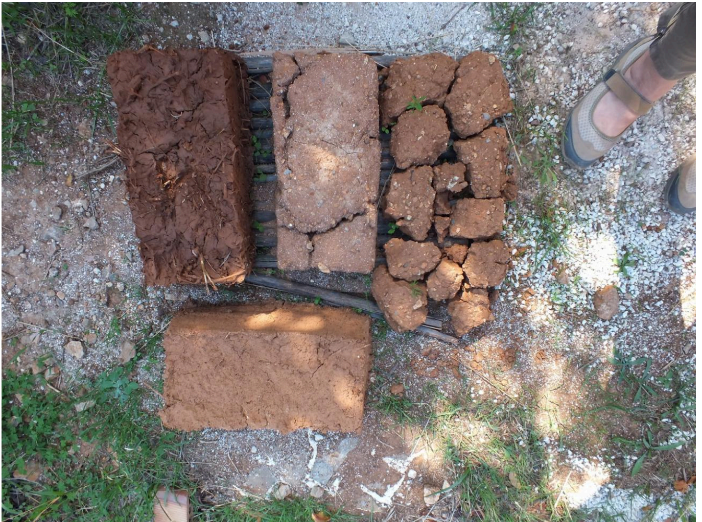
FIG 4. TEST BRICKS (FROM TOP LEFT): STRAW, SAND, PLAIN, PINE NEEDLES (CA. 4 WEEKS OLD)
