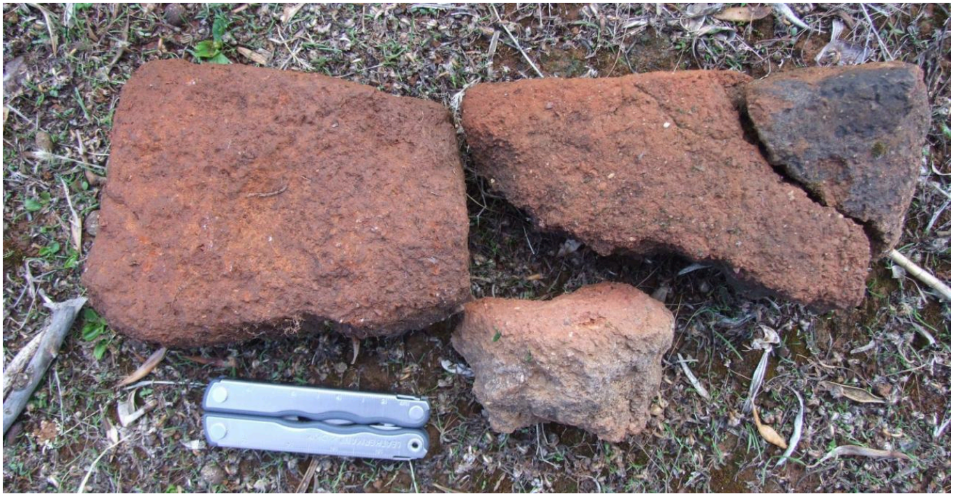
FIG 1. ACCIDENTALLY FIRED FRAGMENTS OF MUDBRICK AT A MIDDLE MINOAN SITE – NOTE THE DIFFERENCES IN COLOUR
