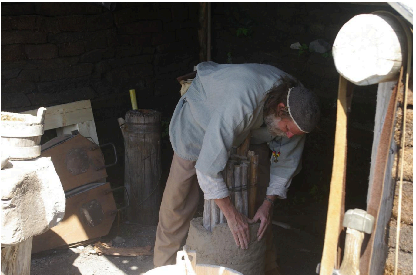
FIG 1. DARRELL MARKEWITZ ADDING MORE COB TO THE SMELTER DURING CONSTRUCTION. A BUNDLE OF STICKS WAS USED TO PROVIDE AND INTERNAL SMELTER FORM. (PHOTO: KELLY PROBYN-SMITH)
