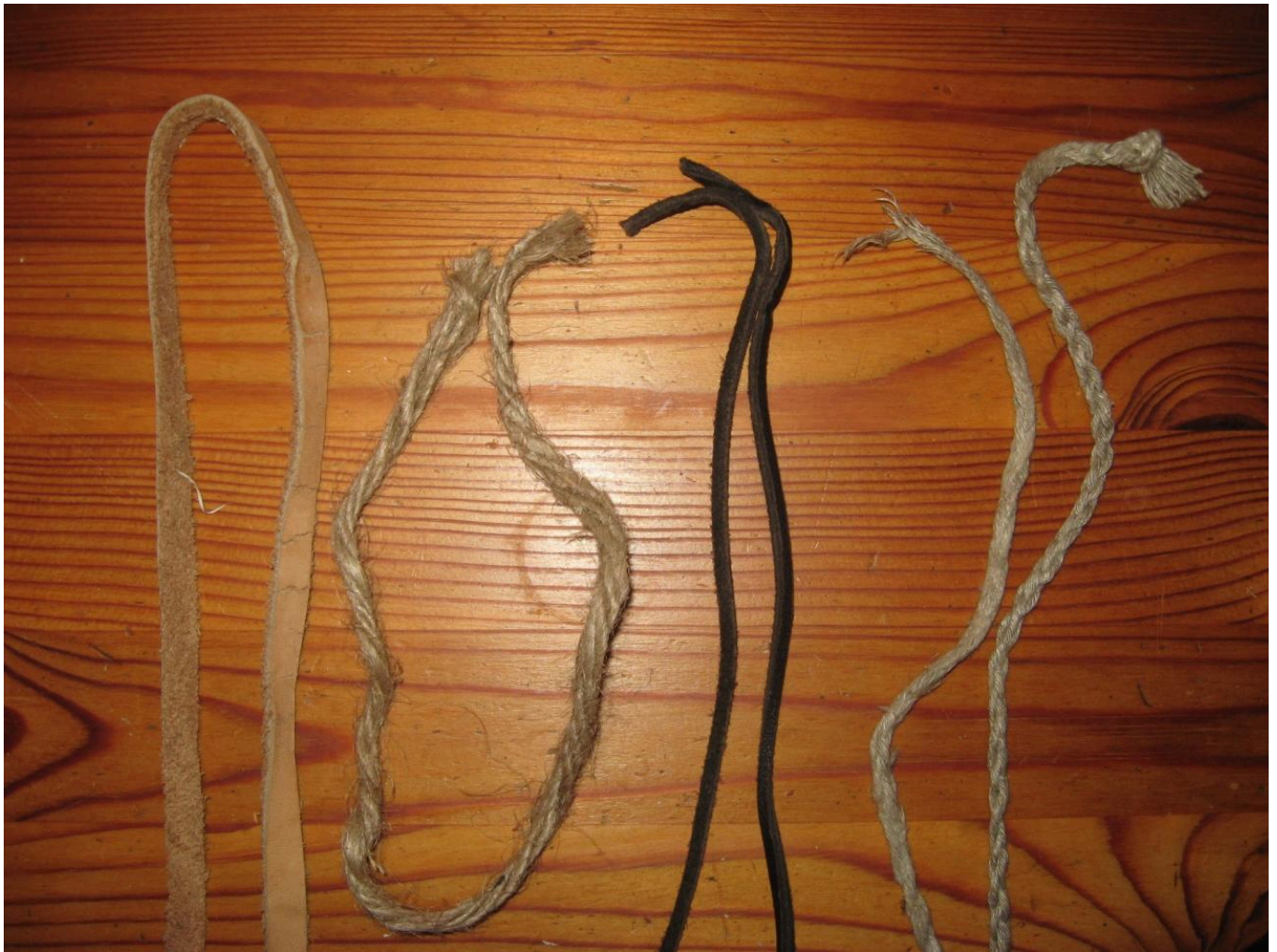
FIG 19. MATERIALS USED FOR POLE LATHE DRIVE CORDS. LEFT TO RIGHT: 1CM SOFT CHROME TANNED LEATHER, SINGLE PLY NATURAL JUTE TWINE, LATIGO LACE, AND 4-STRAND HEMP CORD. ON HEMP CORD, LEFT HAND SIDE SHOWS WEAR AND FINAL FAIL DURING USE, RIGHT HAND SIDE SHOWS ORIGINAL TEXTURE. (PHOTO: MARCUS BURNHAM)
