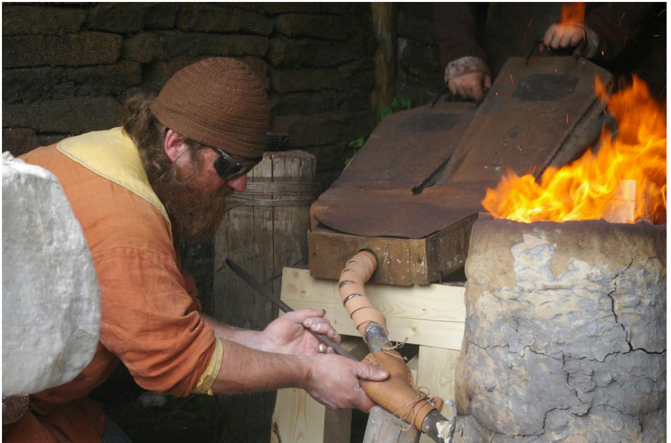
FIG 2. MARK PILGRIM CLEARING OBSTRUCTIONS DURING THE SMELT. NOTE THE MODERN SAFETY GLASSES - NO MATTER WHERE YOU ARE WORKING SOME THINGS SHOULD STILL BE USED. METAL TAPE WAS USED TO CONNECT THE BELLOWS AND THE TUYERE. NORMALLY THIS WOULD HAVE BEEN A LEATHER TUBE BUT THE SHORT TIME BETWEEN THE ARRIVAL DATE AND THE REQUIRED SMELT DATE DID NOT ALLOW FOR THE MANUFACTURE OF A CUSTOM PIECE ON SITE. (PHOTO: KELLY PROBYN-SMITH)
