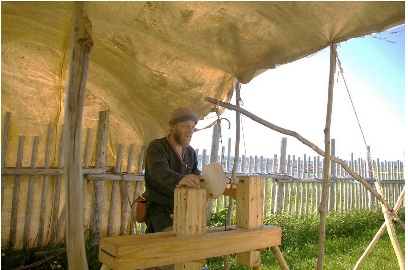
FIG 4. MARCUS BURNHAM PREPARING TO CONTINUE TURNING THE OUTSIDE OF A BOWL AFTER RE-ALIGNING THE LATHE. (PHOTO: KELLY PROBYN-SMITH)
