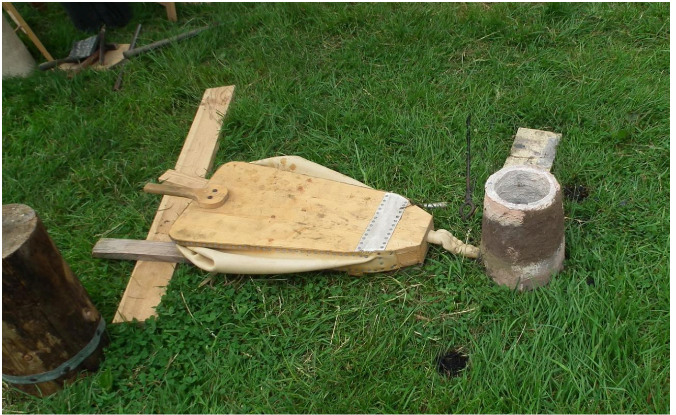
FIG 3. ROMAN BELLOWS AND FURNACE BUILT BY THOMAS LEIMBACH
