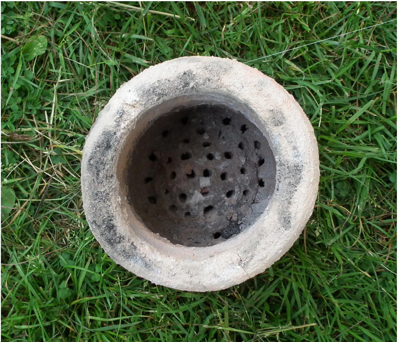
FIG 4. VIEW OF THOMAS LEIMBACH'S FURNACE FROM THE TOP, SHOW THE PERFORATED PLATFORM
