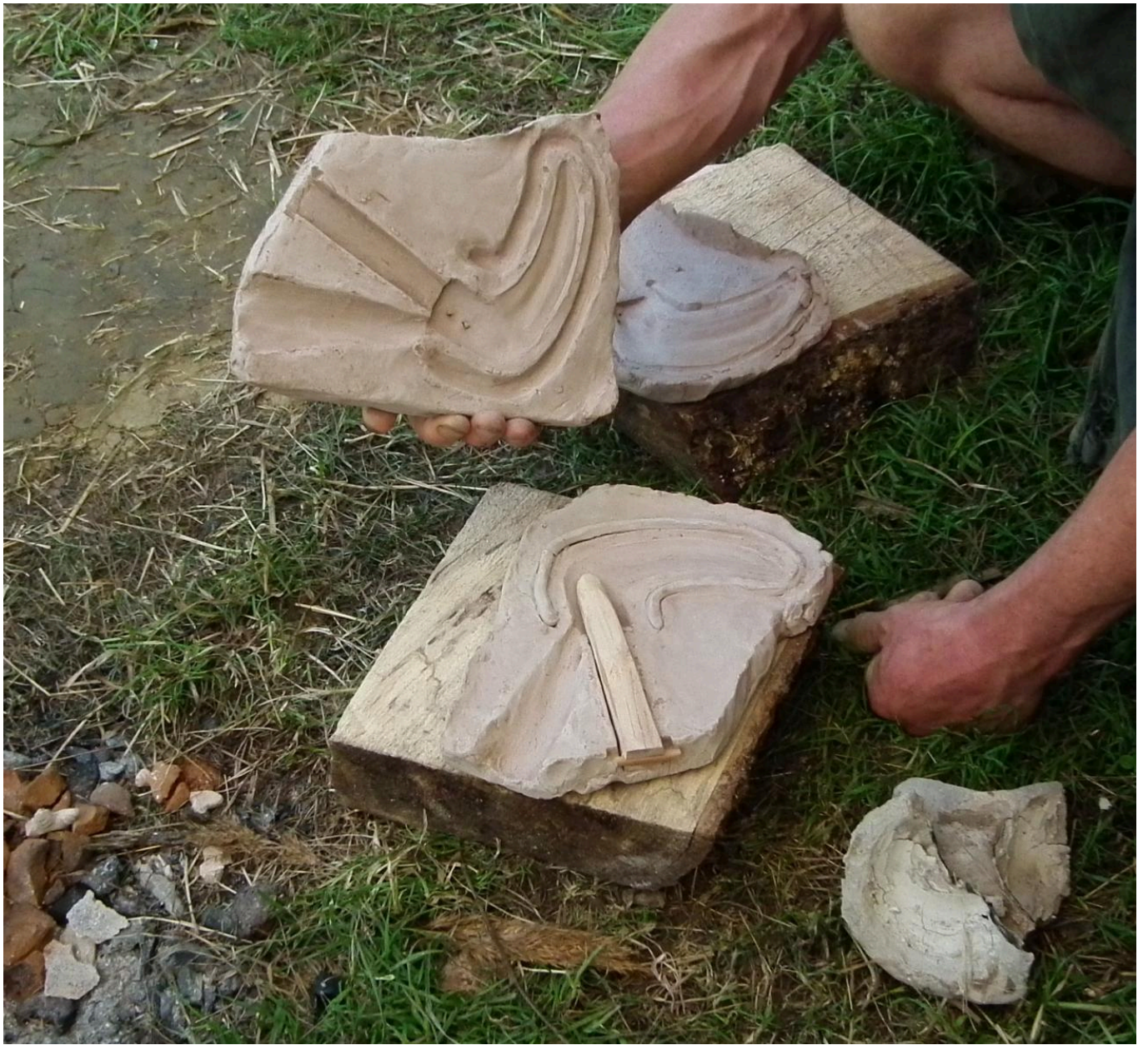
FIG 6. CLAY MOULD FOR A SICKLE WITH WOODEN CORE BY MARK VYVYAN-PENNEY
