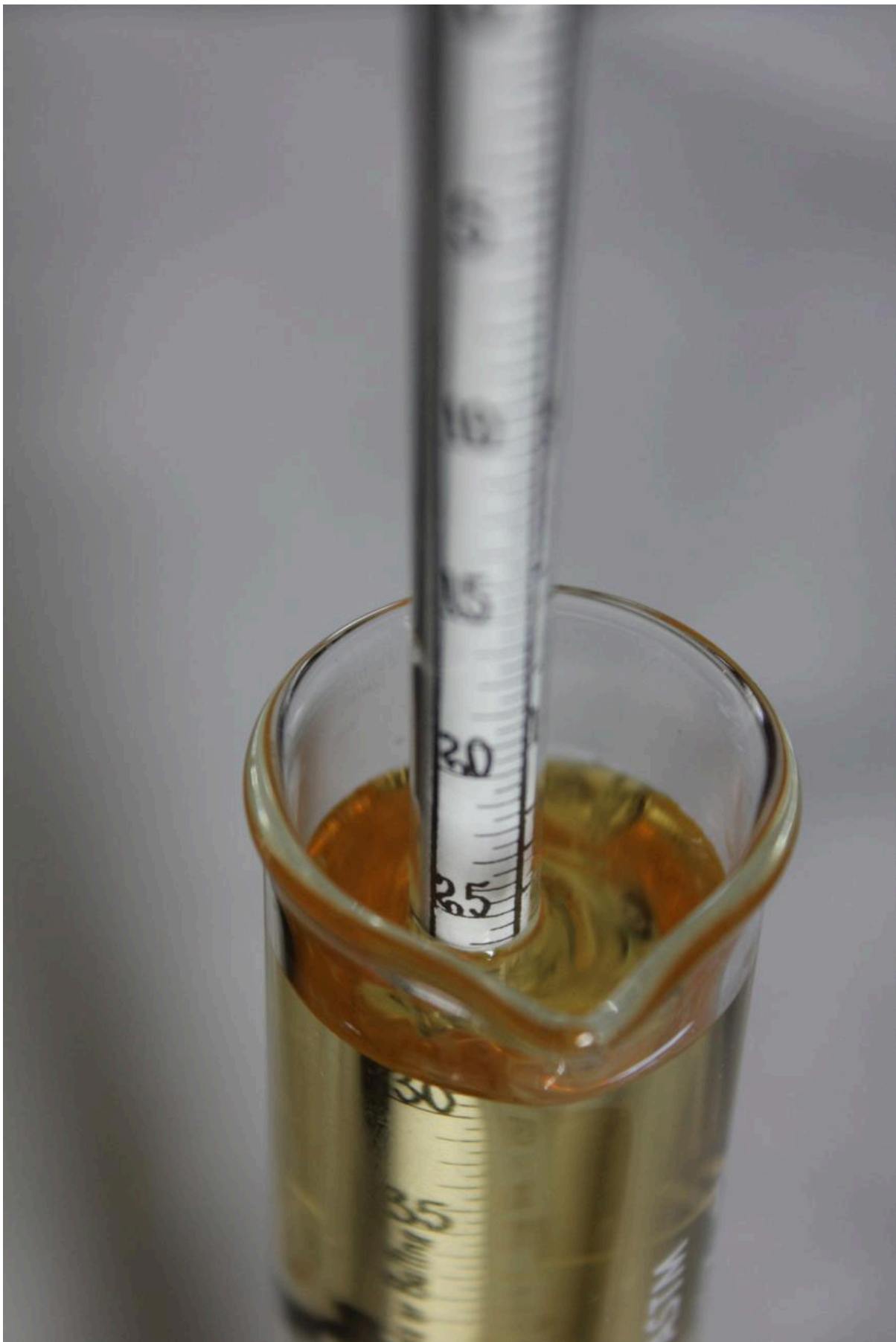
FIG 11. A HYDROMETER WAS USED TO DETERMINE SUGAR AND ALCOHOL CONTENT. ONE READING WAS TAKEN PRIOR TO FERMENTATION AND ONE AFTER; THE DIFFERENCE INDICATES THE ALCOHOL CONTENT.
