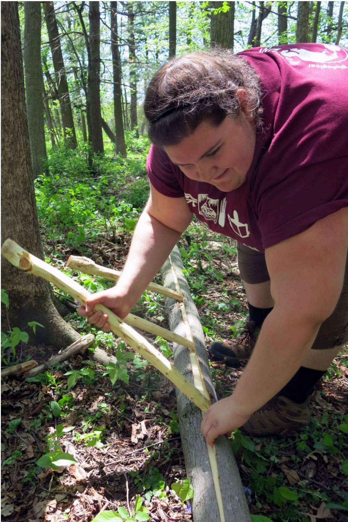
FIG 1. MAUREN FOLK USES HOMEMADE WOODEN BARKING SPUDS TO SEPARATE THE INNER AND OUTER BARK FROM ONE FELLED BASSWOOD TREE.
