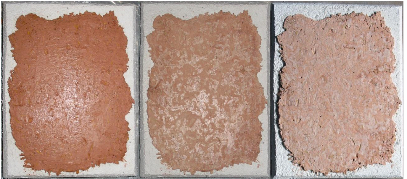
FIG 16. 22314 BRYSSBAERT 3: ALTERATIONS DURING THE DRYING OF BASE LAYER 2.
