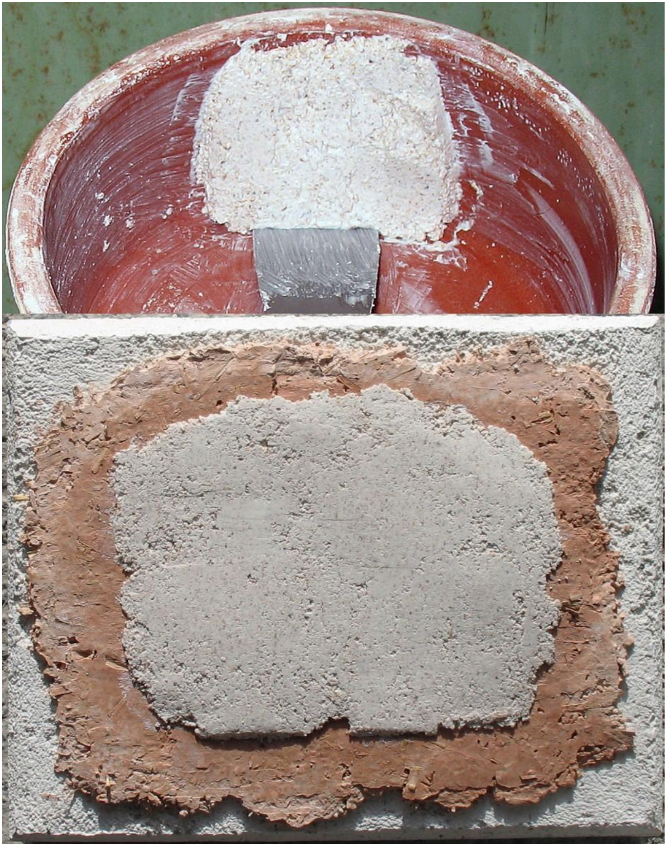
FIG 17. 22314 BRYSSBAERT 3: MIXTURE AND TESTING LAYER OF SEASHELLS AND LIME-PLASTER.
