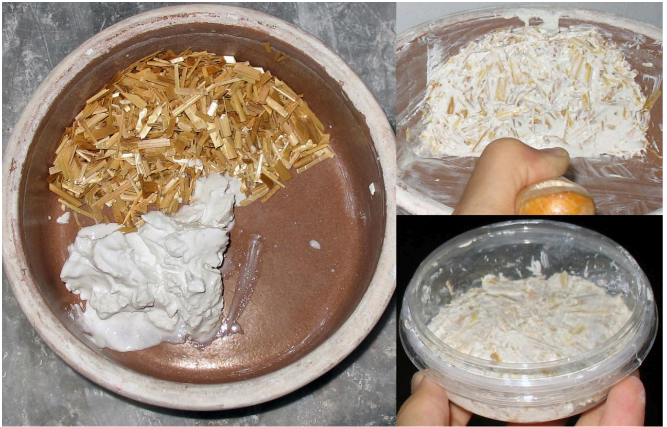
FIG 12. 16314 PALMETTE FLOWER: THE FRESH MIXTURE OF THE STRAW AND PLASTER.
