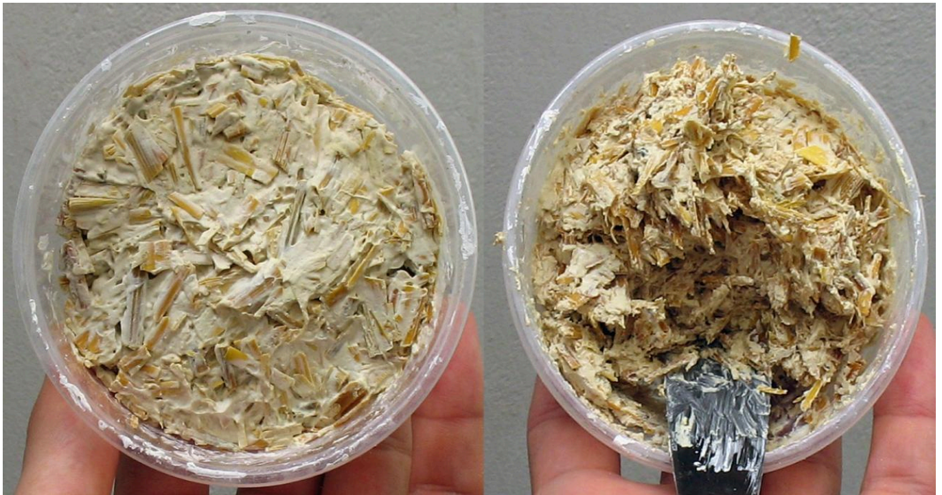
FIG 13. 16314 PALMETTE FLOWER: OPENING THE MIXTURE OF THE STRAW AND PLASTER AFTER 3 DAYS.
