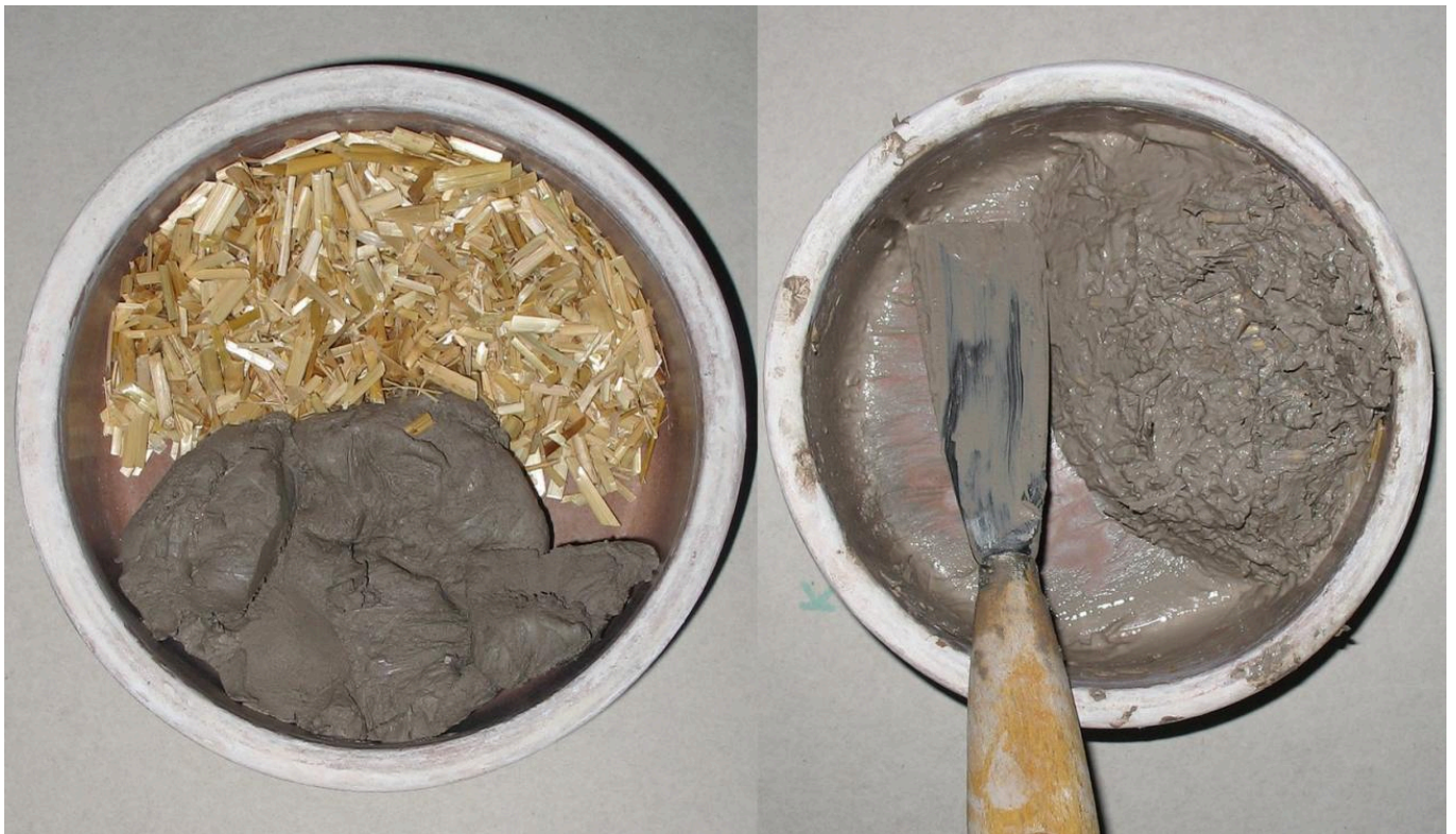
FIG 4. 25214 BRYLSBAERT 1: THE MIXTURE OF THE CLAY PLASTER.
