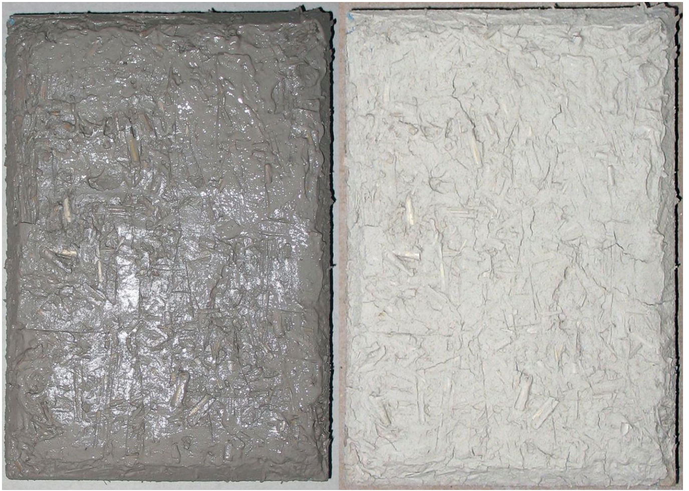
FIG 5. 25214 BRYLSBAERT 1: WET AND DRY CLAY PLASTER LAYER.
