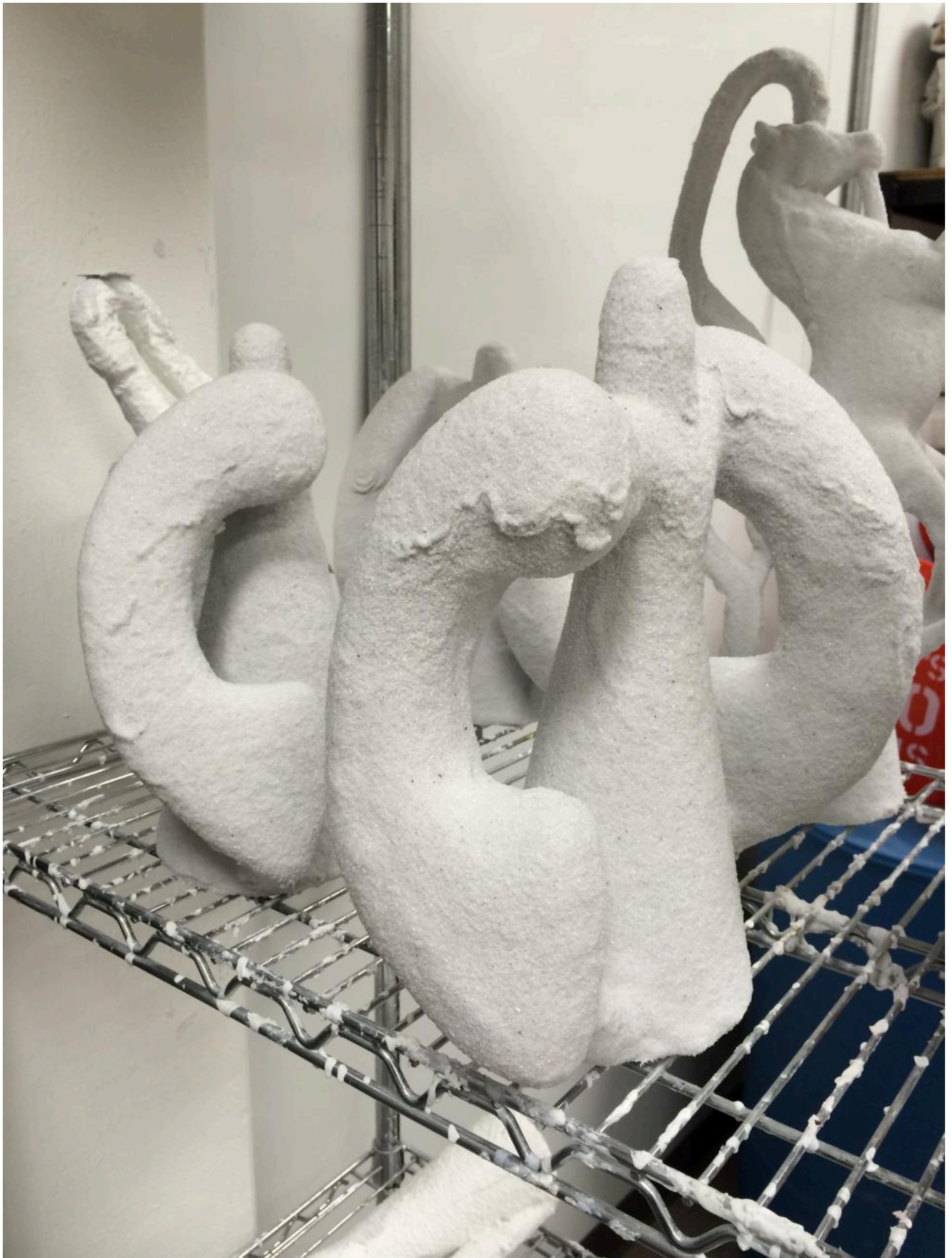
FIG 9. THE SULLRY HARDENS TO FORM THE SHELL FOR THE LOST WAX PROCESS.
