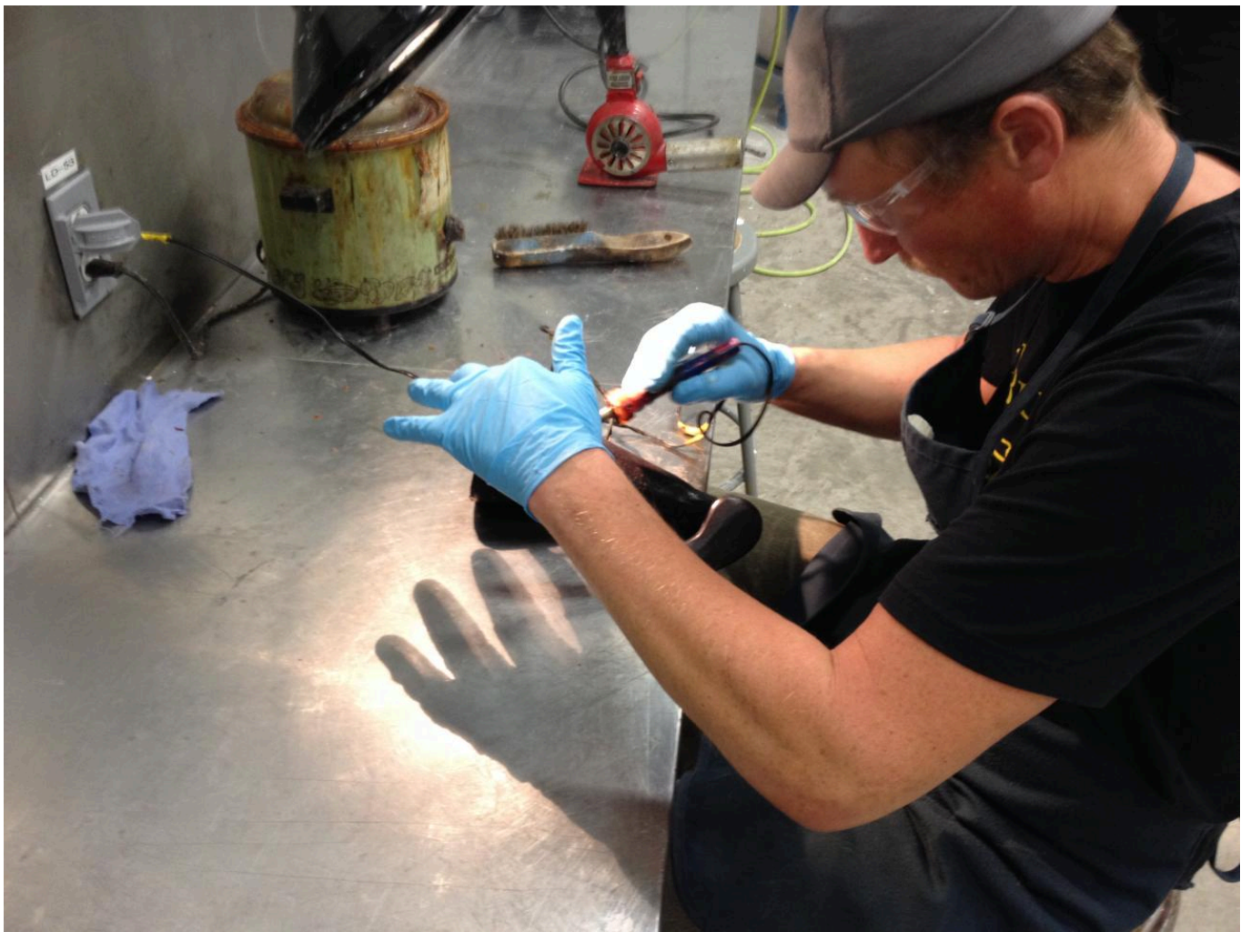
FIG 8. WILL CANNING MAKING THE WAX SPRUCES TO CREATE THE MOULD.
