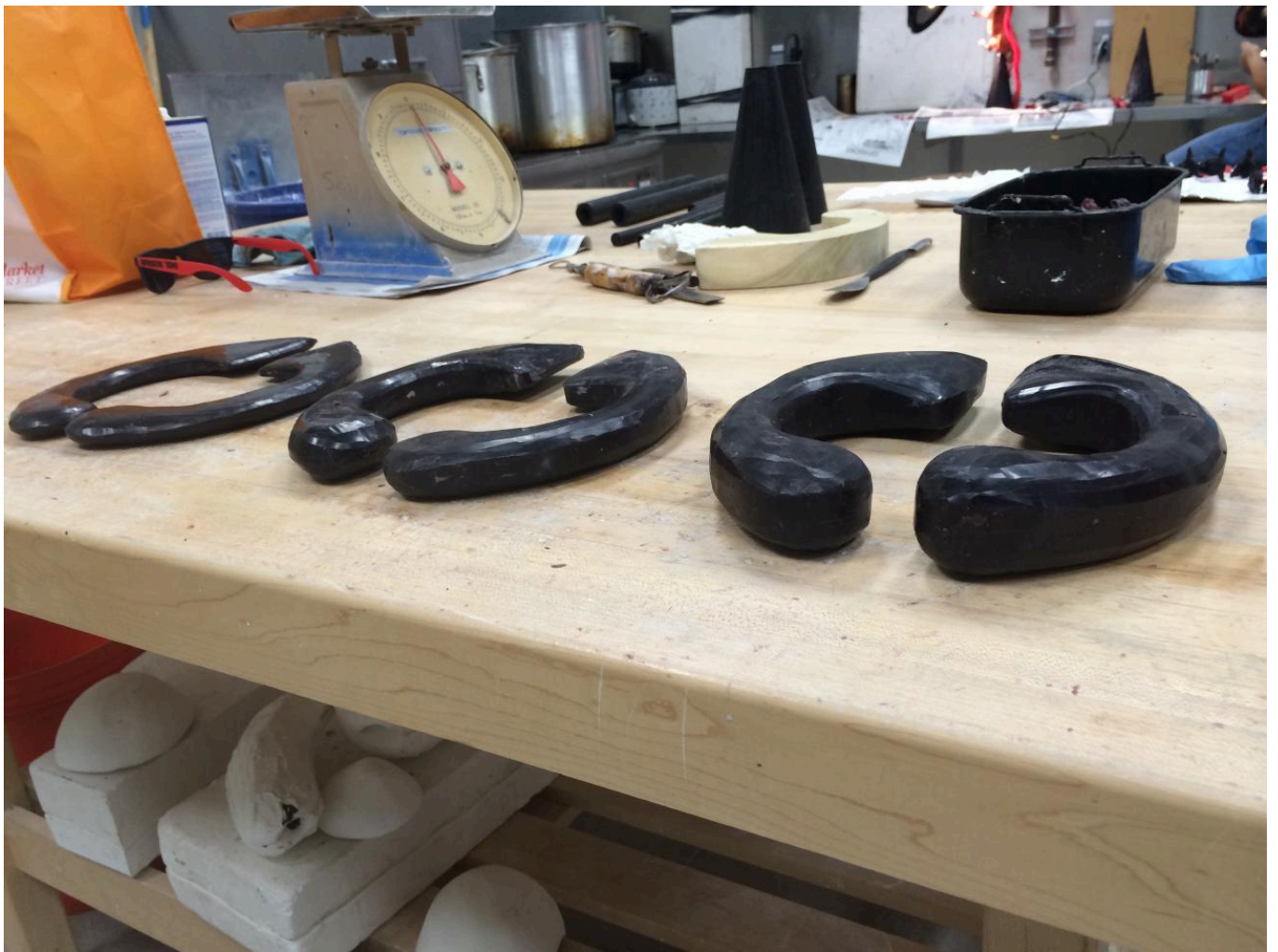
FIG 7. FINISHED WAX VERSIONS WHICH WERE PROPORTIONALLY THE SAME WEIGHT AS THE FINISHED BRONZE.
