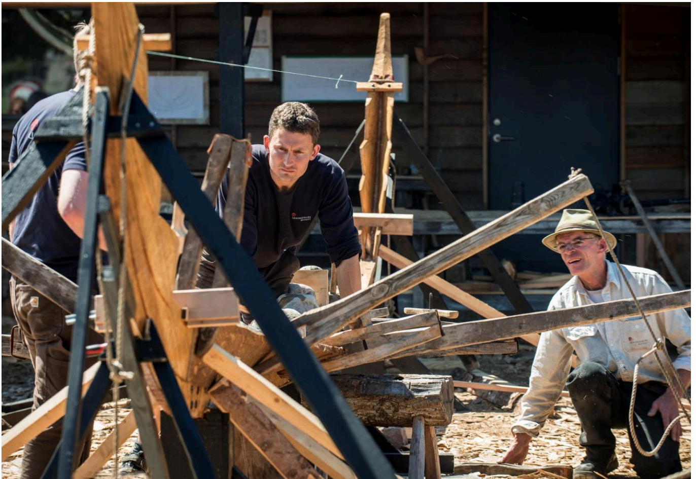
FIG 4. ONCE THE KEEL IS LAID AND THE STEMS ARE RAISED, THE PROCESS OF ADDING PLANKS TO THE HULL CAN BEGIN. EACH PLANK IS FIRST HEATED OVER THE FIRE TO MAKE IT PLIABLE AND THEN CLAMPED INTO PLACE ON
