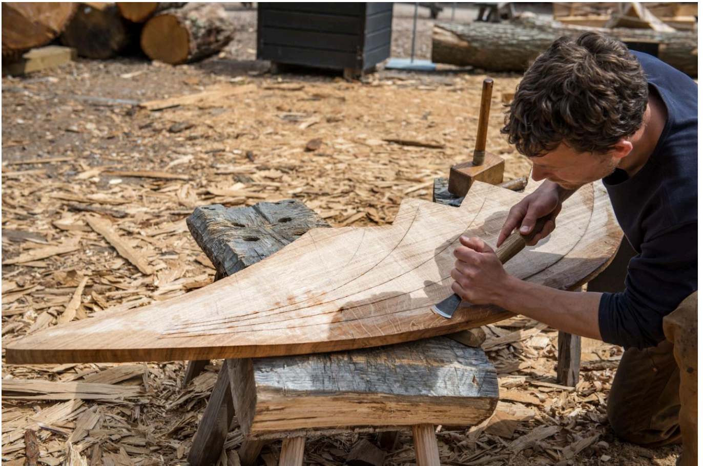
FIG 3. BOATBUILDER MARTIN RODEVAD DAEL SHAPES THE STEM FOR THE GISLINGE BOAT. PHOTO: WERNER KARRASCH: VIKING SHIP MUSEUM IN ROSKILDE
