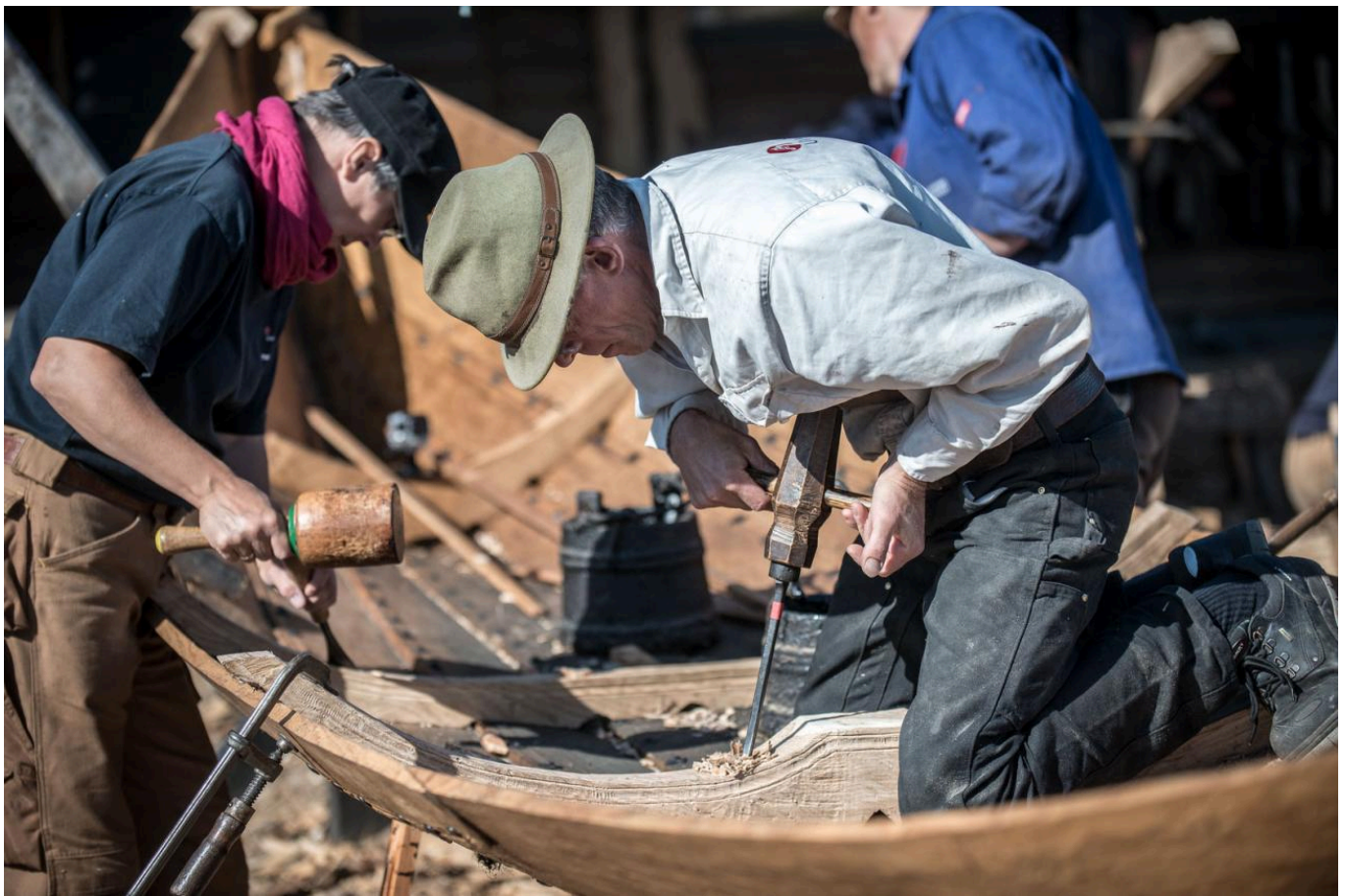
FIG 6. BOATBUILDER BIRGER ANDERSEN USES A SPOON AUGER TO DRILL THROUGH ONE OF THE FLOOR TIMBERS. THE FLOOR TIMBERS ARE SECURED IN POSITION USING TREENAILS MADE OF WILLOW. PHOTO: WERNER KARRASCH: VIKING SHIP MUSEUM IN ROSKILDE
