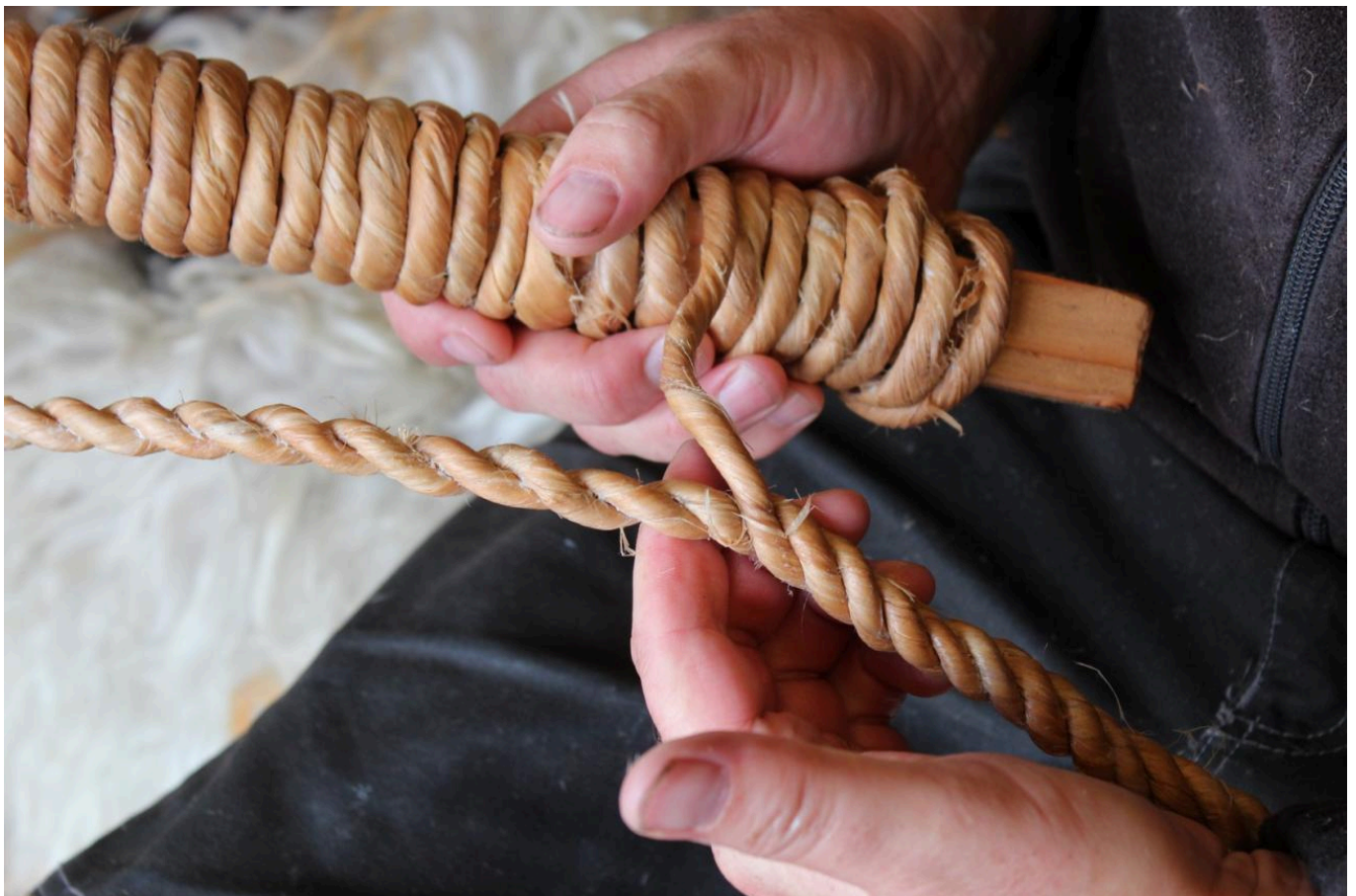
FIG 7. ROPEMAKER CARSTEN HVID LAYS LIME BAST ROPE FOR THE GISLINGE BOAT BY HAND. PHOTO: TRÍONA SØRENSEN: VIKING SHIP MUSEUM IN ROSKILDE.
