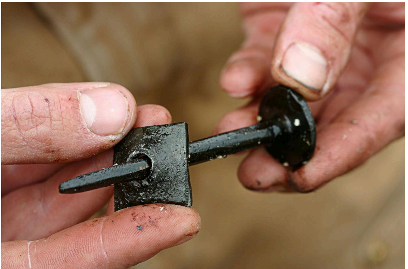
FIG 9. AN IRON RIVET AND ROVE. A SAMPLE OF THE RIVETS AND ROVES FOR THE GISLINGE BOAT WERE MADE FROM BOG IRON AND WILL BE MONITORED AS PART OF AN ON-GOING PROJECT TO SEE HOW THE MATERIAL BEHAVES WHEN USED IN A MARITIME CONTEXT. PHOTO: WERNER KARRASCH: VIKING SHIP MUSEUM IN ROSKILDE.
