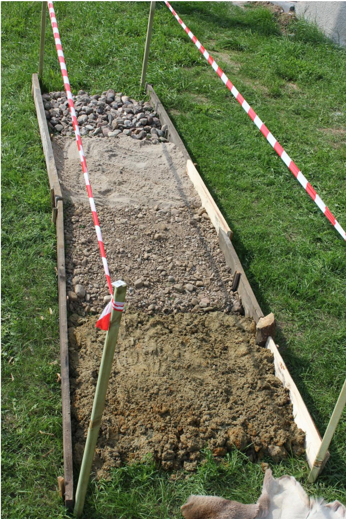
FIG 5. A PATH WITH SECTORS FILLED WITH SAND, GRAVEL, STONE, AND CLAY USED IN EXPERIMENTAL WORKS WITH TRAMPLING.
