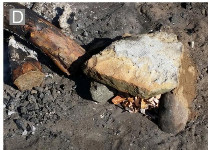
FIG 2. EXPERIMENTS WITH METHODS OF BIRCH TAR PRODUCTION WITHOUT THE USE OF CERAMICS. VARIOUS TYPES OF KILN STRUCTURES: A- CLOSED-HEARTH STONE KILNS LINED WITH SANDY CLAY DURING CONSTRUCTION; B - KILN MADE OF WATTLE COVERED WITH SILT; C - KILN MADE OF EMPTY GOOSE EGG SHELLS; D - OPEN-HEARTH STONE KILN.
