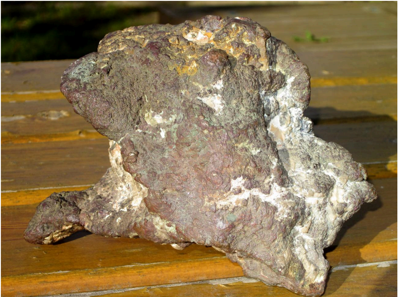
FIG 1. NATIVE COPPER (THE RED-BROWN PART) FROM ARIZONA. HEIGHT CA 12 CM. "ULF FORNHAMMAR"
