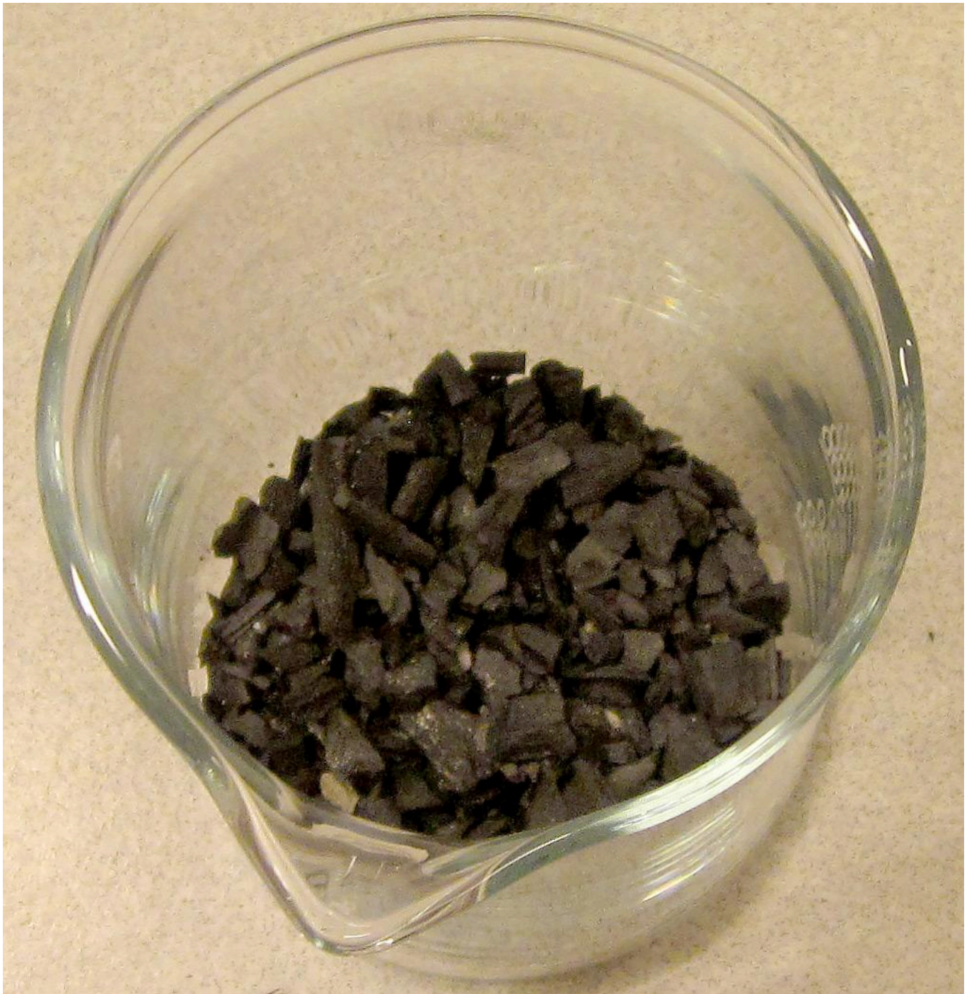
FIG 6. CRUSHED AND SIEVED CHARCOAL, WHICH IS A CARBONACEOUS FUEL. "ULF FORNHAMMAR"
