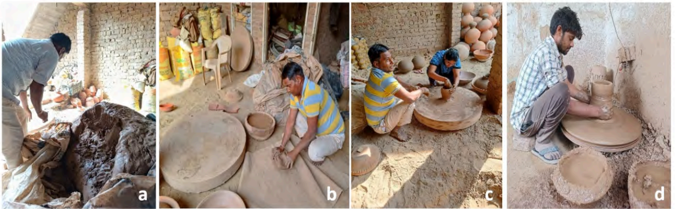
FIG 9-1. A. SOAKED/ LEVIGATED CLAY. B. KNEADING OF CLAY C. HAND MOTIONED WHEEL. D. ELECTRIC WHEEL. PHOTO BY GARIMA SINGH
