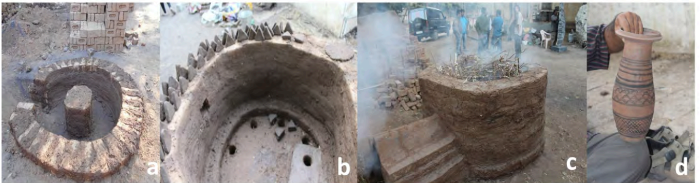
FIG 6. A. KILN SHAFT IN THE CENTRE WITH A ROOM TO PUT FUEL, B. UPPER PORTION TO PUT POTS, C. KILN AFTER FIRING, D. PAINTED POT. PHOTO BY GARIMA SINGH
