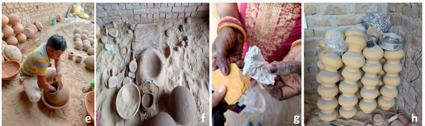
FIG 9-2. E. SHAPING OF JAR AFTER LEATHER HARD STATE. F. POTTERS TOOLS. G. YELLOW OCHRE AND WHITE MINERAL FOR COLOURING THE POTS H. COLOURED POTS KEPT IN A DARK SPACE TO AIR DRY. PHOTO BY GARIMA SINGH
