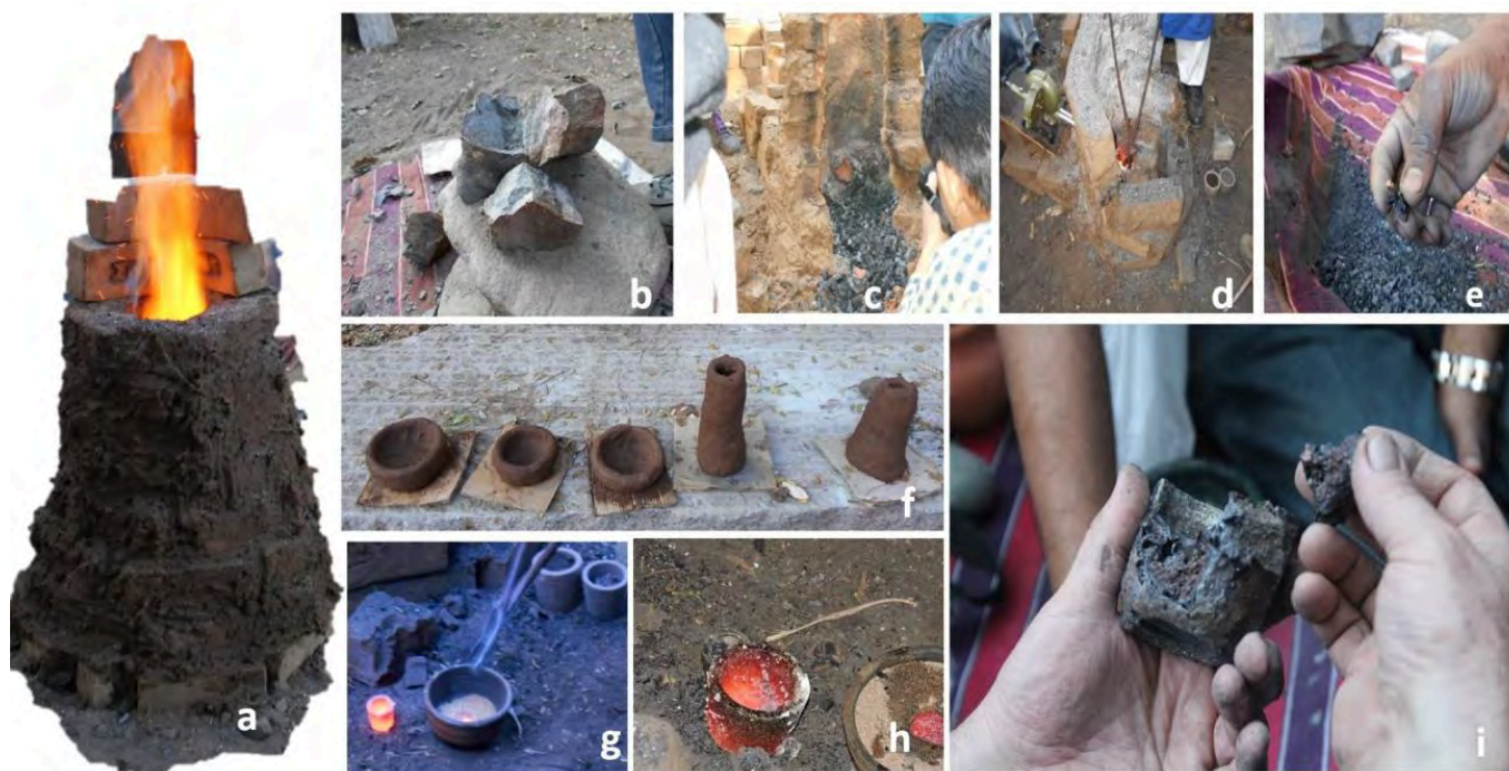
FIG 7. A COPPER SMELTING FURNACE. B. COPPER ORE C. DISMANTLED FURNACE FOR COLLECTING MOLTEN METAL FROM ORE. D. COLLECTION OF METALLIC FRAGMENTS FROM CRUCIBLE. E. OXIDIZED ORE F. CLAY TYERS FOR FURNACE G. POURED MOLTEN COPPER OVER SAND. H. CRUCIBLES. I. BROKEN CRUCIBLE AFTER MELTING THE COPPER. PHOTO BY GARIMA SINGH
