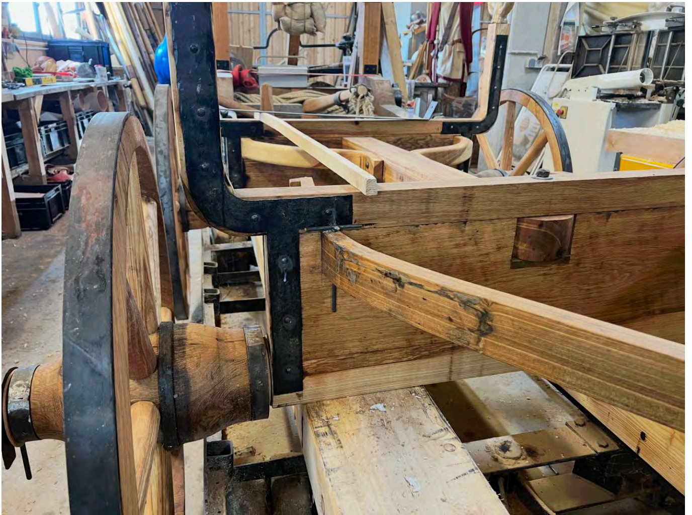
FIG 25. VIEW ON AXLE BOLSTERS AND SWING HANGERS IN THE BACKGROUND. PHOTO BY B. DREYER
