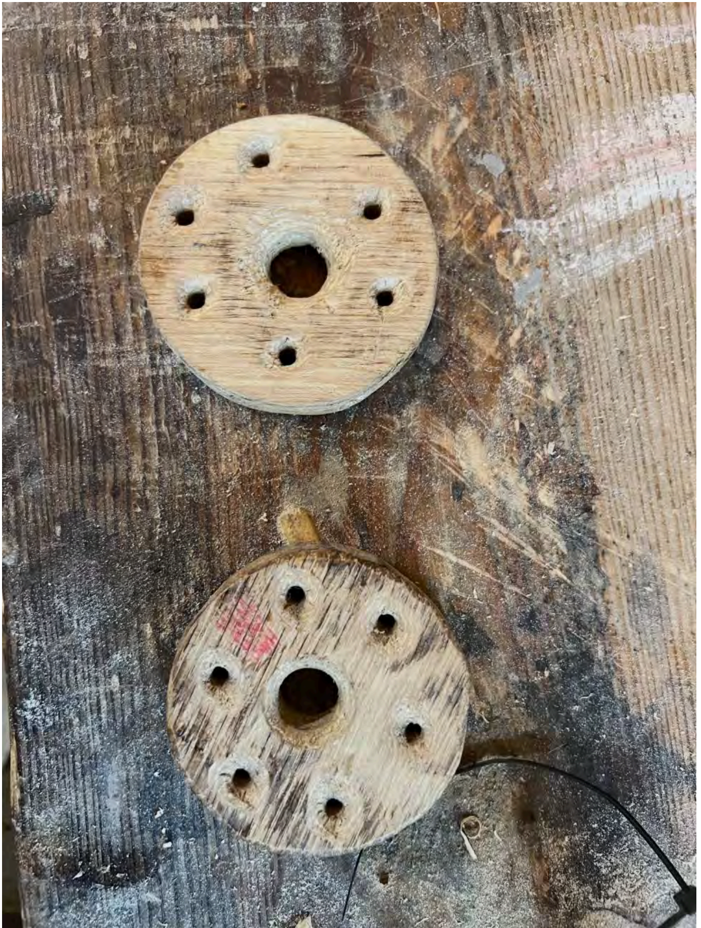
FIG 16. PIERCED LETTERS FOR MAKING BOW-STRINGS. PHOTO BY B. DREYER
