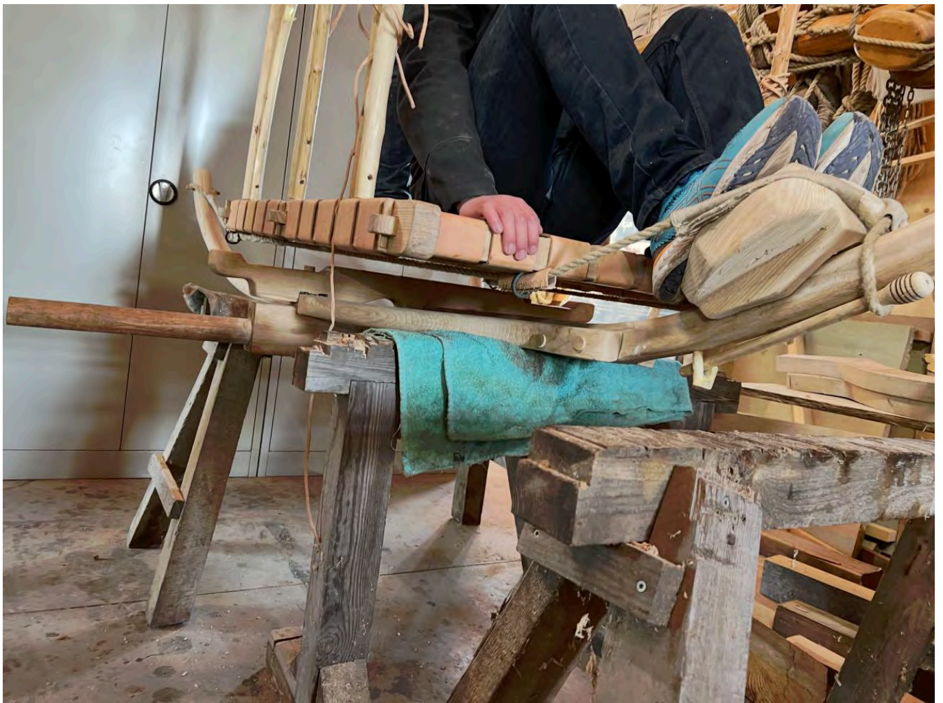
FIG 22. SUSPENSION BY ROPES LED FROM THE BENT FORKS AT THE REAR RIGHT AND LEFT TO THE FRONT IN THE TRIANGLE AND UNDER THE BOX BODY THROUGH EYELETS AND STRETCHED OVER THE FOOTBOARD AT THE FRONT WITH TOGGLES. THIS LIGHTWEIGHT VEHICLE IS HIGHLY MANOEUVRABLE, WEIGHING BARELY 100 KG AND YET ROBUST. PHOTO BY. B. DREYER
