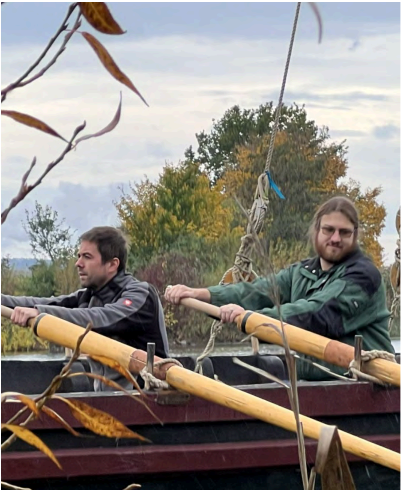
FIG 5B. THE DIFFERENT BELT SUSPENSIONS ARE SHOWN HERE, THE HISTORICAL SUSPENSION (EVIDENCED BY ABRASION AT THE THOLEPINS OF THE BOAT WRACKS) WITH A ROPE RING (STROPE). PHOTO BY B. DREYER
