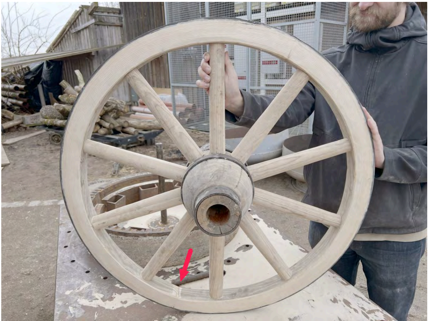
FIG 20. THE RIM OUT OF ONE (SEE ARROW FOR THE SOLE SEAM) BEAM OF ASH-WOOD. PHOTO BY B. DREYER
