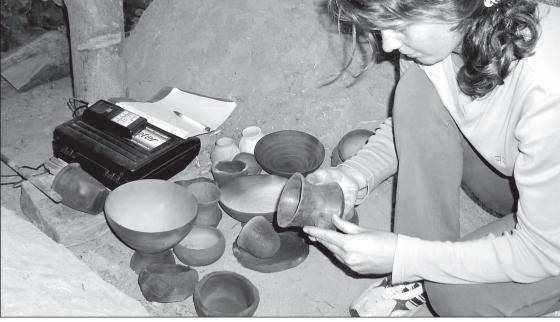
**Experimental firing of pottery** with measurment the development of temperatures.
