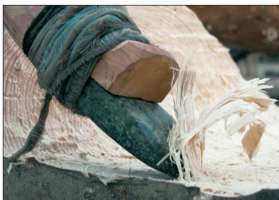
■ Fig. 6 Detail: the sharp blade of the adze removes a chip of wood.
