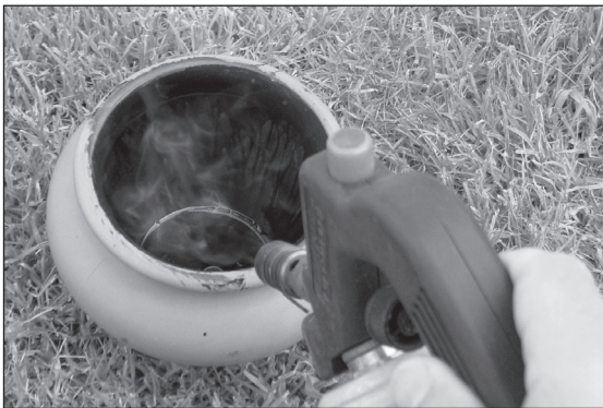
■ Fig. 2 Hardening the tar with a gas flame
